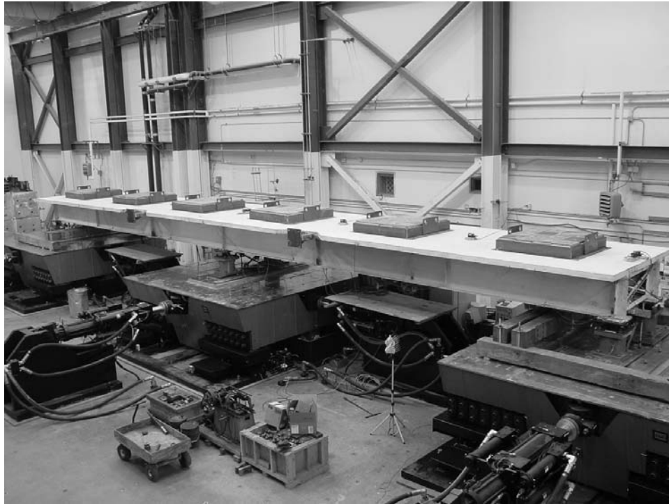
FIGURE 2-27 Bridge Model attached to three 50 ton shake tables
