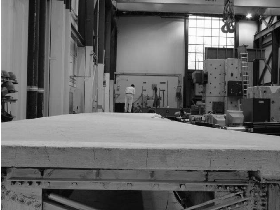
FIGURE 3-1 RSHXB - Deformed deck slab of bridge model during transverse loading
