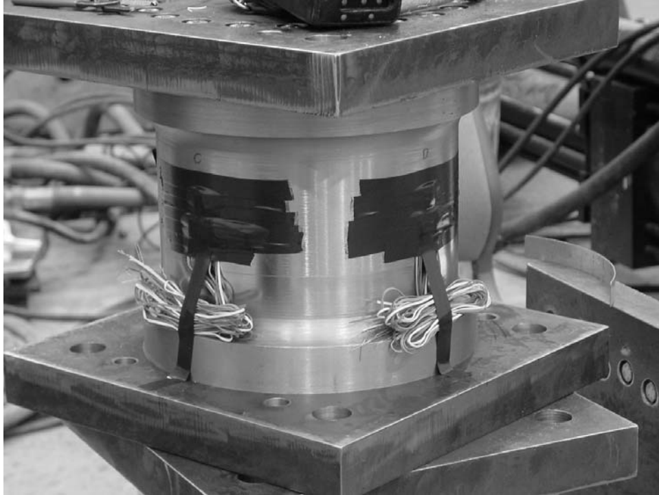
FIGURE 2-37 Multi-axial load cell during construction
