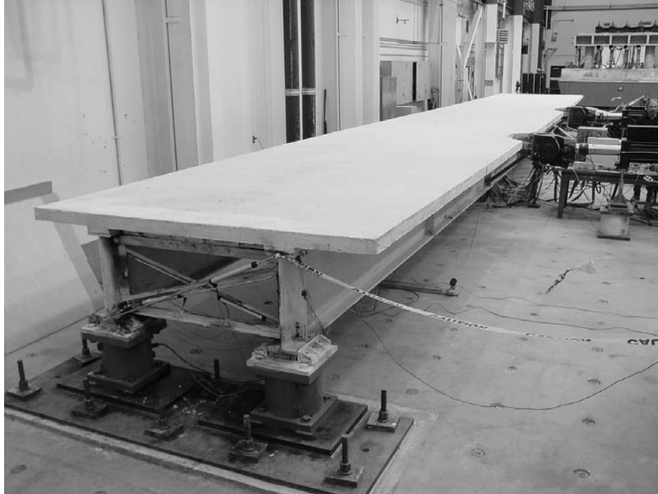
FIGURE 2-5 Steel slab-on-girder bridge superstructure model.
