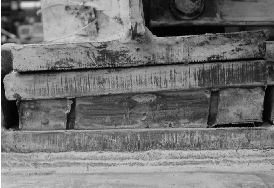
FIGURE 7-2 Deformation of elastomeric bearing with rotation applied to bearing in bridge model
