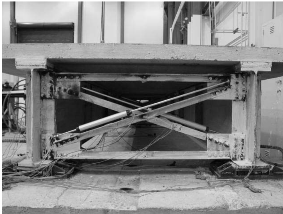
FIGURE 2-9 “Heavy” end cross frames at the north end in the bridge model
