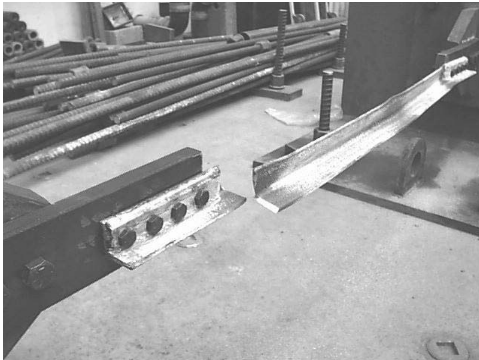
FIGURE 3-7 Failure of single angle with reinforced bolted connection
