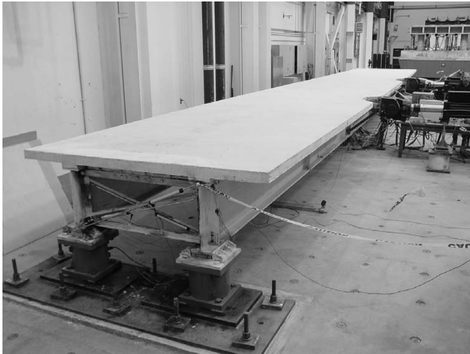
FIGURE 2-1 Slab-on-girder bridge superstructure model
