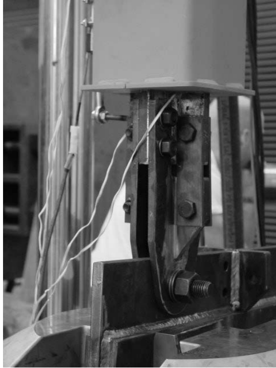
FIGURE 3-35 Pin ended connection in unbonded brace component experiment
