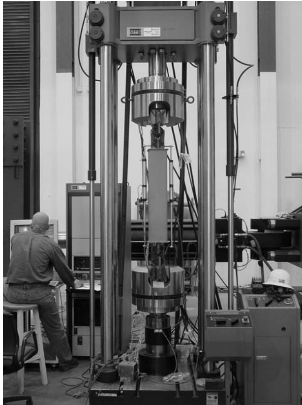
FIGURE 3-34 Experimental setup for testing of unbonded braces
