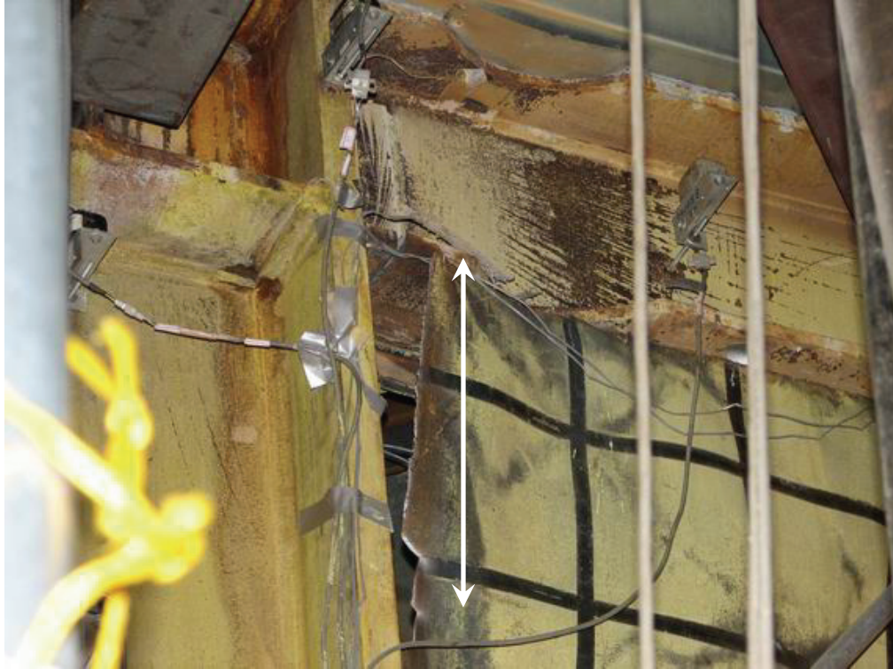
FIGURE 4-53 Plate Tear at the Upper North Corner of the First-Story Infill Panel (During Cycle 10)
