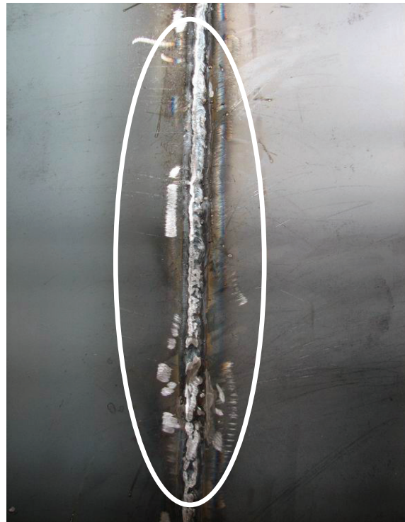
(b) Final Continuous Welds
