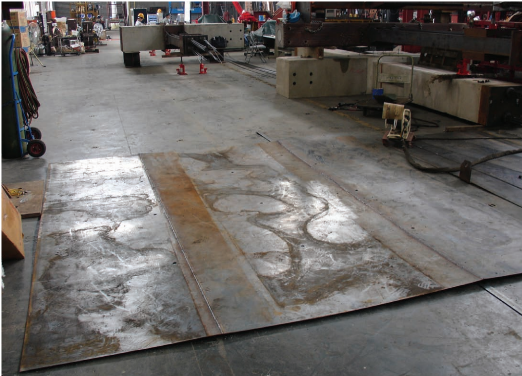
FIGURE 3-10 Assembled Infill Panels (Photo Courtesy of C.H.Lin and K.C.Tsai, NCREE)
