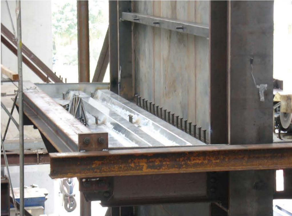
FIGURE 3-13 Corrugated Steel Deck (Photo Courtesy of C.H.Lin and K.C.Tsai, NCREE)
