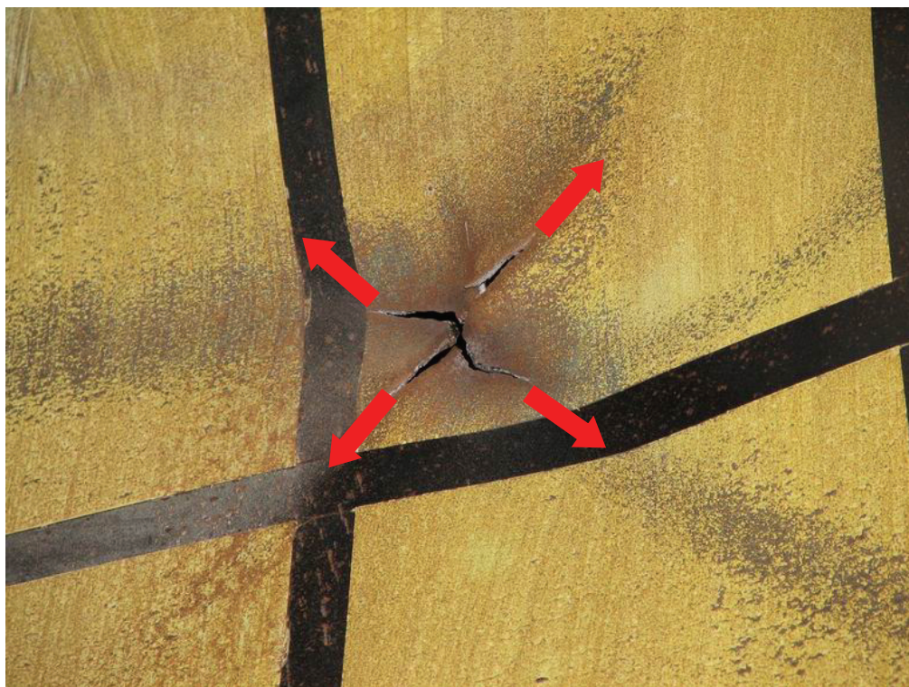
(b) Detail of Panel Tear
