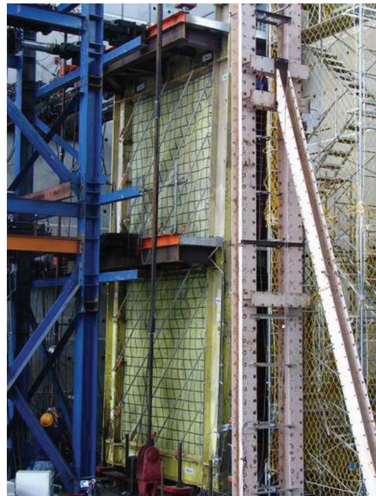
(b) Tension Field in the Specimen
