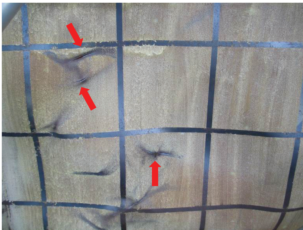
FIGURE 4-16 Initiation of the Panel Tear
