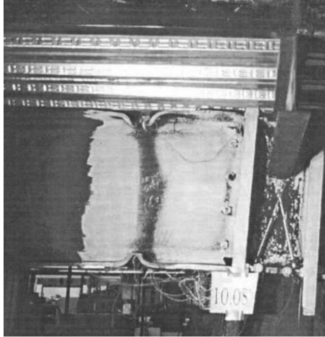
(h) Web of the beam with RBS in moment frame (from Jones et al. 2002)
