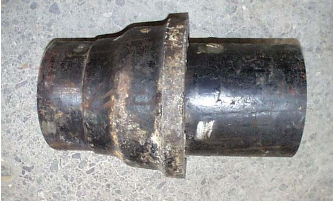
Figure 5.5 Cast Iron Pipe with Bell-and-Spigot Lead Caulked Joint (after American Lifelines Alliance, 2005)
