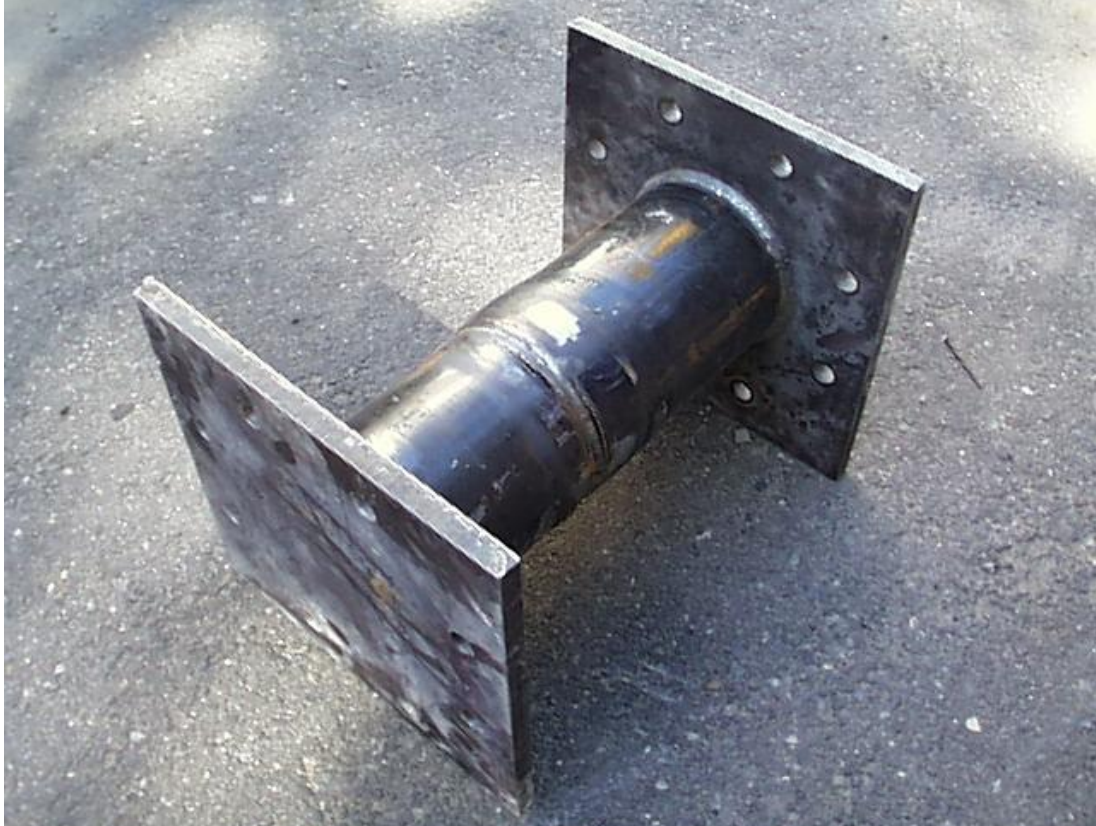
Figure 5.13 Steel Pipe with Welded Slip Joint
