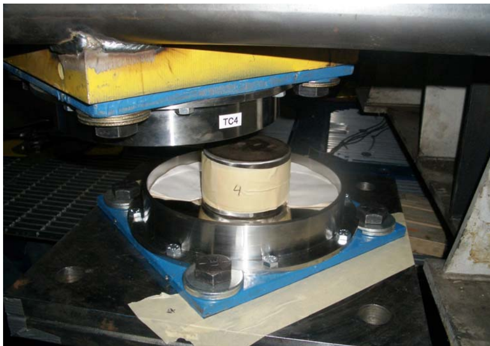
FIGURE 4-25 Taped Slider and Template Used to Align and Center the Slider
