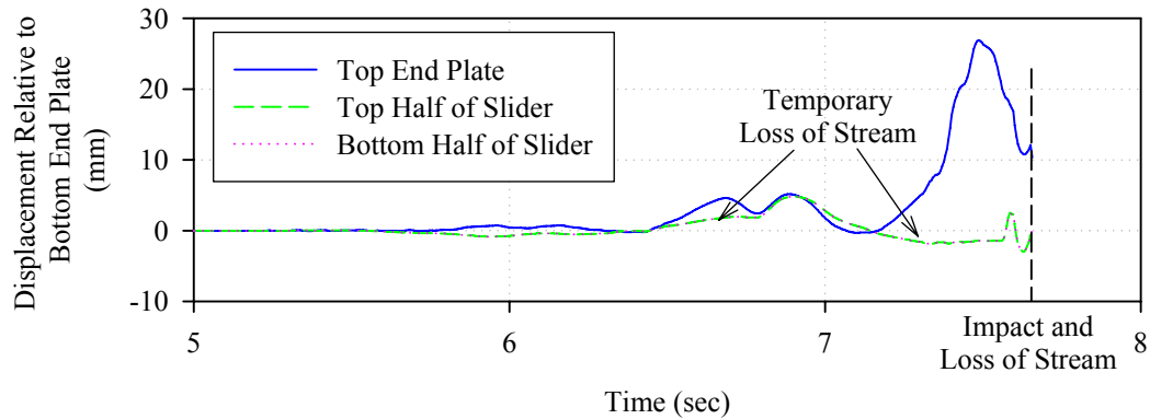
FIGURE 5-25 History of Vertical Displacements Relative to the Bottom Concave Plate of Various Parts of the SE Bearing in the 200% Tridirectional El Centro Test
