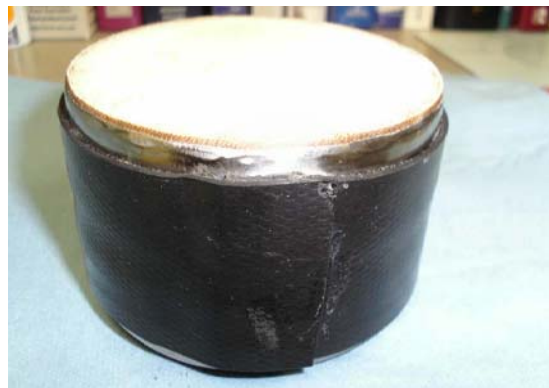
FIGURE 5-31 Triple FP Bearing Slider Assembly with Prototype Rubber Boot Attached to the Slide Plates
