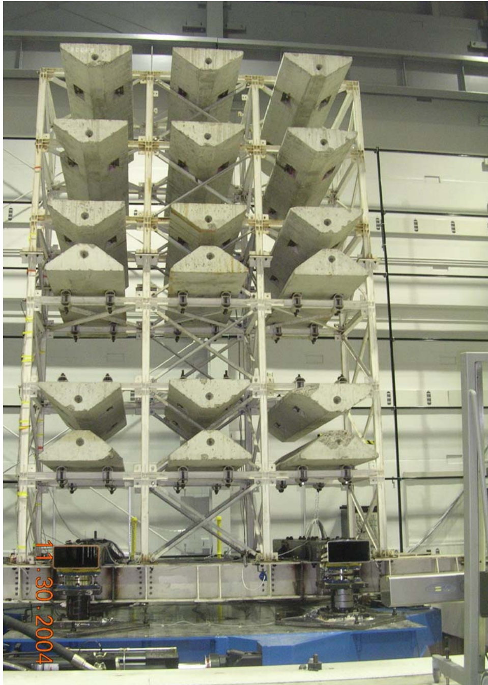
FIGURE 4-1 Photograph of Six-Story Isolated Model in the Structural Engineering and Earthquake Simulation Laboratory at UB (Braced Frame Configuration)
