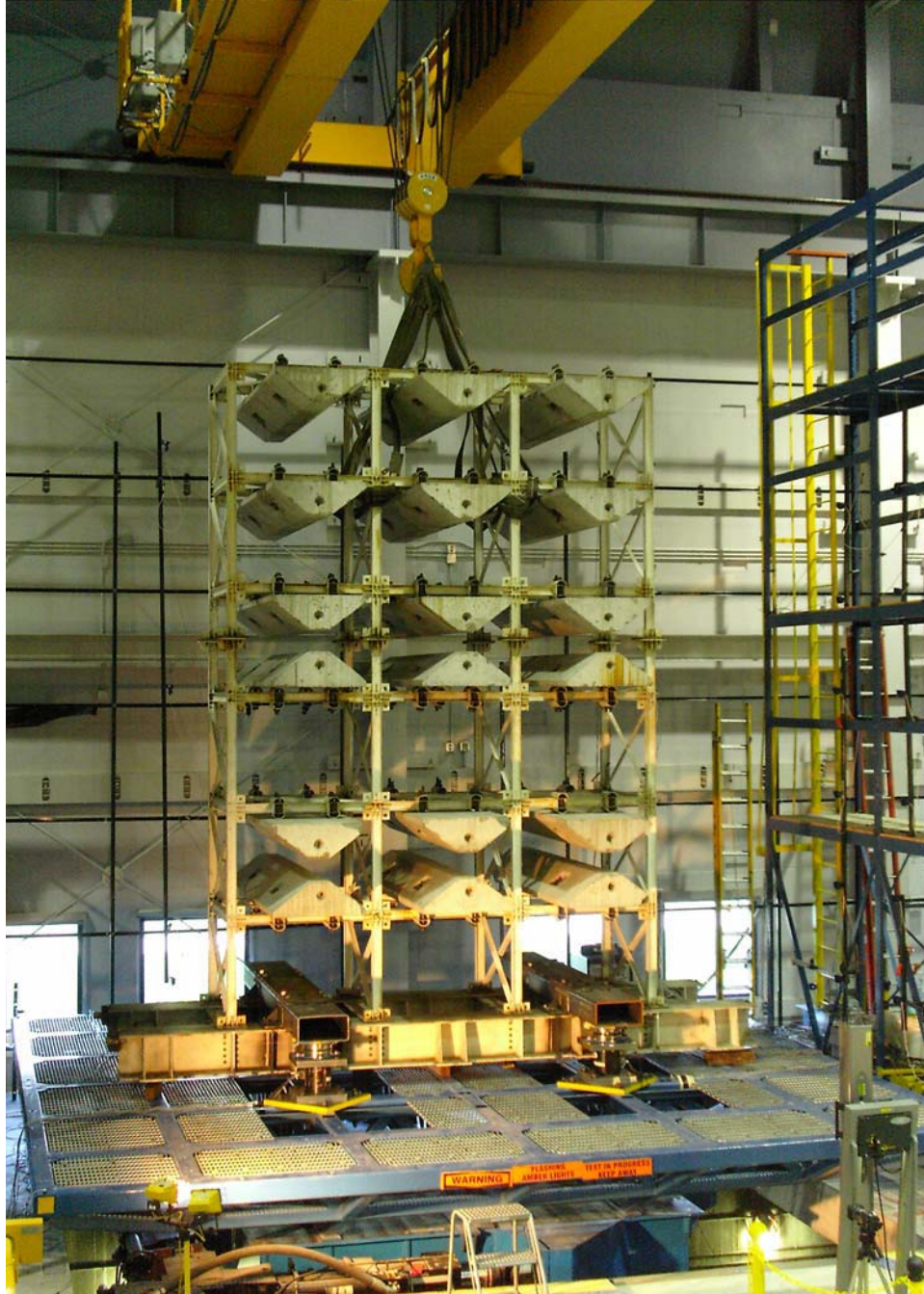
FIGURE 4-2 Photograph of Six-Story Isolated Model in the Structural Engineering and Earthquake Simulation Laboratory at UB (Moment Frame Configuration)
