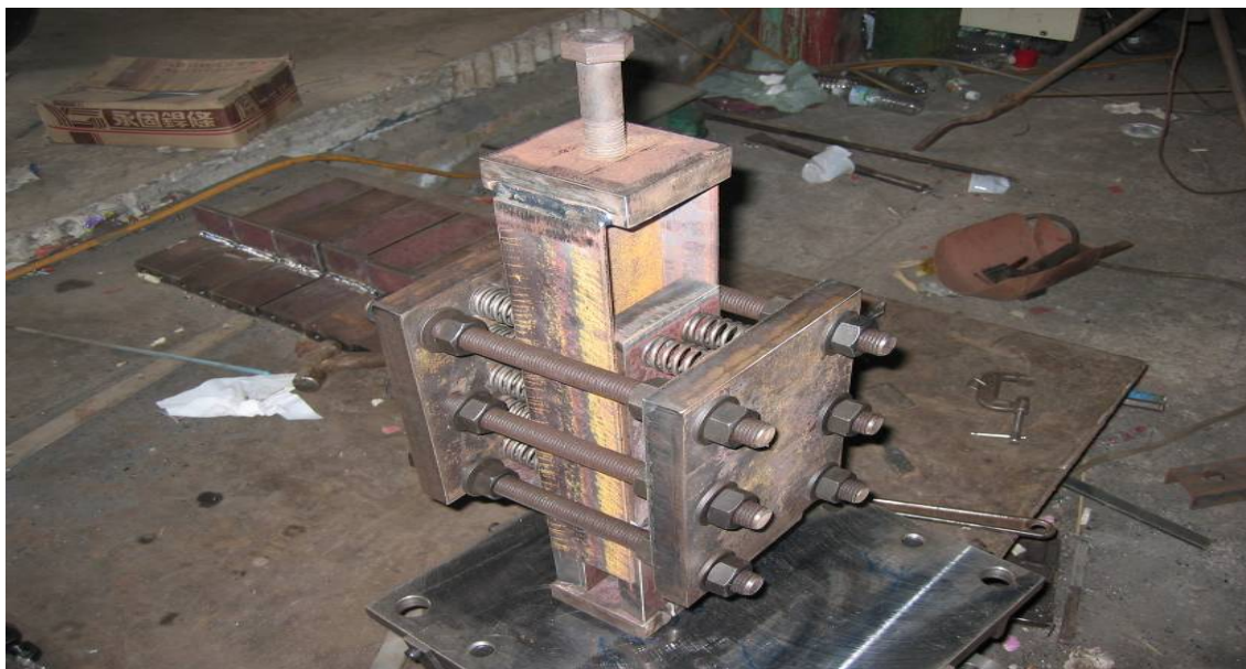
Figure 1-9 Damper used in NCREE test
