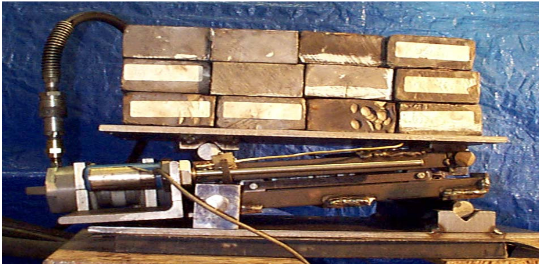
Figure 4-1 Experiment set up for clean track test (TN)
