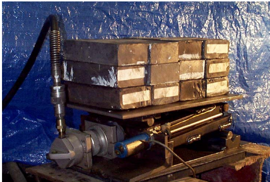
Figure 2-2 The first experiment set up for the roller friction test
