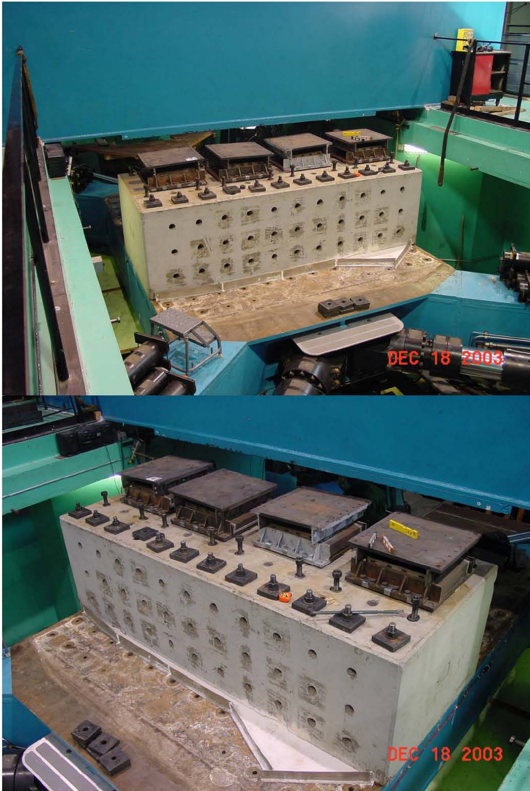
Figure 4-2 Test table and bearings
