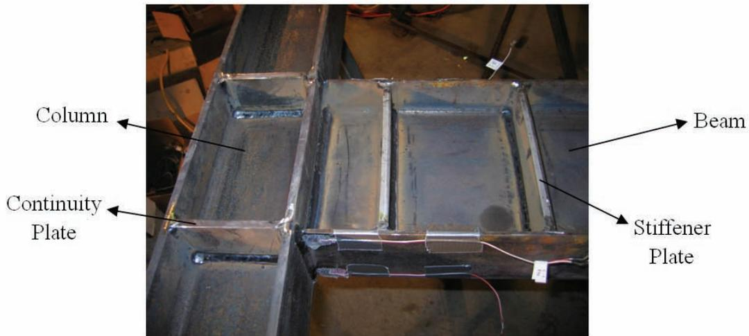
Figure 6-3 Beam-Column Connection in SMRF Mode
