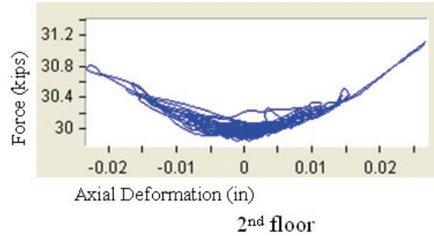
**Figure 7-43 Force vs. Deformation of PT Strands
