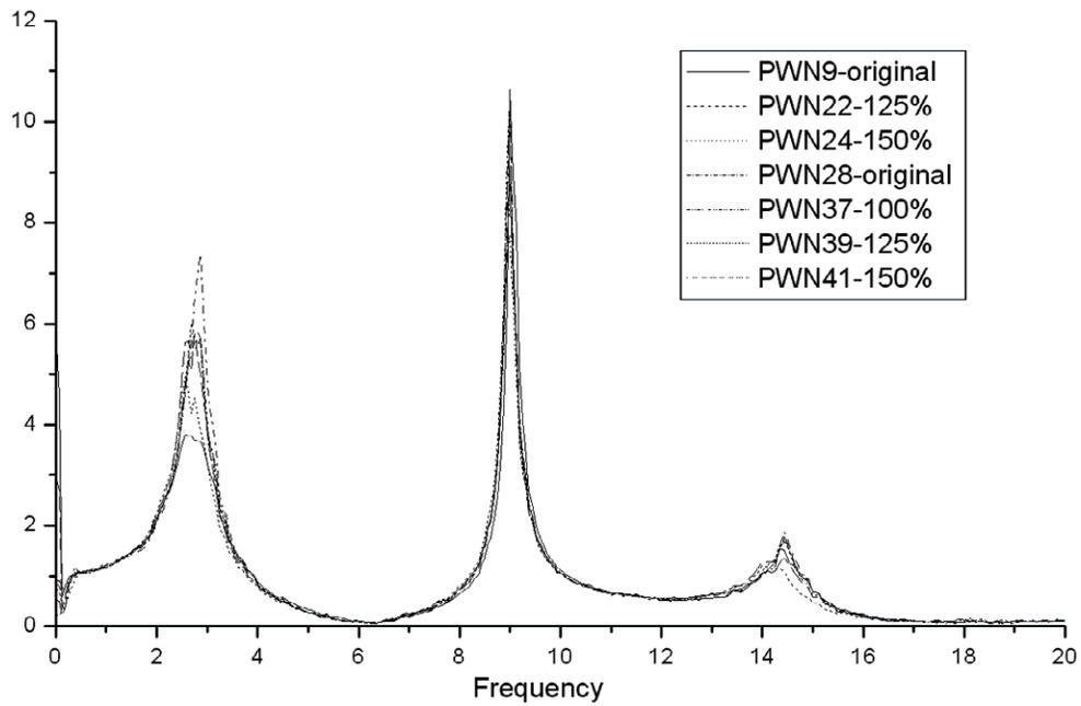
Figure 7-9 Transfer Functions for White Noise Tests, SCPT Model
