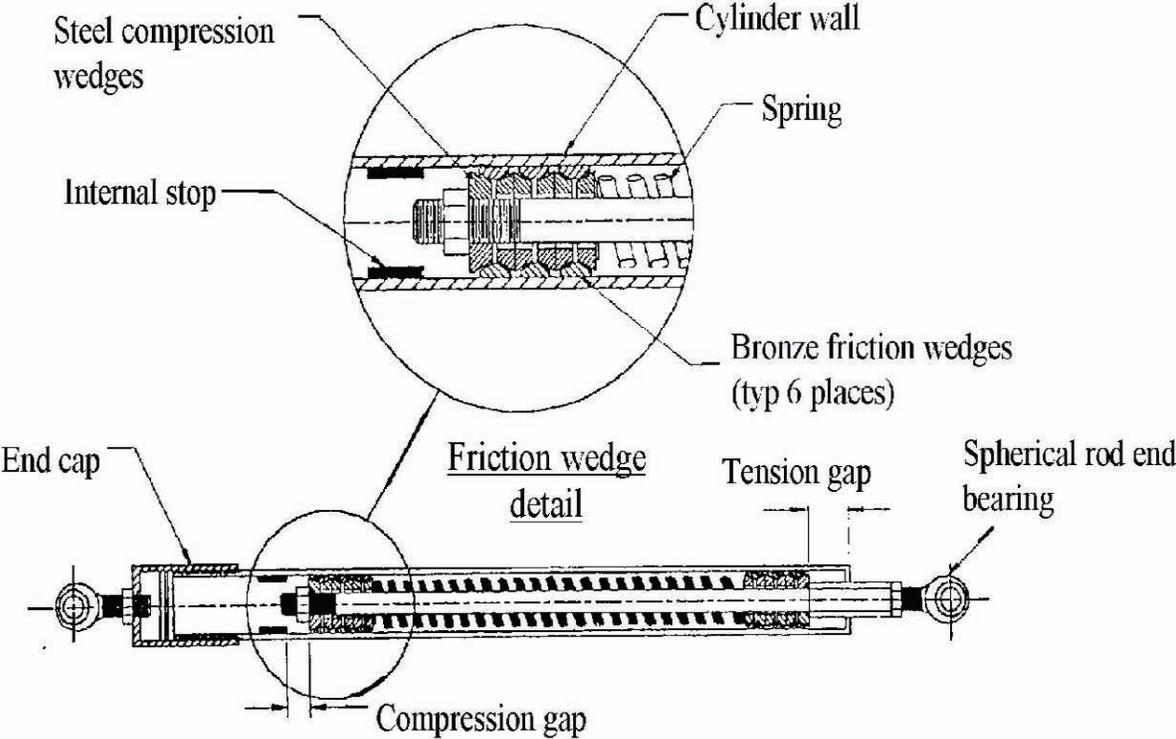
Figure 2-4 Internal View of Energy Dissipating Restraint (Nims et al. 1993)
