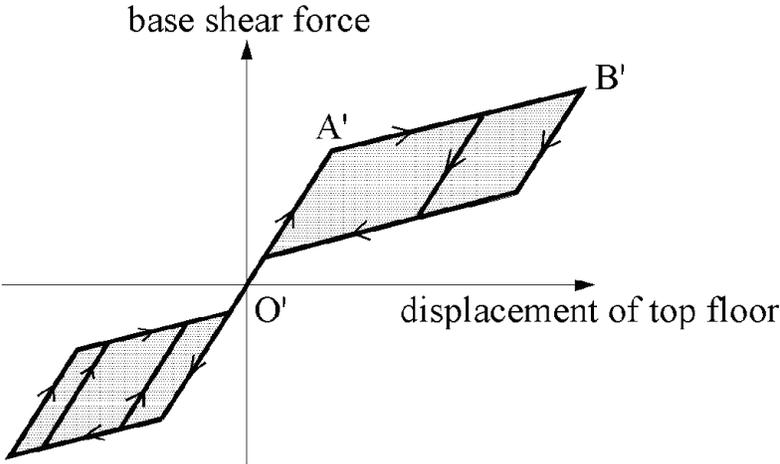
Figure 1-6 Ideal Seismic Response of Self-Centering Systems (SCS)
