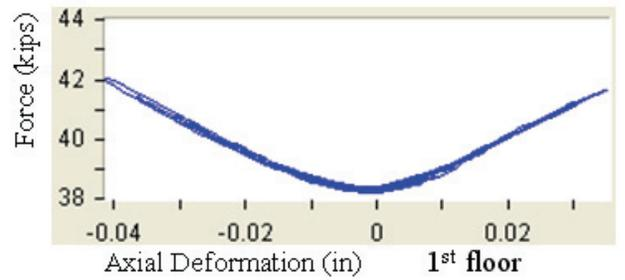
Figure 7-54 Force vs. Deformation of PT Strands For Test PER23 (-150%)
