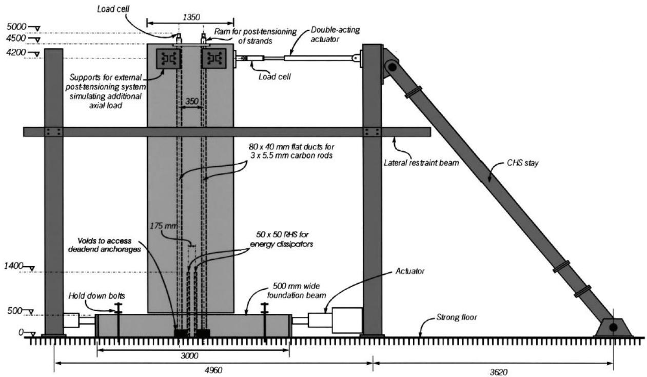
Figure 2-10 Loading Frame and Rocking Wall (Holden et al. 2003)
