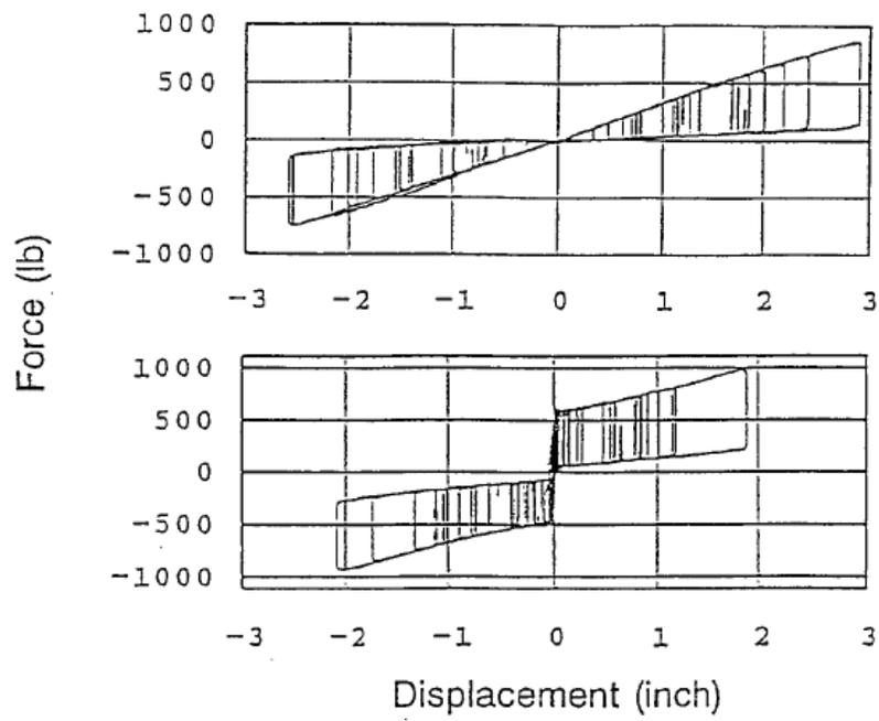
Figure 2-5 Various Self-Centering Hysteresis Loops Provided by the EDR Device (Aiken et al. 1993)
