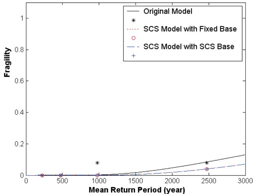
Figure 4-14 Fragility in Collapse Prevention with 5% transient drift criteria
