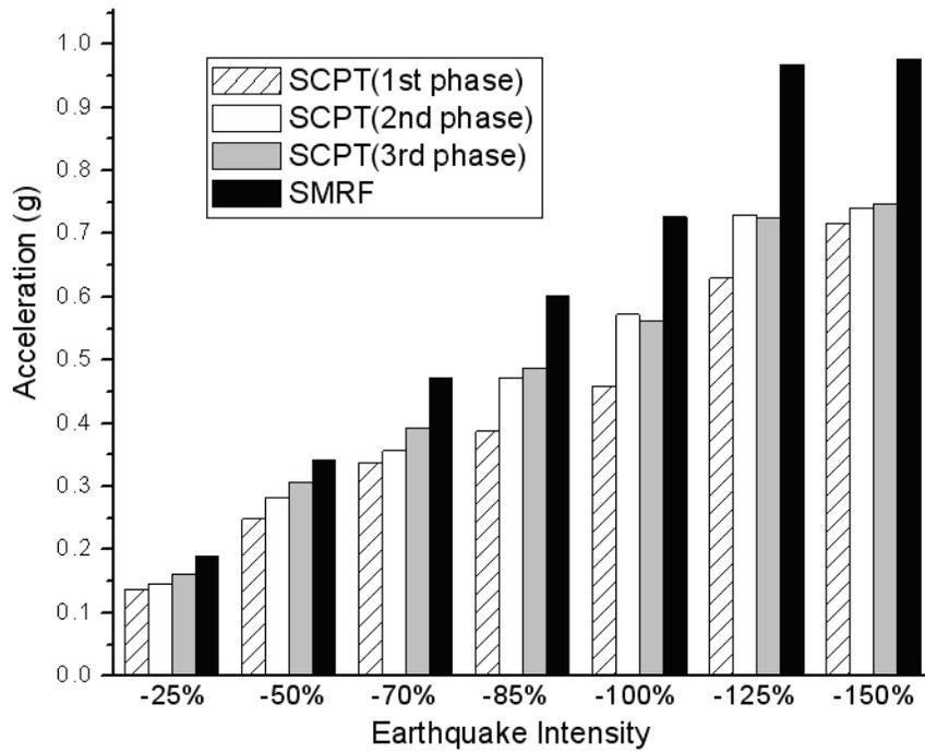
Figure 7-25 Peak Acceleration Response of the 2<sup>nd</sup> floor for the SCPT and SMRF Models in Negative Direction Seismic Tests
