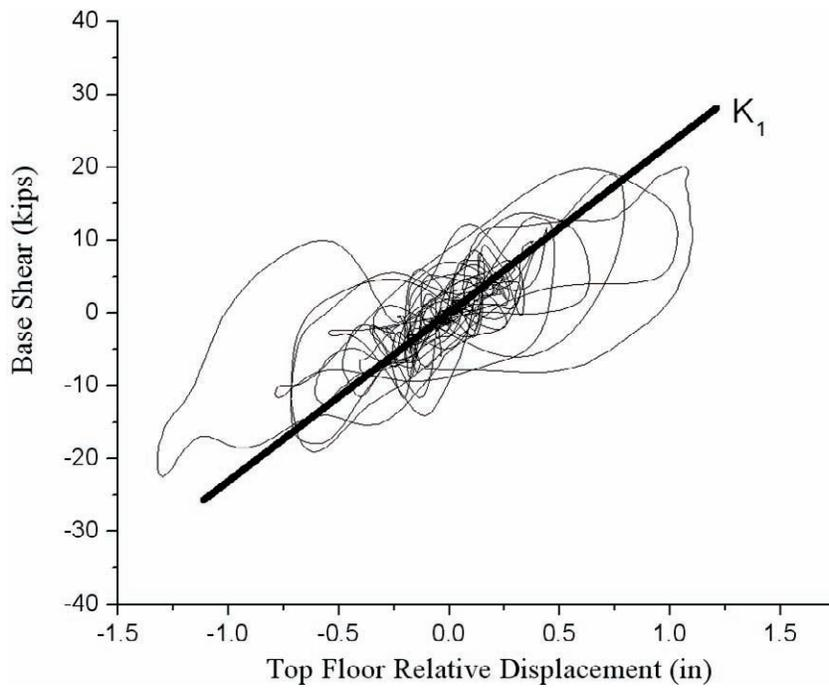
Figure 7-33 Hysteresis for the SCPT Model in test PE6A (1<sup>st</sup> phase, +125% intensity)
