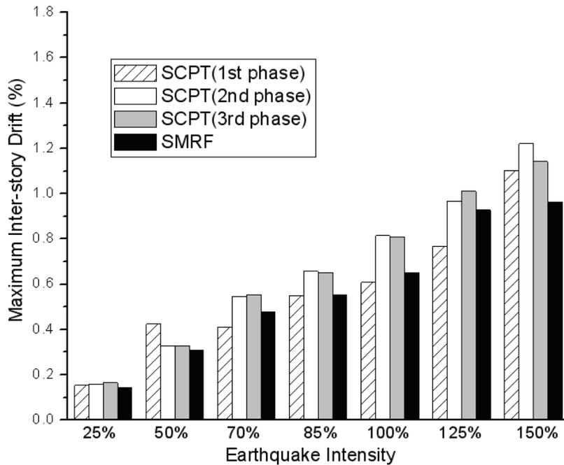
Figure 7-29 Maximum Inter-story Drift of the 3<sup>rd</sup> floor for the SCPT and SMRF Models in Positive Direction Seismic Tests
