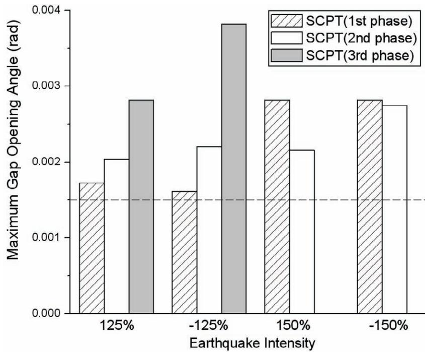
Figure 7-42 Gap Opening of the beam-column joint in 2<sup>nd</sup> floor for the SCPT Model
