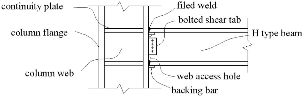
Figure 1-2 Recent (post-1970) Type of Welded SMRF Connection
