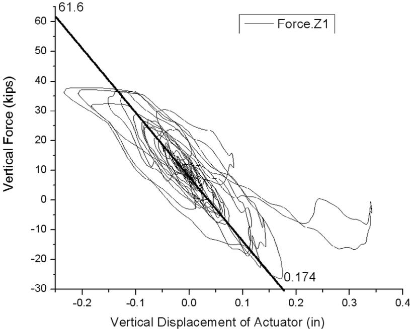
Figure 8-3 Force vs. Displacement of the vertical actuator Z1
