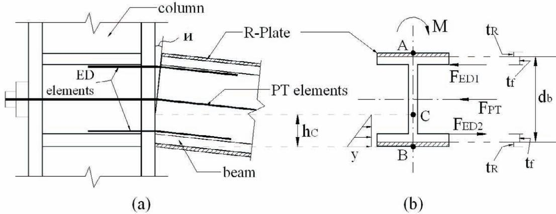
Figure 4-16 SCPT connection (a) beam-column connection (b) cross section of beam
