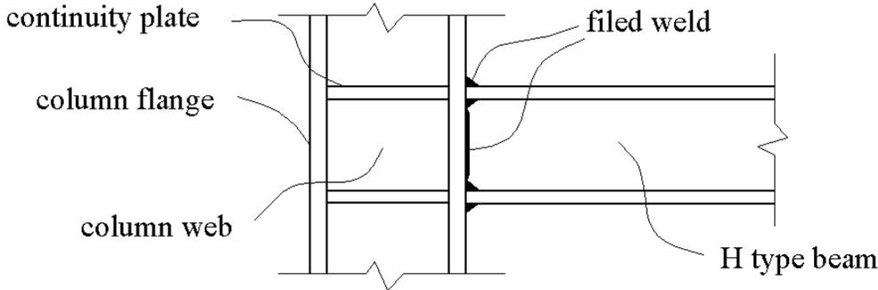
Figure 1-1 Earlier (pre-1970) Type of Welded SMRF Connection
