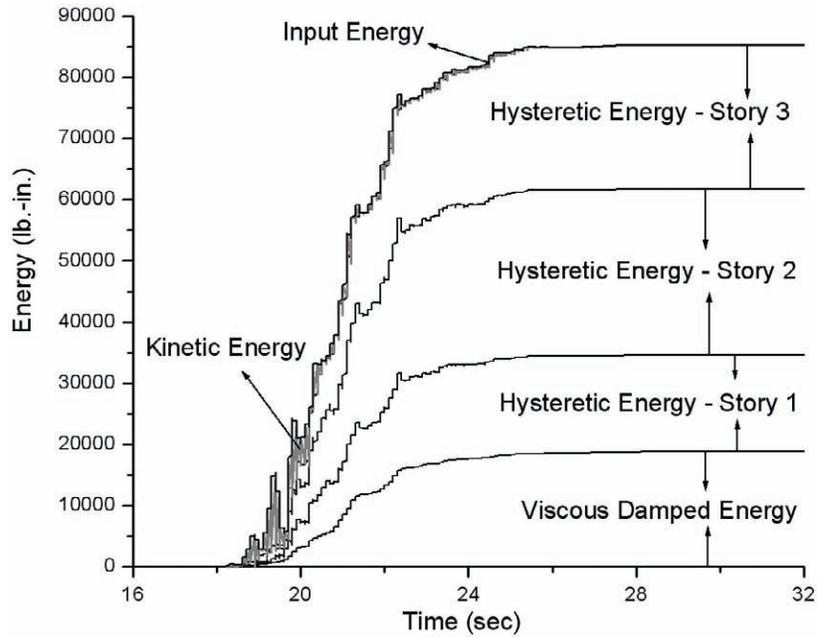
Figure 7-56 Energy Time History of the SCPT Model for Test PE6A (+125% in 1<sup>st</sup> phase)
