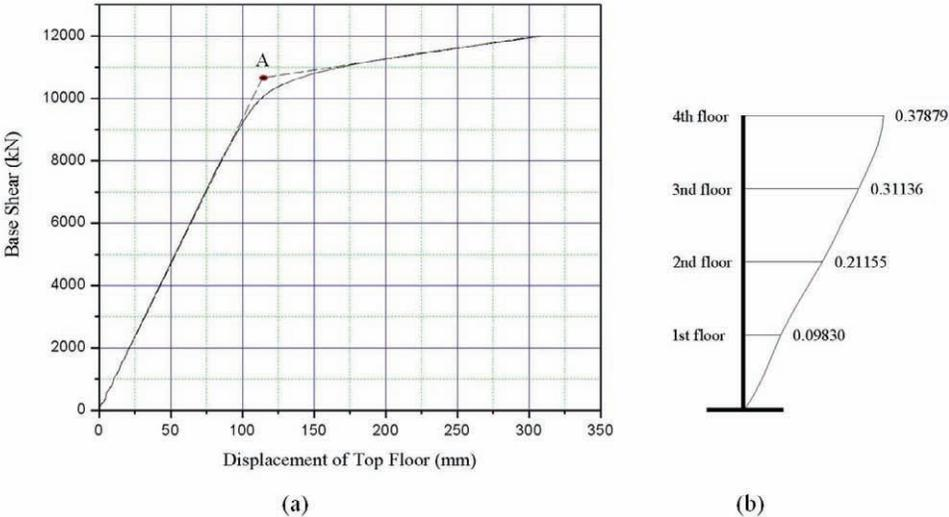
Figure 4-7 Pushover Analysis of the SMRF structure
