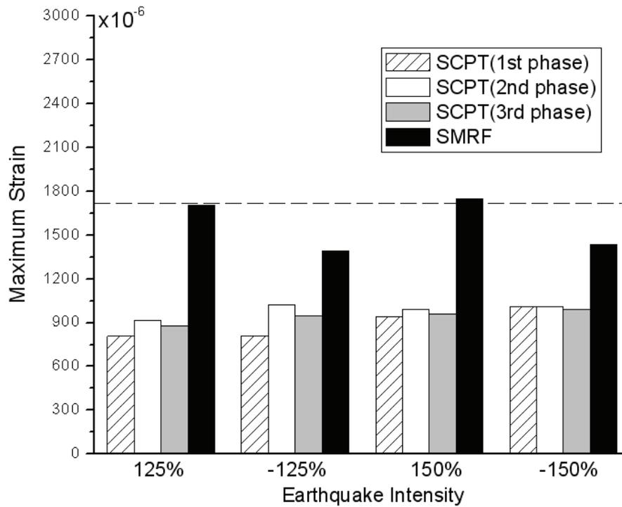
Figure 7-40 Maximum Strains of the center column of the base connection for the SCPT and SMRF Models
