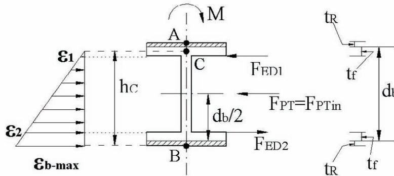
Figure 4-18 Beginning of Gap-Opening, Phase ii
