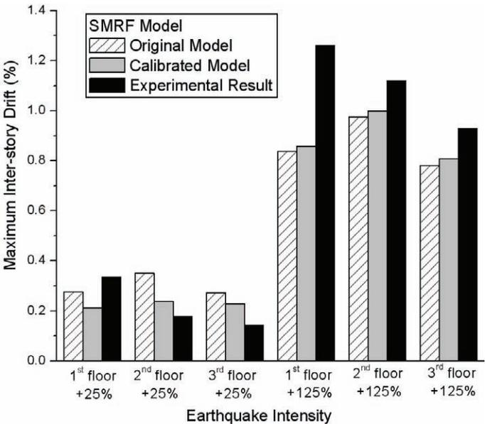
Figure 8-5 Maximum Inter-story Drifts for the SMRF Model
