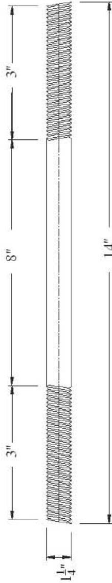
Threaded Rods (ASTM A325  $\phi 1 1/4$ , total 3 pc. and corresponding ASTM A563 nuts, 6pc.)
