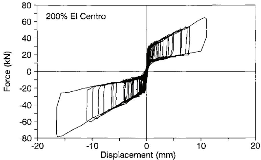
Figure 2-8 Force-Displacement Hysteresis loop of SHAPIA Damper Recorded during the Seismic Test (Filiatrault et al. 2000)
