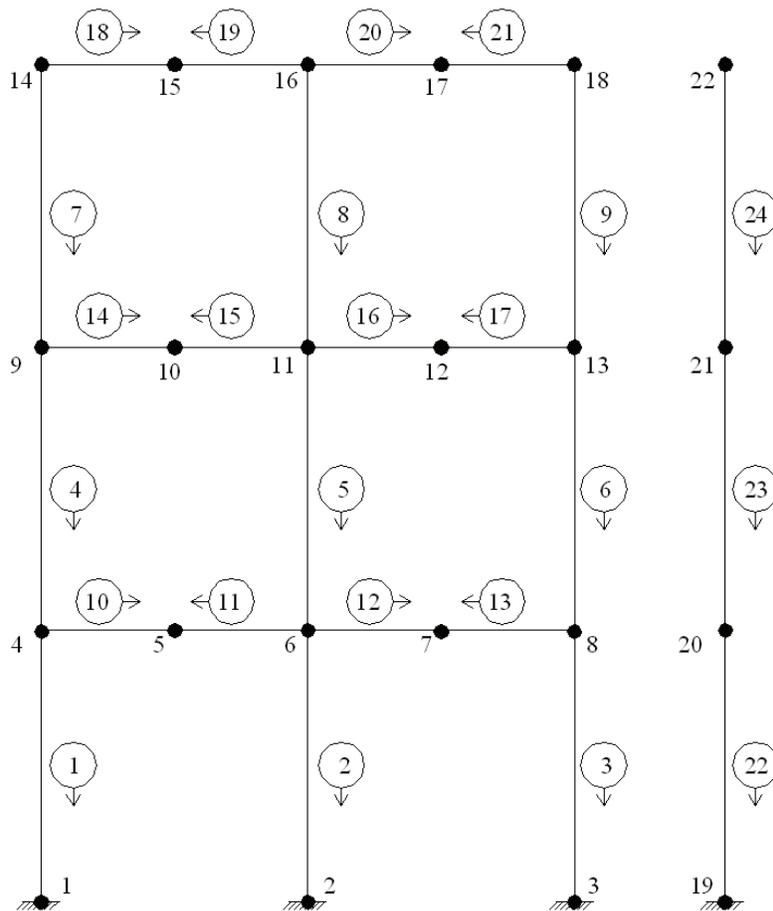
Figure 8-1 Initial Numerical Model of SMRF
