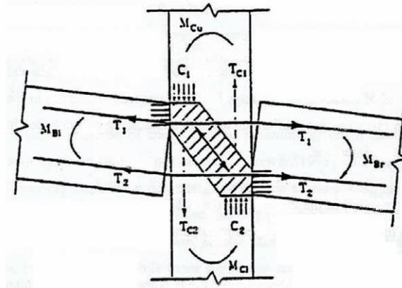
Figure 2-11 Shear Transfer Mechanism in the Joint Region with Unbonded Tendons (Priestley and Tao, 1993)
