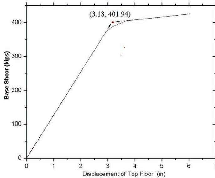
**Figure 5-6 Push-Over Analysis of SMRF Prototype**
