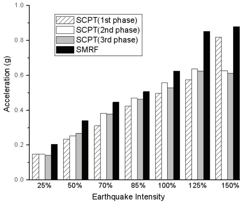
Figure 7-21 Peak Acceleration Response of the 1<sup>st</sup> floor for the SCPT and SMRF Models in Positive Direction Seismic Tests
