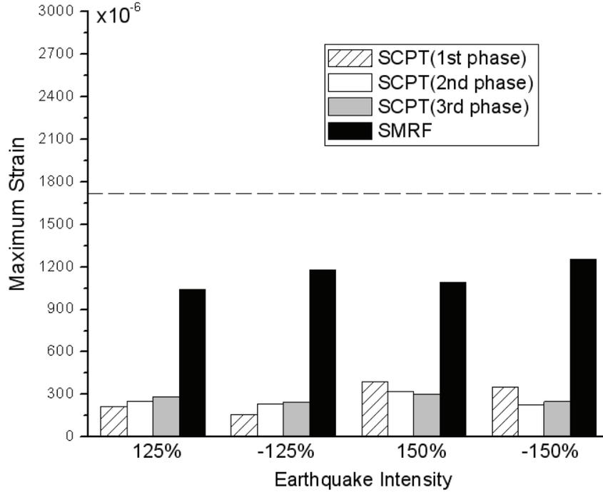
Figure 7-38 Maximum Strains of the beam of the 3<sup>rd</sup> floor for the SCPT and SMRF Models
