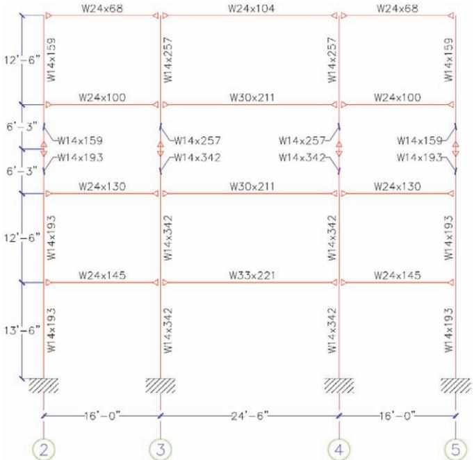
Figure 4-2 Elevation View of Exterior Moment Resisting Frame on lines B and N of WC70 (Yang and Whittaker 2002)
