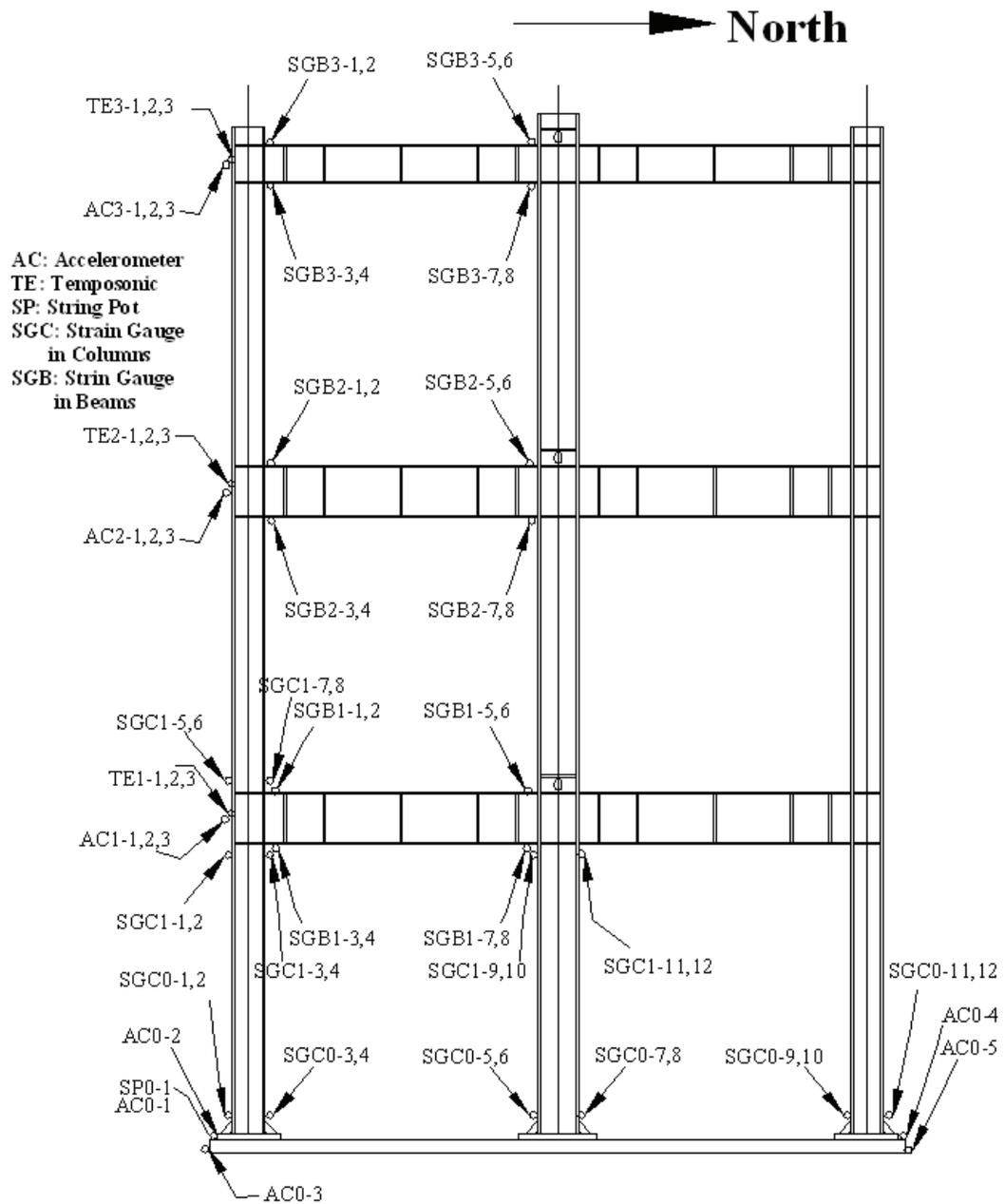
Figure 6-19 Position of Instrumentations for the SMRF Model
