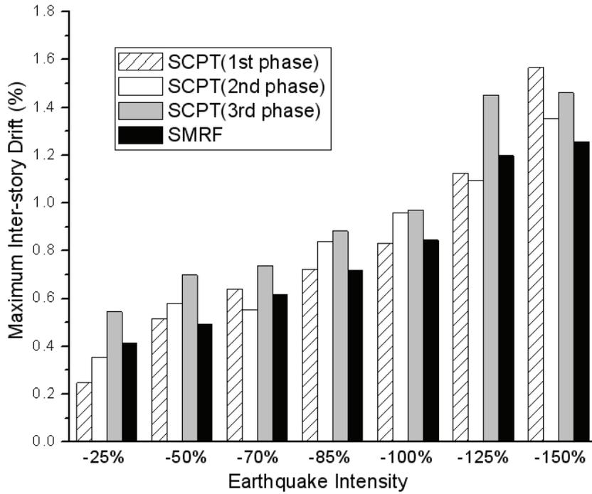
Figure 7-30 Maximum Inter-story Drift of the 1<sup>st</sup> floor for the SCPT and SMRF Models in Negative Direction Seismic Tests
