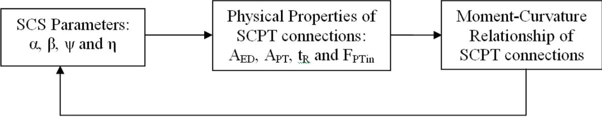
Figure 4-15 Relationship between parameters in SCS and SCPT connections
