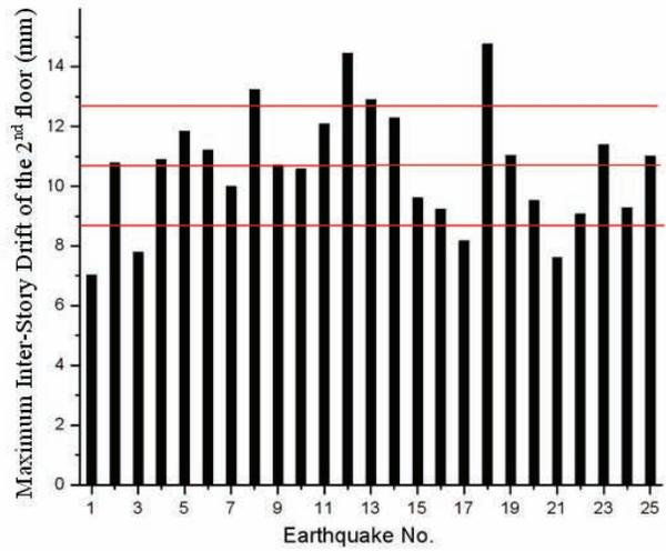
Figure 6-10 Maximum Inter-story Drift in the 2<sup>nd</sup> level
