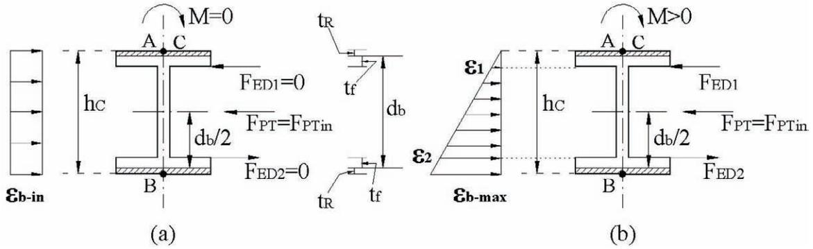
Figure 4-17 Onset of Gap-Opening, Phase i (a) beam cross section in initial position
