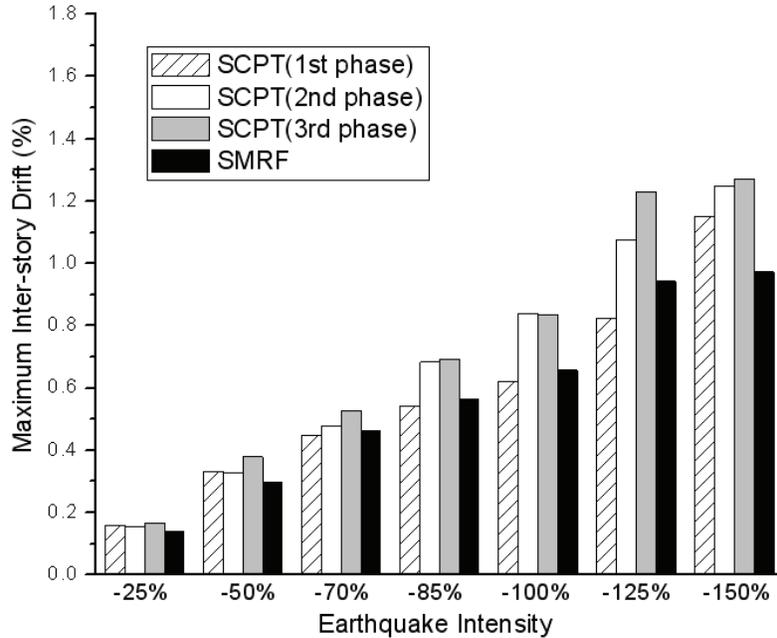
Figure 7-32 Maximum Inter-story Drift of the 3<sup>rd</sup> floor for the SCPT and SMRF Models in Negative Direction Seismic Tests
