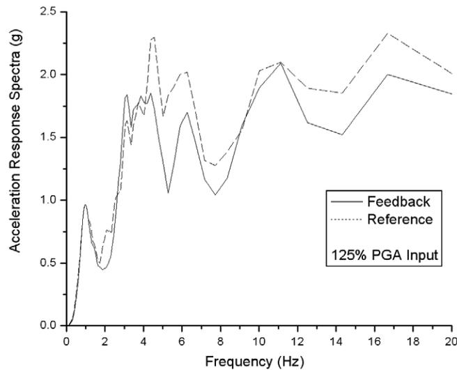
Figure 7-20 Acceleration Spectra for 125%-intensity Earthquake Excitation
