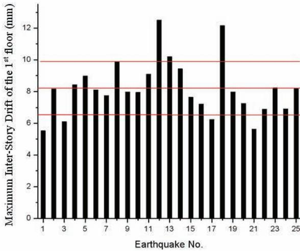
Figure 6-9 Maximum Inter-story Drift in the 1<sup>st</sup> level
