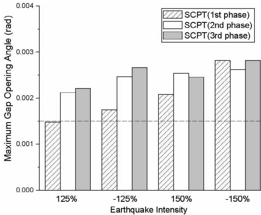
Figure 7-41 Gap Opening of the beam-column joint in 1<sup>st</sup> floor for the SCPT Model
