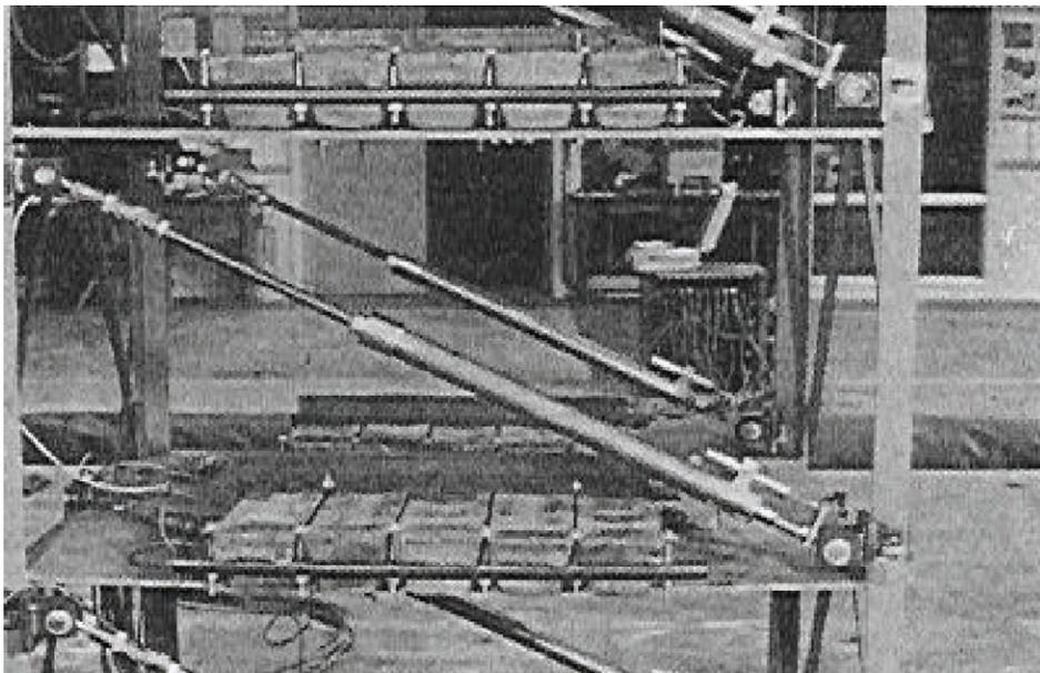
Figure 2-6 View of EDRs Installed at the Second Level of Test Frame (Aiken et al. 1993)
