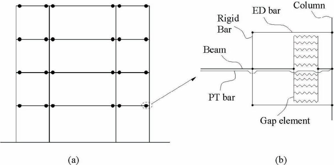
Figure 4-22 Numerical Model of WC70 Hospital Building with SCPT Connections
