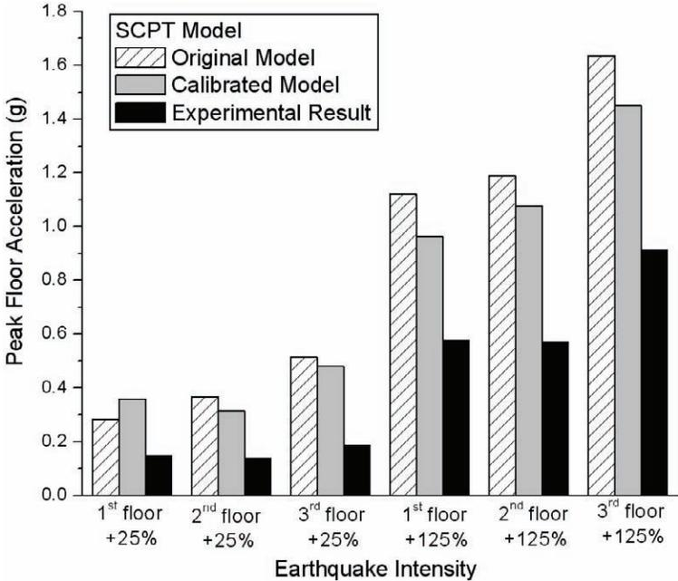
Figure 8-8 Peak Floor Acceleration of the SCPT Model
