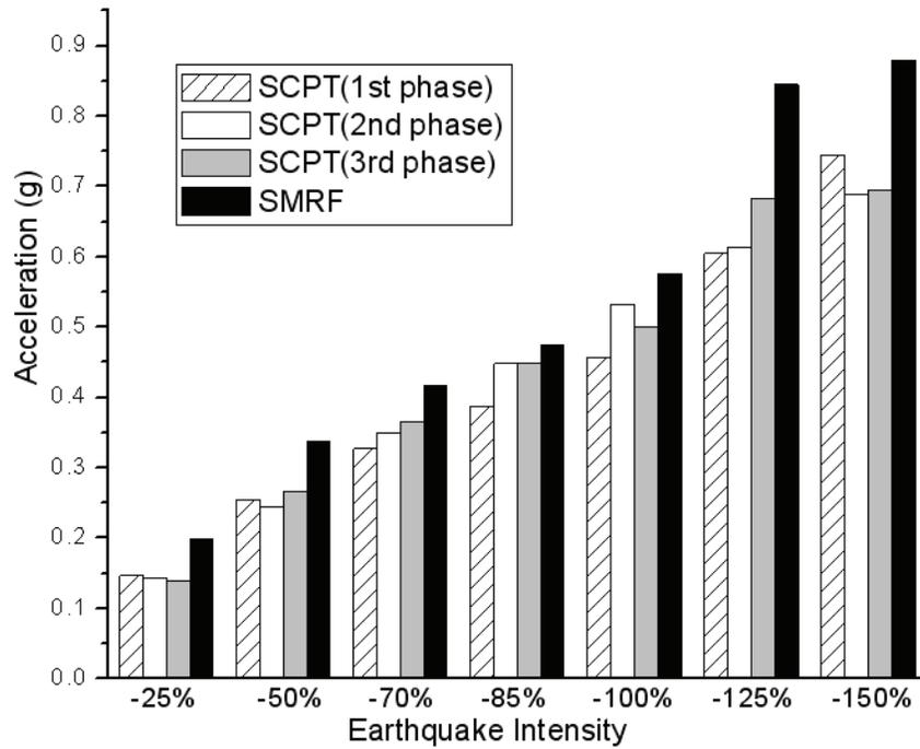
Figure 7-24 Peak Acceleration Response of the 1<sup>st</sup> floor for the SCPT and SMRF Models in Negative Direction Seismic Tests
