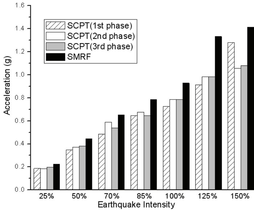
Figure 7-23 Peak Acceleration Response of the 3<sup>rd</sup> floor for the SCPT and SMRF Models in Positive Direction Seismic Tests
