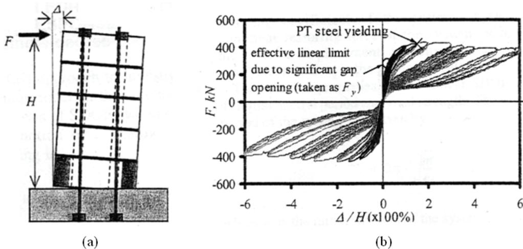
Figure 2-9 Post-Tensioned Precast Concrete Wall (a) Deformed Configuration of Unbonded PT Precast Concrete Wall (b) Experimental Cyclic lateral Load-Drift Behavior of Unbonded PT Precast Concrete Wall (Perez 2004)
