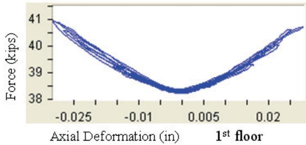
Figure 7-51 Force vs. Deformation of PT Strands For Test PE22 (+125%)
