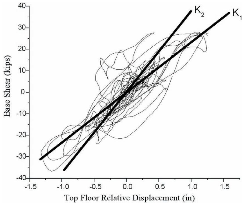
Figure 7-35 Hysteresis for the SMRF Model in test ME06A (+125% intensity)
