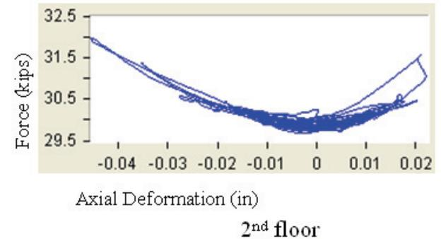
**Figure 7-45 Force vs. Deformation of PT Strands
