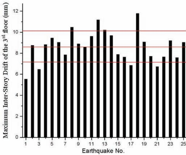
Figure 6-11 Maximum Inter-story Drift in the 3<sup>rd</sup> level
