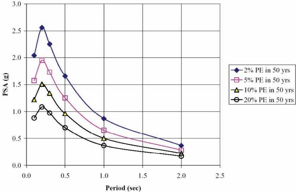
Figure 3-2 USGS Uniform Hazard Spectra: Northridge, CA (Wanitkorkul and Filiatrault, 2005)
