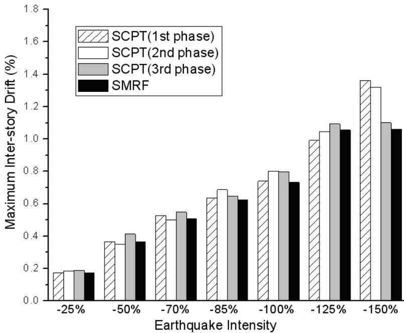
Figure 7-31 Maximum Inter-story Drift of the 2<sup>nd</sup> floor for the SCPT and SMRF Models in Negative Direction Seismic Tests
