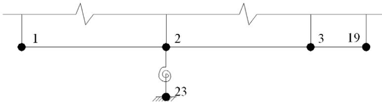
Figure 8-4 Rotational Element in the Numerical Calibrated Model
