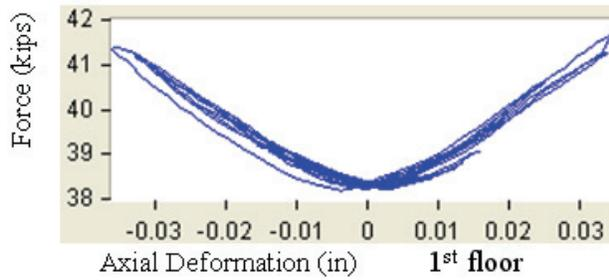
Figure 7-53 Force vs. Deformation of PT Strands For Test PE23 (+150%)
