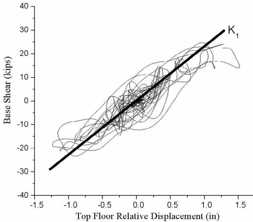
Figure 7-34 Hysteresis for the SCPT Model in test PE22 (3<sup>rd</sup> phase, +125% intensity)
