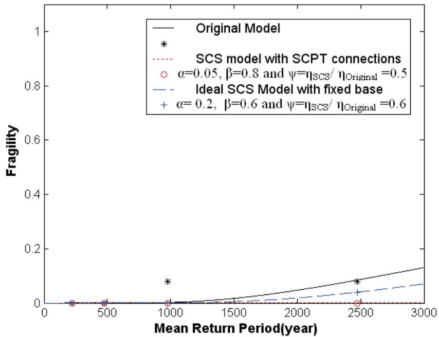
Figure 4-27 Fragility of Life Safety with the criteria of 1% permanent drift
