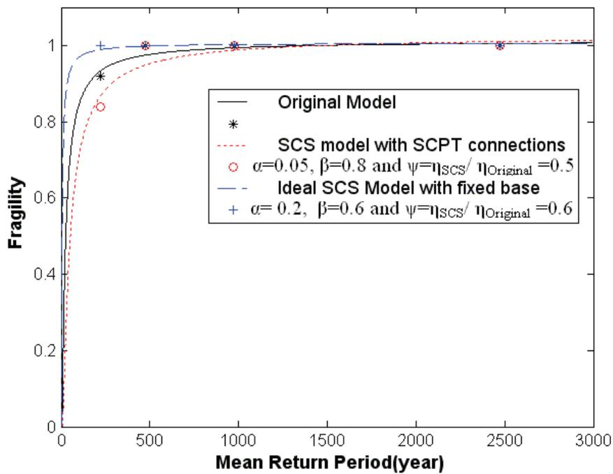
Figure 4-24 Fragility of Immediate Occupancy with the criteria of 0.7% transient drift
