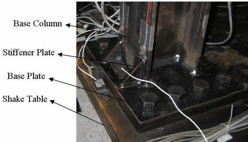
Figure 6-2 Base Column Connection of SMRF Model
