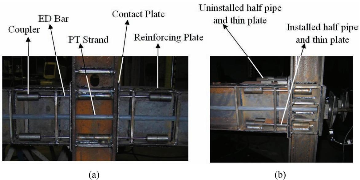
Figure 6-5 Beam-Column Connections in the SCPT Frame1 Model
