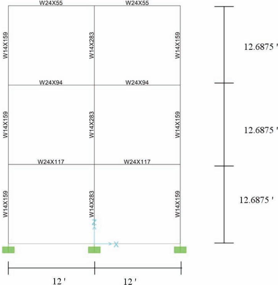
Figure 5-3 Prototype Frame
