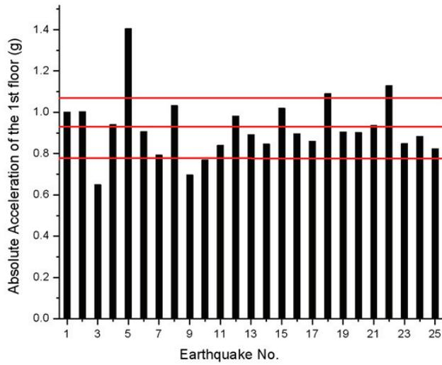
Figure 6-13 Maximum Acceleration in the 1<sup>st</sup> level
