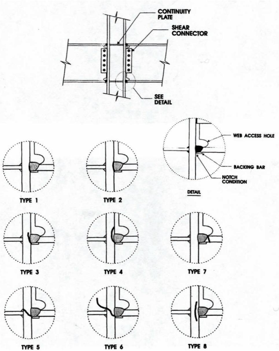
Figure 1-4 Eight Types of Fractures in Beam-Column Connections Identified as a Result of the Northridge Earthquake (Tremblay et al. 1995)
