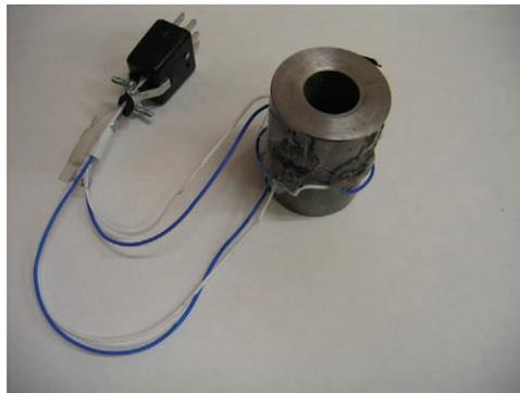
Figure 6-17 Load Cell
