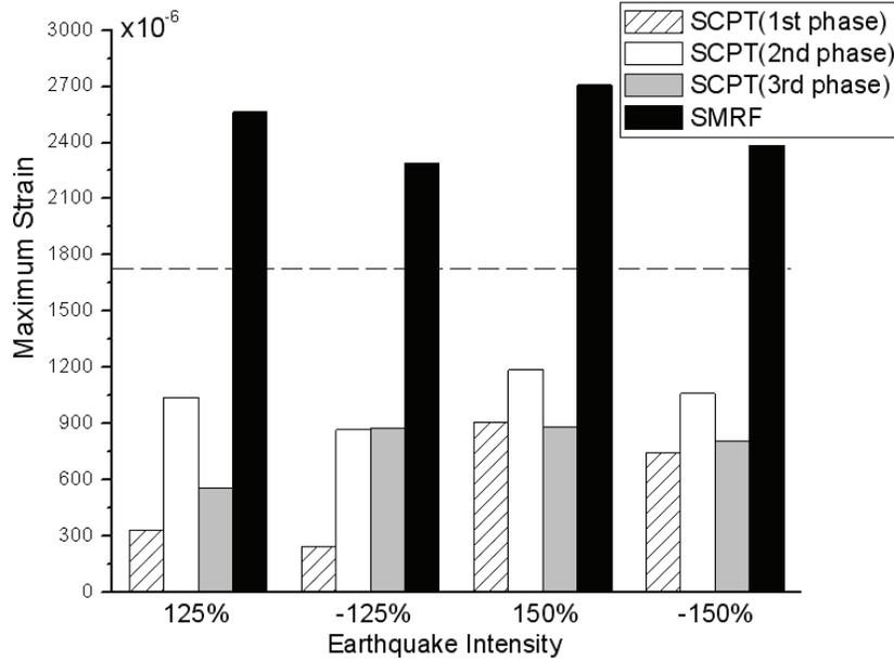
Figure 7-36 Maximum Strains of the beam of the 1<sup>st</sup> floor for the SCPT and SMRF Models
