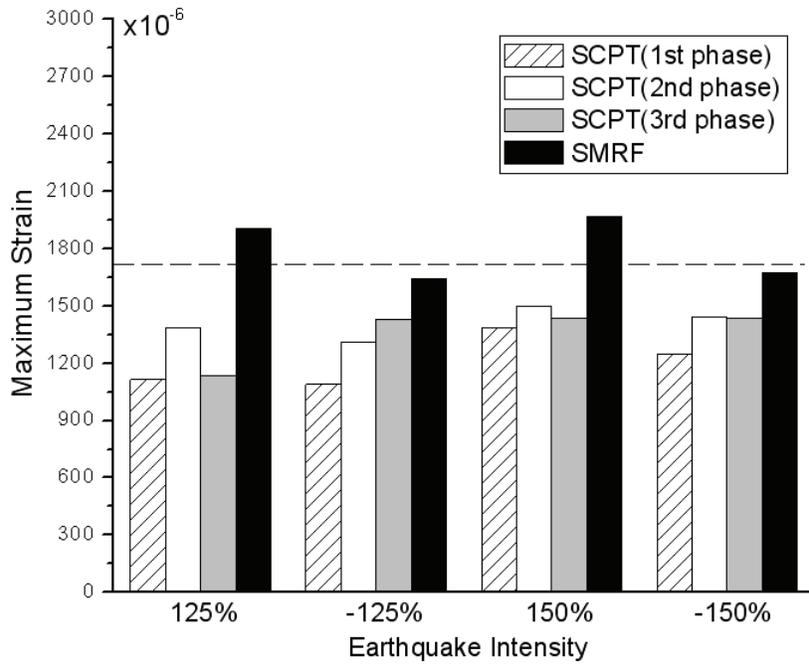
Figure 7-39 Maximum Strains of the exterior column of the base connection for the SCPT and SMRF Models
