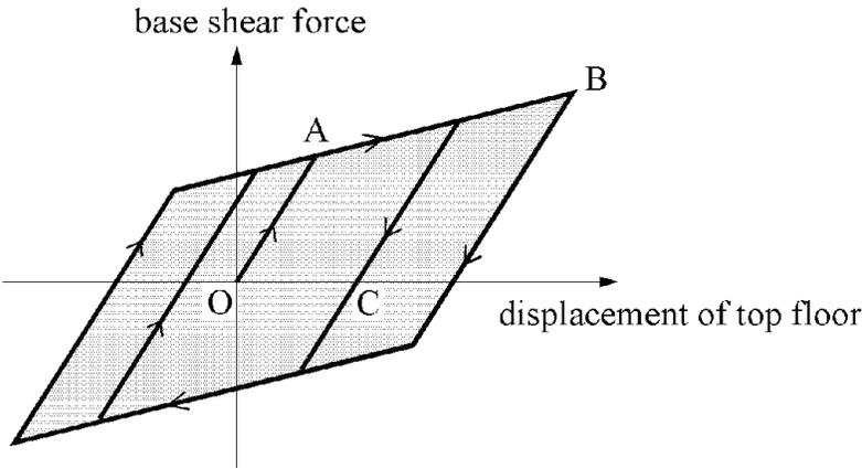
Figure 1-5 Ideal Inelastic Seismic Response of Elasto-Plastic Systems (EPS)
