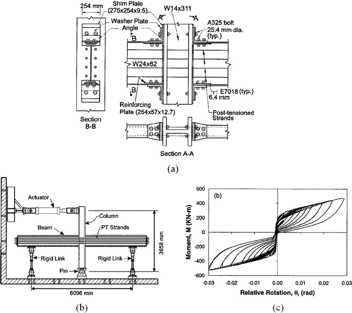
Figure 2-13 Post-Tensioned Connections Test (a) Post-Tensioned Specimen Connection (b) Post-Tensioned Connection Subassembly Setup (c) Moment-Rotation Response of a PT Connection (Ricles, et al. 2002)
