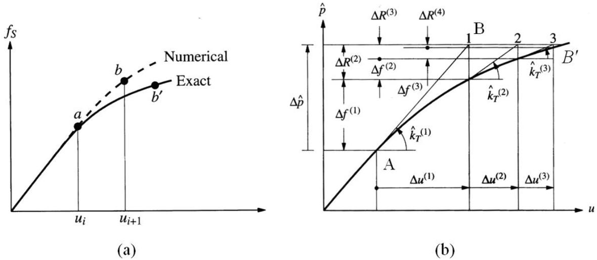
Figure 3-3 Error in Newmark's Method (a) Numerical Error in Newmark's method (b) Newton-Raphson Iteration (Chopra 2000)
