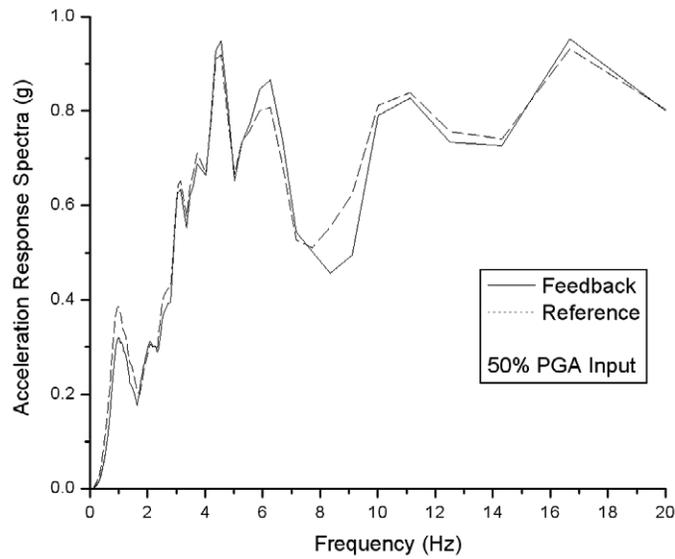
Figure 7-19 Acceleration Spectra for 50%-intensity Earthquake Excitation
