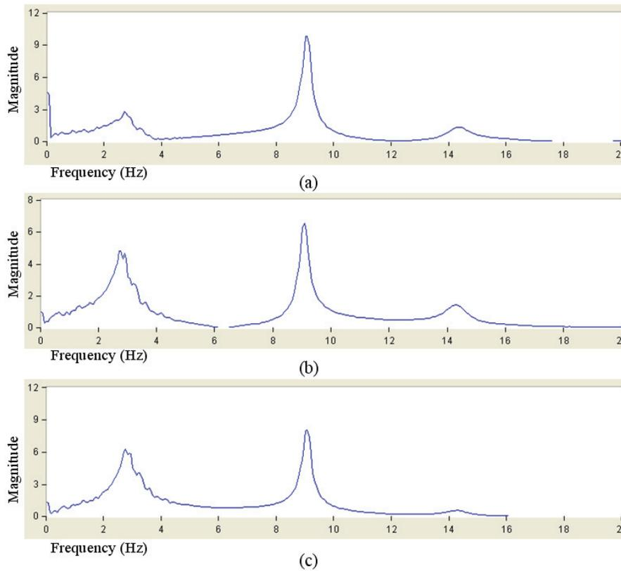
Figure 7-17 Transfer Functions in the SCPT model from the Sine Sweep Test
