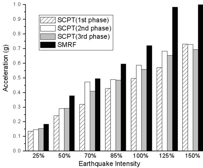
Figure 7-22 Peak Acceleration Response of the 2<sup>nd</sup> floor for the SCPT and SMRF Models in Positive Direction Seismic Tests
