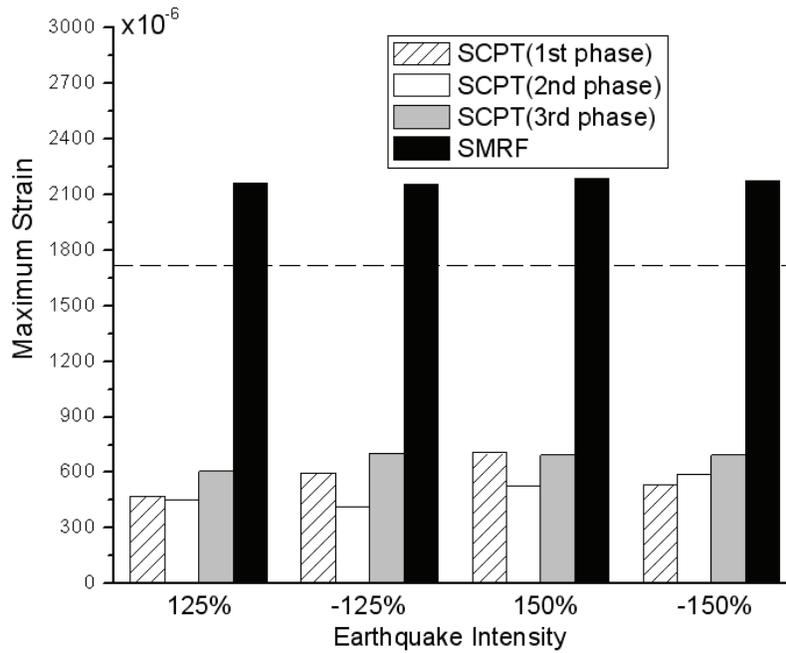
Figure 7-37 Maximum Strains of the beam of the 2<sup>nd</sup> floor for the SCPT and SMRF Models
