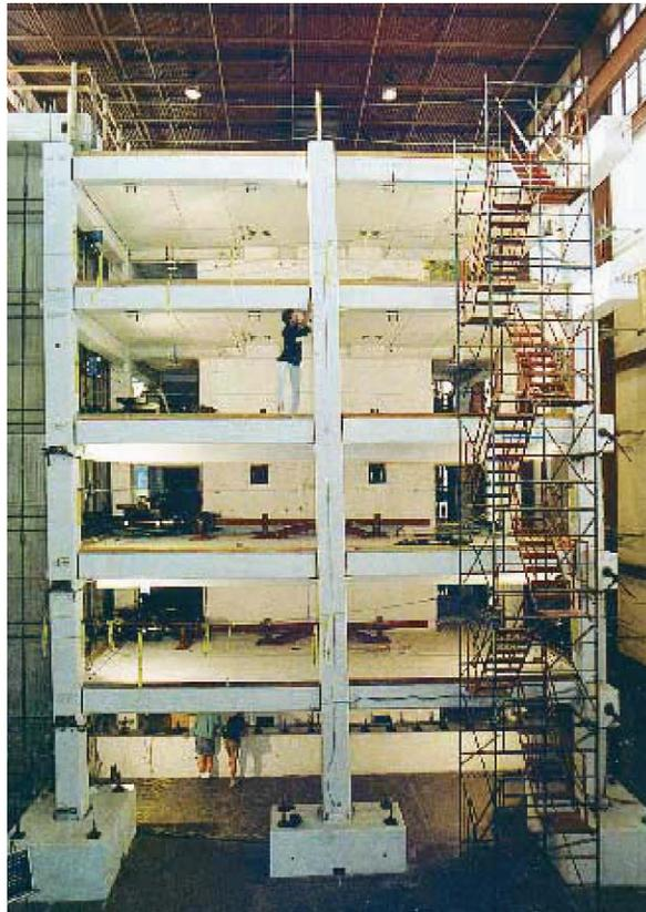
Figure 2-12 Overall View of Five-Story Building under Test (Priestley et al. 1999)
