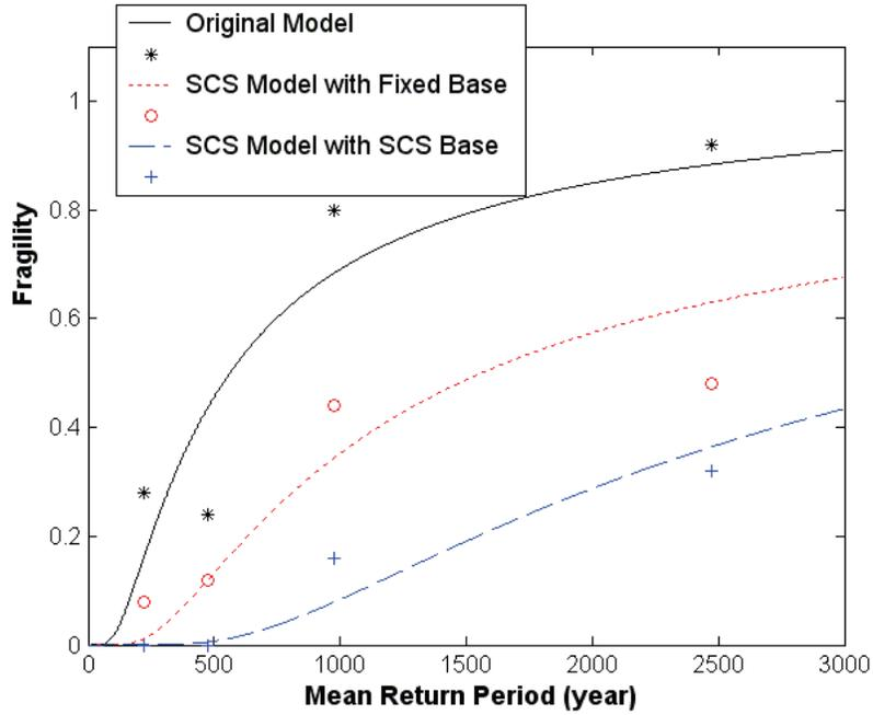
Figure 4-11 Fragility of Immediate Occupancy with 0.2% permanent drift criteria
