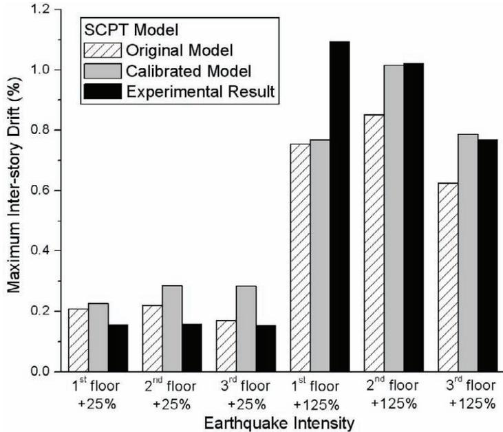
Figure 8-7 Maximum Inter-story Drift of the SCPT Model
