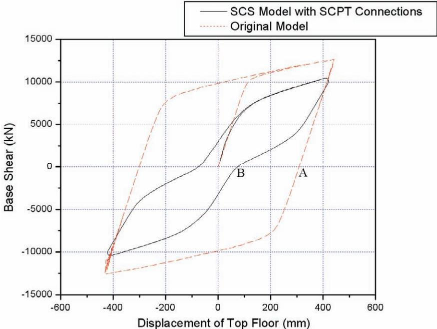
Figure 4-23 Push-Over Analysis for two models
