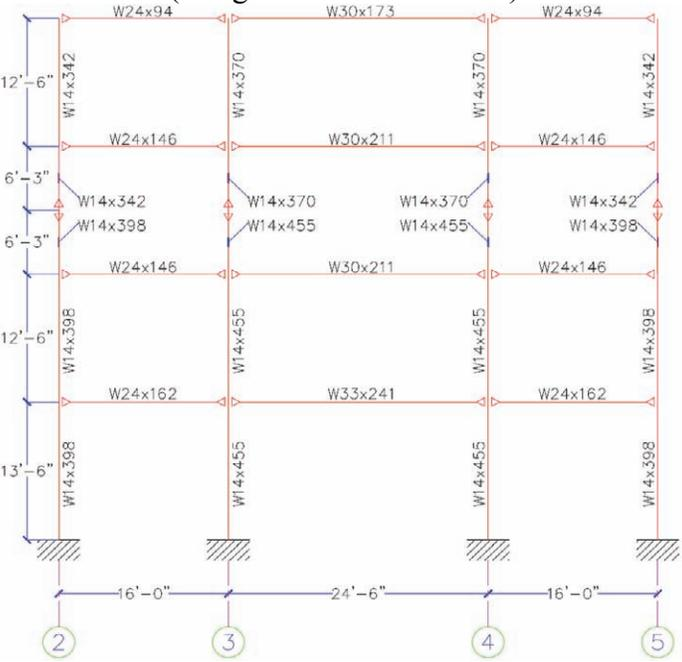
Figure 4-3 Elevation View of Interior Moment Resisting Frame on lines F and J of WC70 (Yang and Whittaker 2002)
