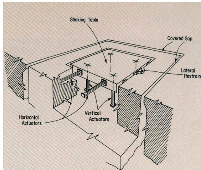
Figure 6-8 Perspective View of Shaking Table and Foundation
