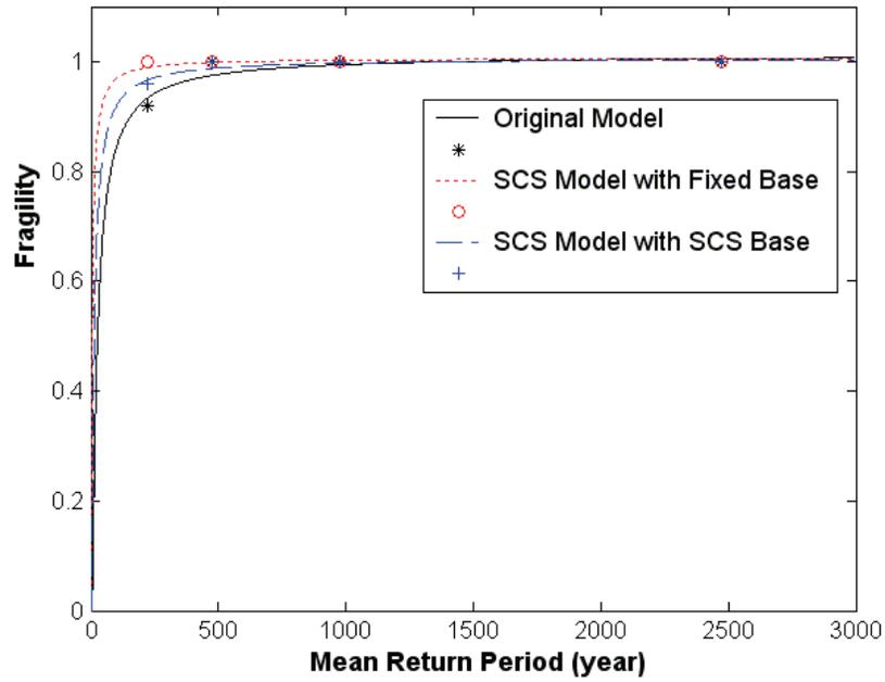
Figure 4-10 Fragility of Immediate Occupancy with 0.7% transient drift criteria
