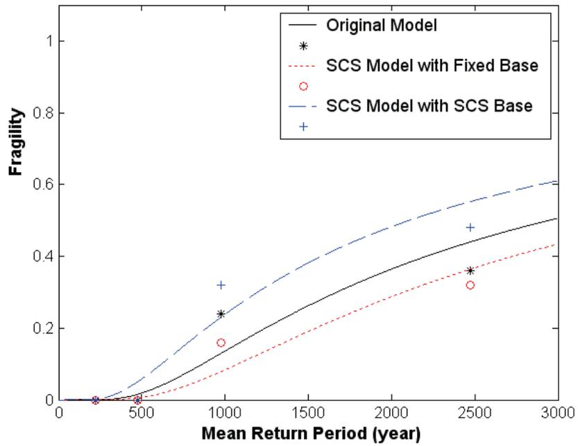
Figure 4-12 Fragility of Life Safety with 2.5% transient drift criteria
