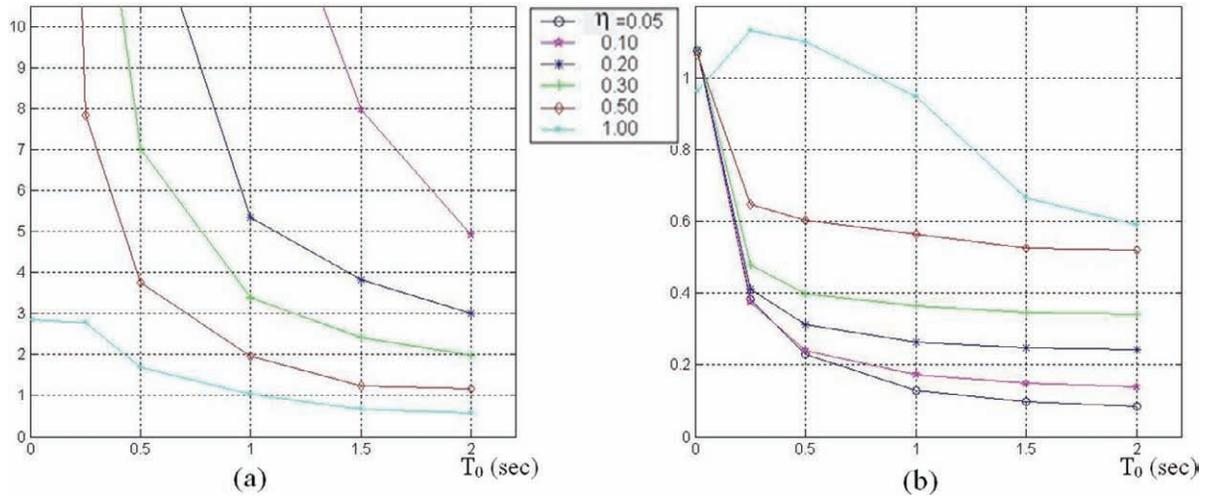
Figure 3-8 Seismic Responses of EPS under Ground Motions having 2% Probability of Exceedance in 50 years (a) Mean Displacement Ductility (b) Mean Maximum Absolute Acceleration (g)
