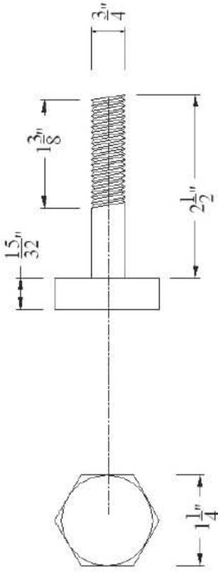
Headed Anchor Bolts (ASTM A325  $\phi 3/4$ , total 24 pc.)
