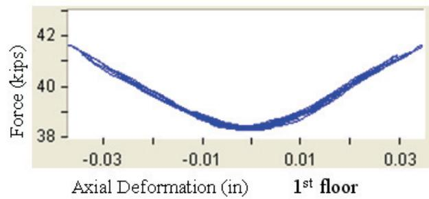
Figure 7-52 Force vs. Deformation of PT Strands For Test PER22 (-125%)
