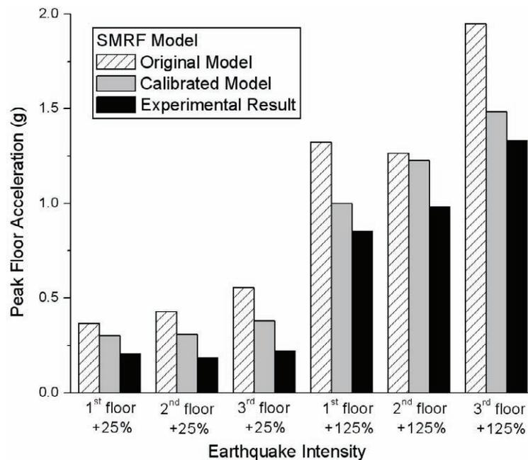
Figure 8-6 Peak Floor Accelerations for the SMRF Model
