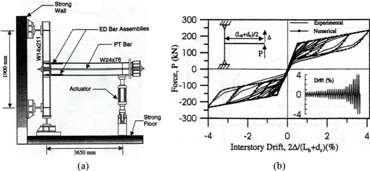
Figure 2-15 Cyclic Testing of a PTED connection (a) Experimental Setup (b) Experimental and Numerical Force-Interstory Drift Response (Christopoulos et al., 2002b)
