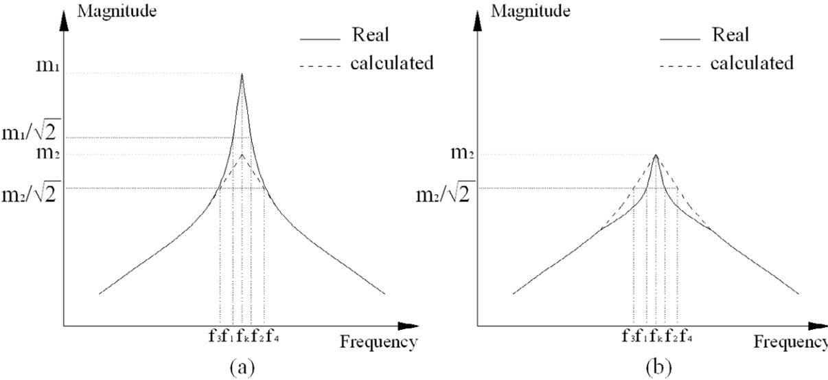
Figure 7-18 Transfer Function for Estimating Damping Ratio
