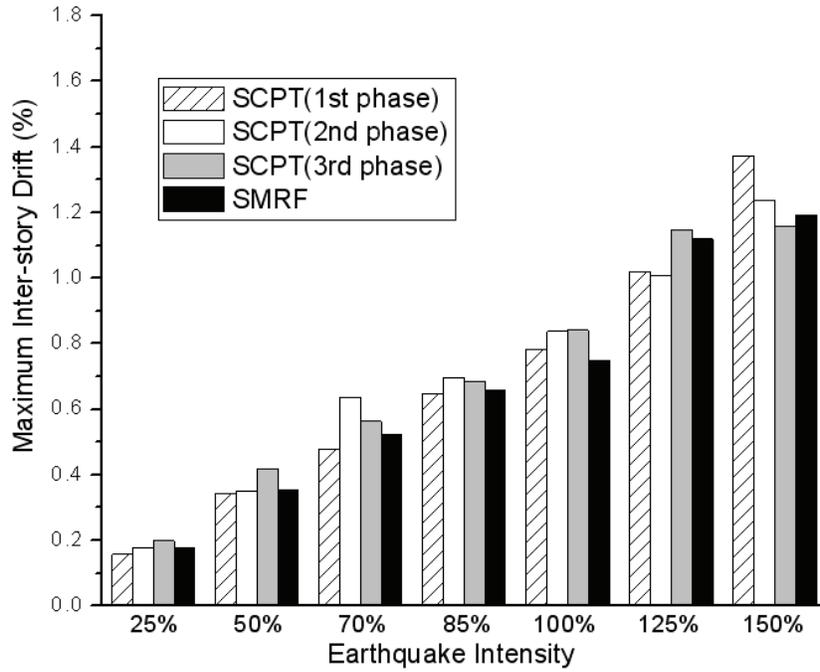
Figure 7-28 Maximum Inter-story Drift of the 2<sup>nd</sup> floor for the SCPT and SMRF Models in Positive Direction Seismic Tests
