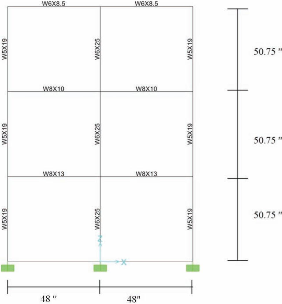
Figure 5-4 SMRF Model Configuration
