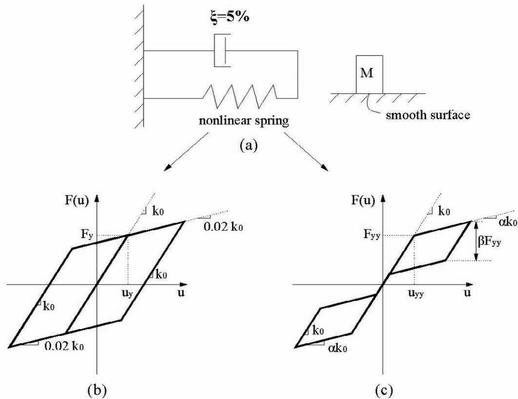
Figure 3-1 SDOF Numerical Model (a) SDOF system (b) Hysteretic Loop of Elasto-Plastic Systems (EPS) (c) Hysteretic Loop of Self-Centering Systems (SCS)
