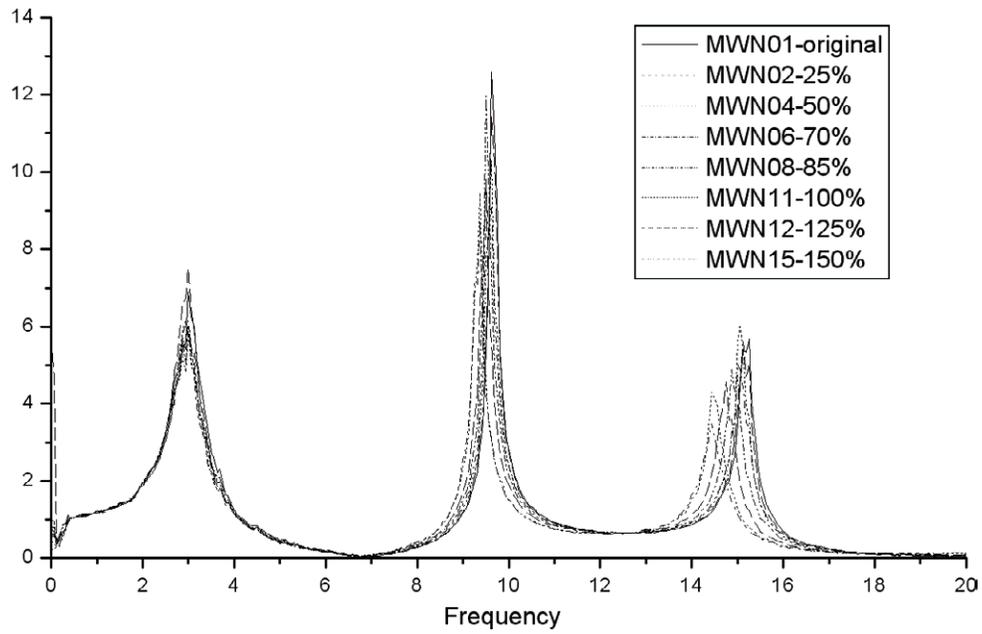
Figure 7-10 Transfer Functions for White Noise Tests, SMRF Model
