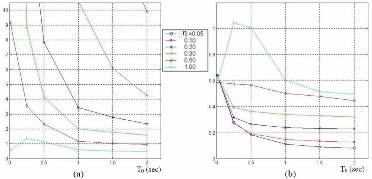
Figure 3-9 Seismic Responses of EPS under Ground Motions having 10% Probability of Exceedance in 50 years (a) Mean Displacement Ductility (b) Mean Maximum Absolute Acceleration (g)
