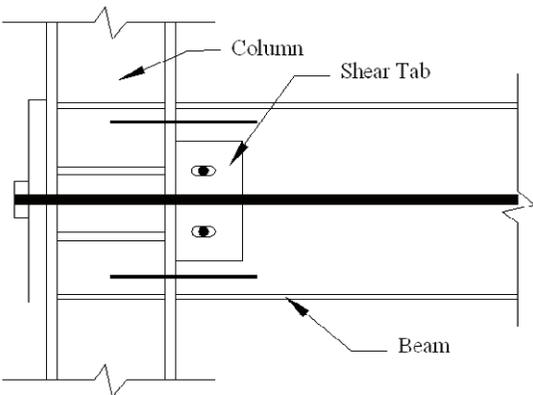
Figure 7-55 Beam-to-Column Connection in SCPT Structures
