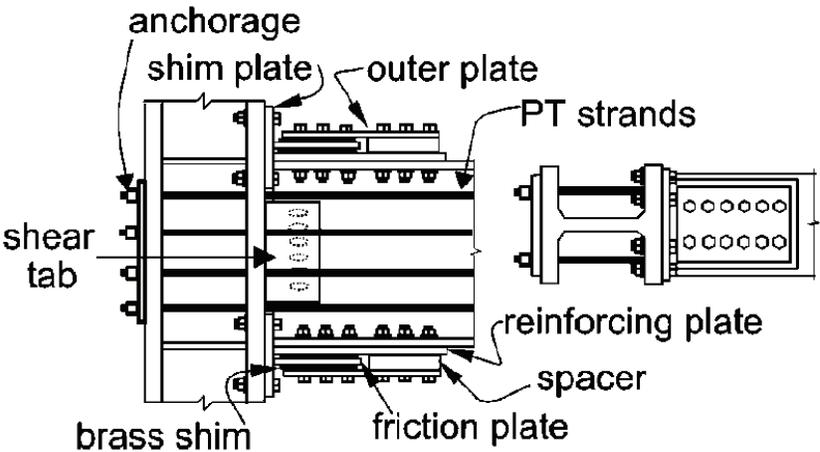
Figure 2-16 Post-tensioned Friction Damped Connection (PFDC) Details (Rojas et al. 2005)
