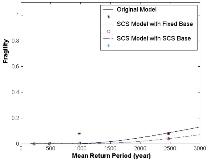
Figure 4-13 Fragility in Life Safety with 1% permanent drift criteria
