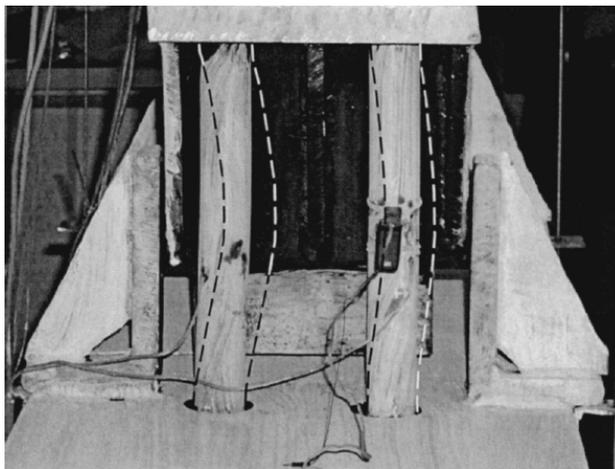
Figure 2-3 Recovered-deformation of Connections with SMA after Heating: dashed lines represent residual shape before heating (Ocel et al. 2004)
