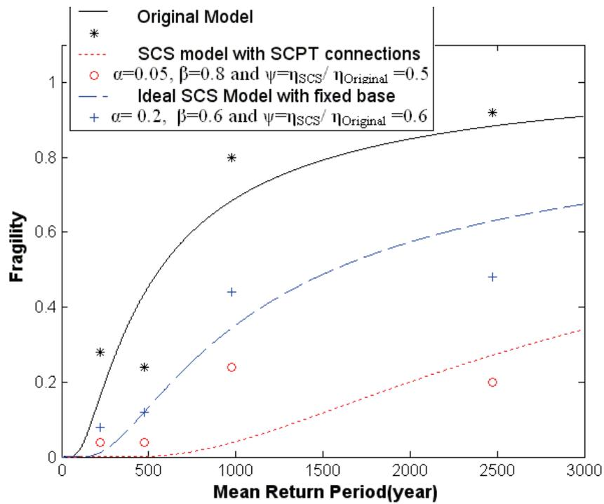
Figure 4-25 Fragility of Immediate Occupancy with the criteria of 0.2% permanent drift
