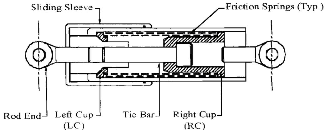
Figure 2-7 Diagrammatic View of the SHAPIA Damper (Filiatrault et al. 2000)
