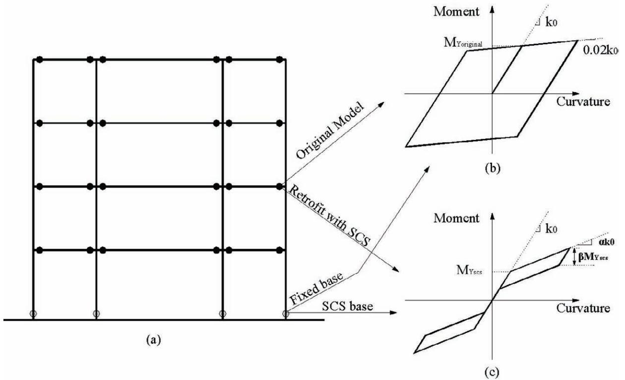
Figure 4-8 Numerical Models of EPS and SCS
