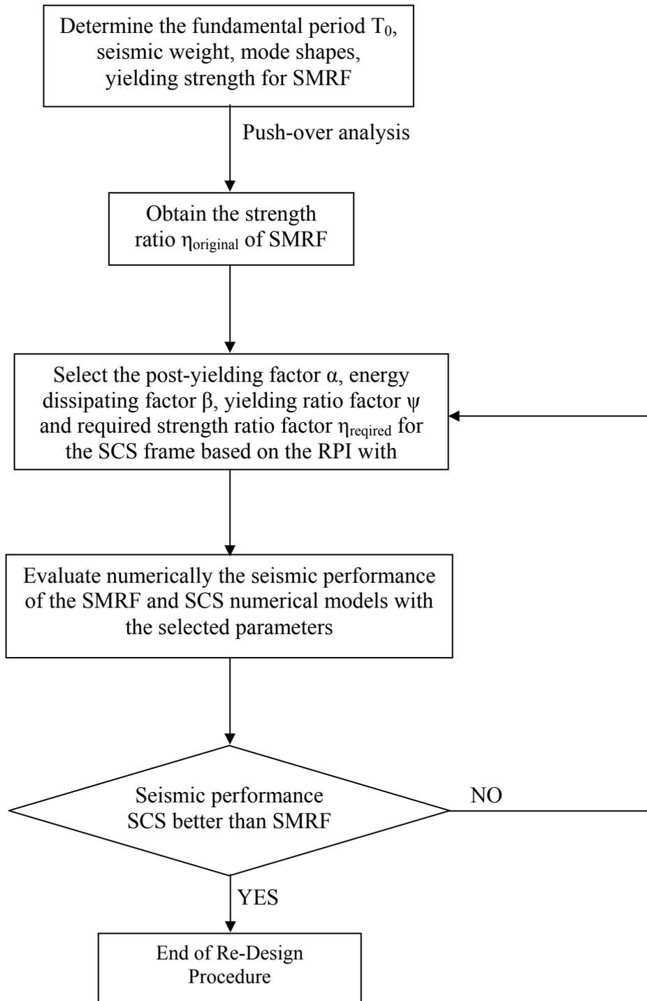
Figure 4-6 Flowchart of the Re-Design Procedure for Ideal SCS Frame
