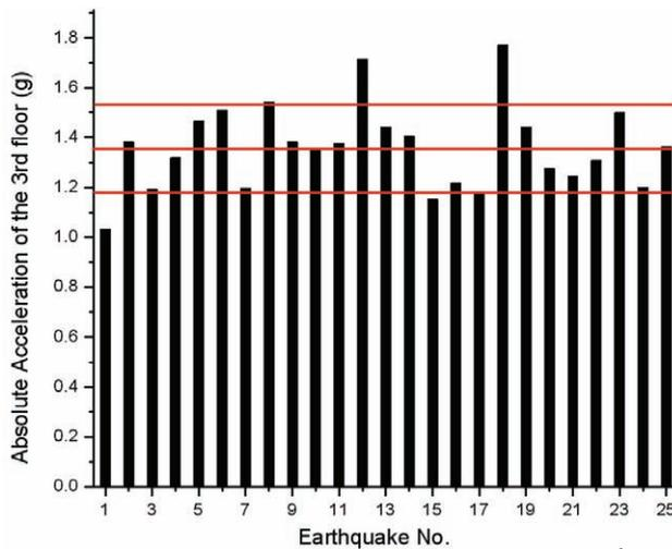
Figure 6-15 Maximum Acceleration in the 3<sup>rd</sup> level
