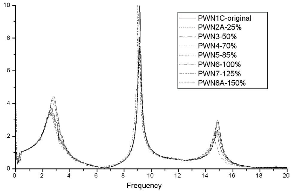
Figure 7-8 Transfer Functions for White Noise Tests, SCPT Model
