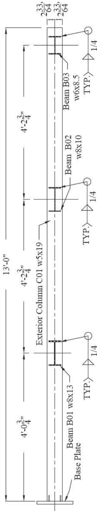
Exterior Beam-Column Connections
