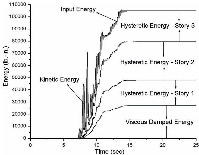
Figure 7-57 Energy Time History of the SMRF Model for Test ME06A (+125%)
