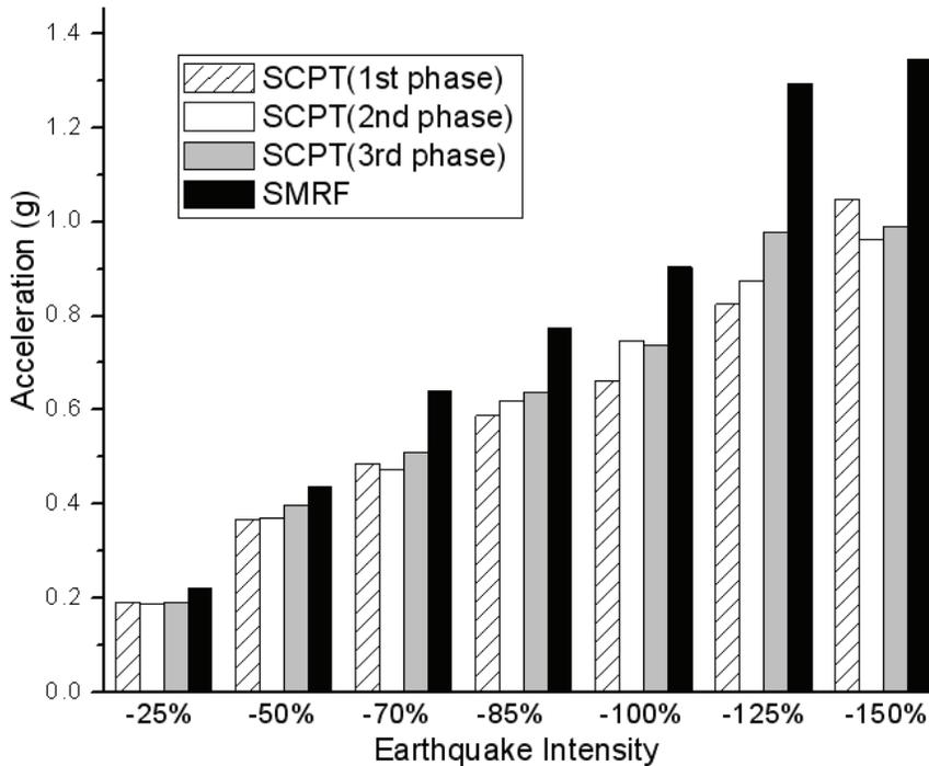
Figure 7-26 Peak Acceleration Response of the 3<sup>rd</sup> floor for the SCPT and SMRF Models in Negative Direction Seismic Tests
