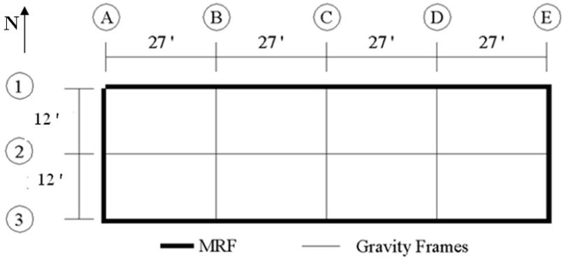
Figure 5-2 Plan View of Prototype Building
