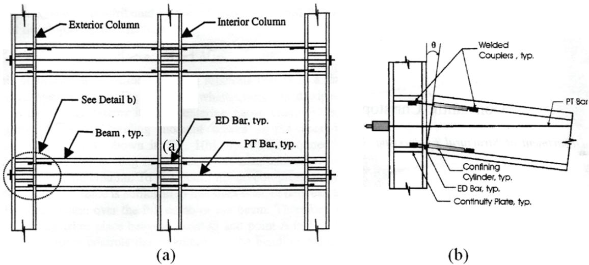
Figure 2-14 Concept of PTED connections (a) Steel Frame with PTED Connections (b) Geometric Configuration of Exterior PTED Connections (Christopoulos et al, 2002a)
