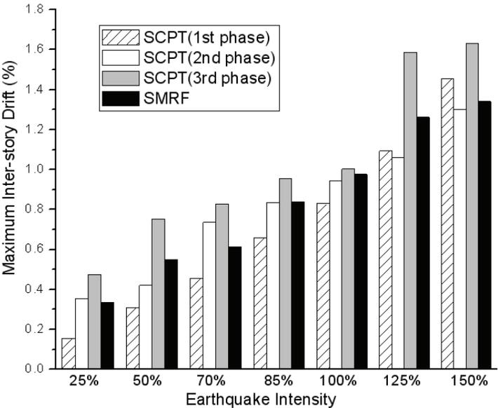
Figure 7-27 Maximum Inter-story Drift of the 1<sup>st</sup> floor for the SCPT and SMRF Models in Positive Direction Seismic Tests
