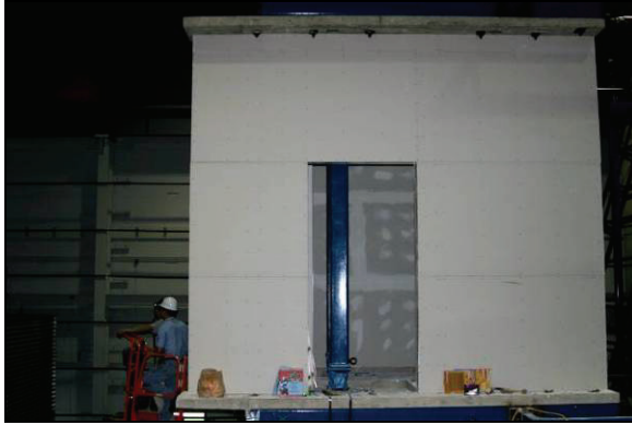
Figure 5.16. General view of gypsum wallboard panels in south wall
