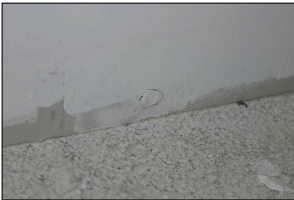
(a) Screw rising observed at a 0.47% drift ratio
