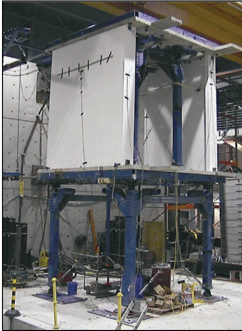
Figure 3.12. Partition walls tested on the UB-NCS with approximate dimensions
