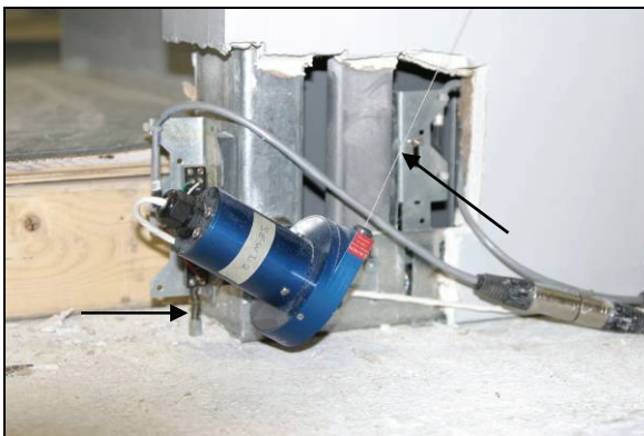
Figure 5.57. Detail of instrumentation at wall boundary. In the photo: string pot SEWD2, and potentiometers SEWVBW and SEWVBWi
