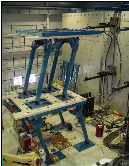
Figure 5.1. Photograph of UB-NCS with concrete slabs
