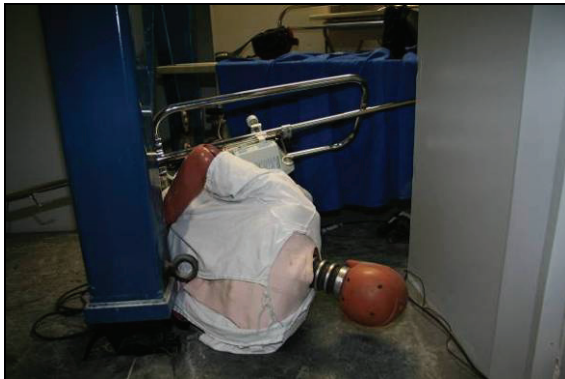
(e) Dummy thrown off medical gurney and pole fell down over dummy
