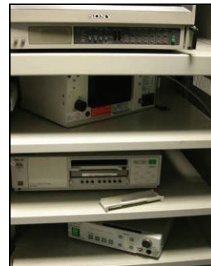
(l) Excessive displacement and rotation of surgical video rack contents
