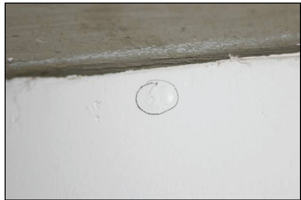
(b) Screw rising observed at a 0.47% drift ratio
