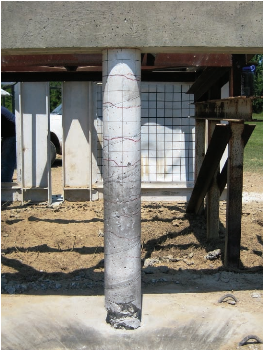
Figure 3-46 Front View of Column RC2 (Test 2)
