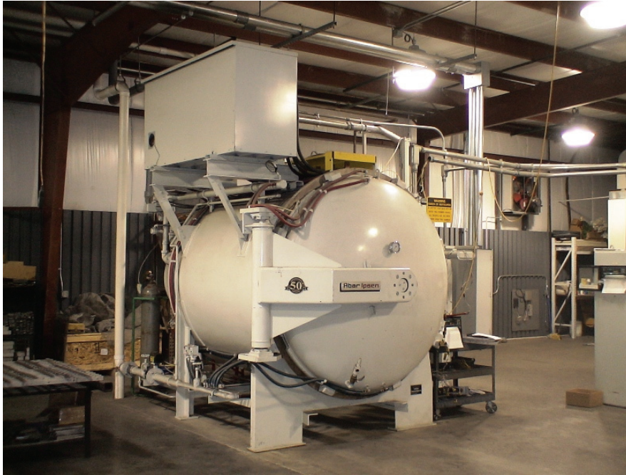
Figure 3-10 Vacuum Furnace for Annealing
