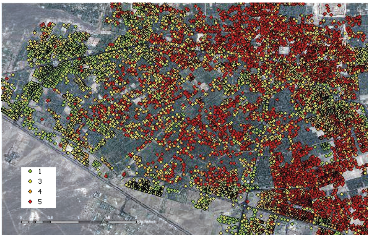
Figure 1-3 Validation Dataset for Bam, Showing EMS Damage Levels 1, 3, 4 & 5. Courtesy of Yamazaki et al. (2004)
