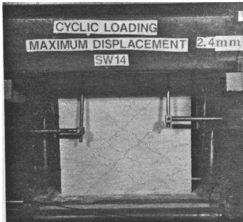
Figure C-121 Condition of wall SW14 at 0.48% drift [Lopes and Elnashai (1991)]
