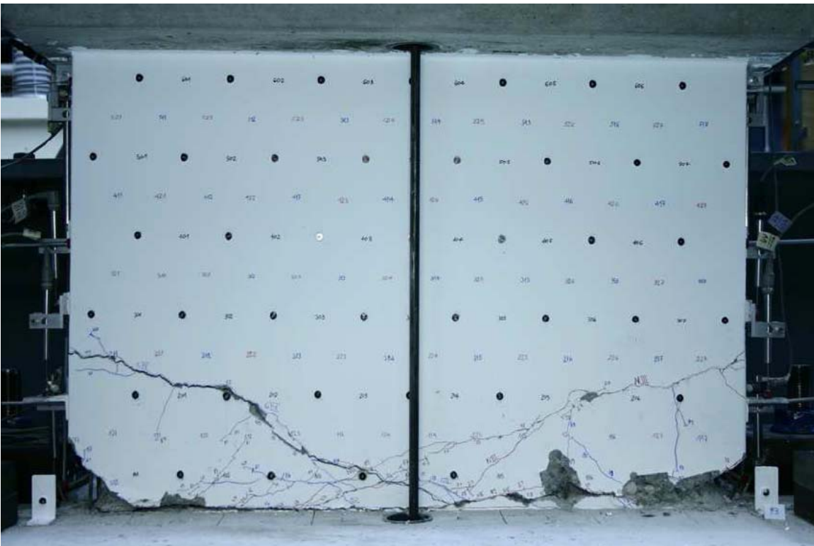
Figure C-93 Condition of wall M4 at -2.05% drift [Greifenhagen et al. (2005)]
