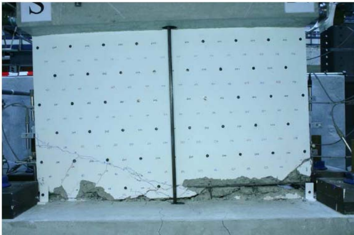
Figure C-71 Condition of wall M1 at 4.19% drift [Greifenhagen et al. (2005)]
