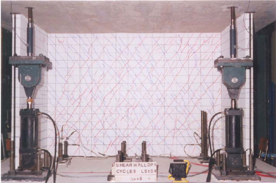
Figure C-296 Condition of wall DP1 at 0.40% drift [Palermo and Vecchio (2002)]
