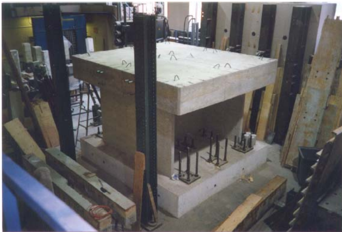
Figure 5-7 Wall DP1 before testing [Palermo and Vecchio (2002a)]
