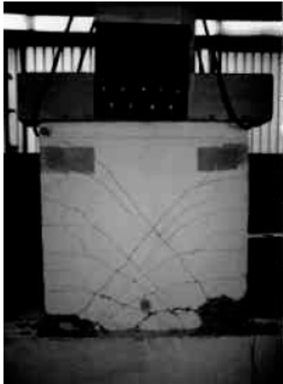
Figure C-181 Condition of wall LSW3 at the end of the test (maximum drift = 1.43%) [Salonikios et al. (1999)]
