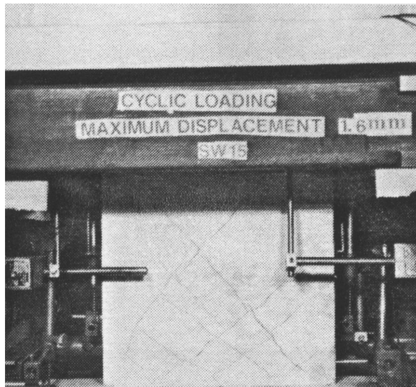
Figure C-130 Condition of wall SW15 at 0.32% drift [Lopes and Elnashai (1991)]
