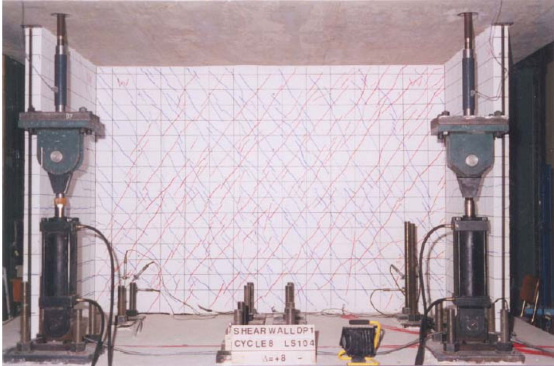
Figure 8-5 Cracking pattern for wall DP1 tested by Palermo and Vecchio (2002a) at a maximum shear crack width of 0.5 mm
