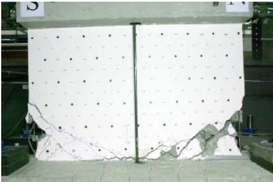
Figure C-79 Condition of wall M2 at 2.52% drift [Greifenhagen et al. (2005)]
