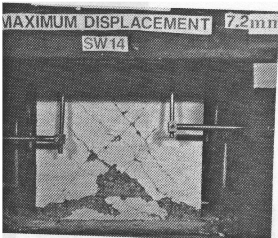
Figure C-127 Condition of wall SW14 at 1.45% drift [Lopes and Elnashai (1991)]
