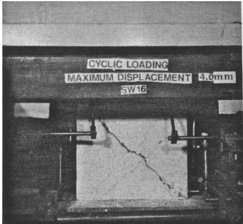
Figure C-139 Condition of wall SW16 at 0.81% drift [Lopes and Elnashai (1991)]
