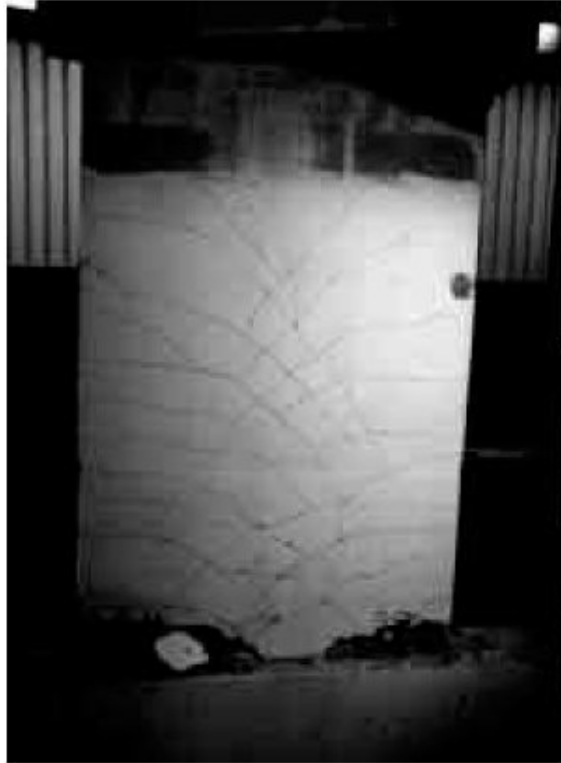
Figure C-183 Condition of wall MSW1 at the end of the test (maximum drift = 1.53%) [Salonikios et al. (1999)]
