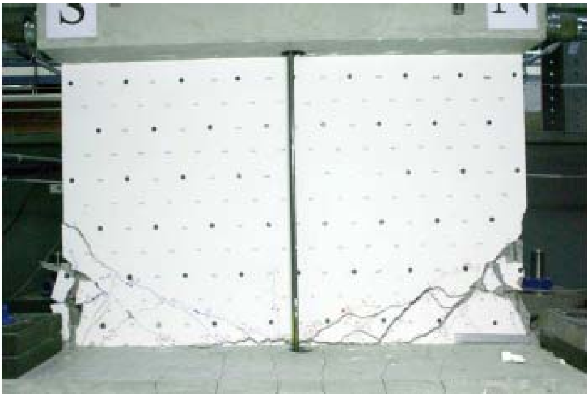
Figure C-77 Condition of wall M2 at 1.98% drift [Greifenhagen et al. (2005)]
