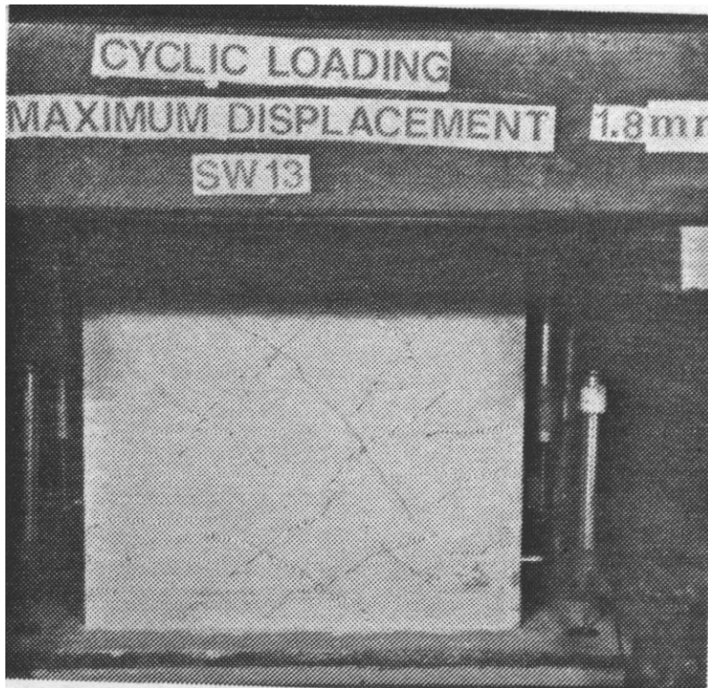
Figure C-112 Condition of wall SW13 at 0.36% drift [Lopes and Elnashai (1991)]
