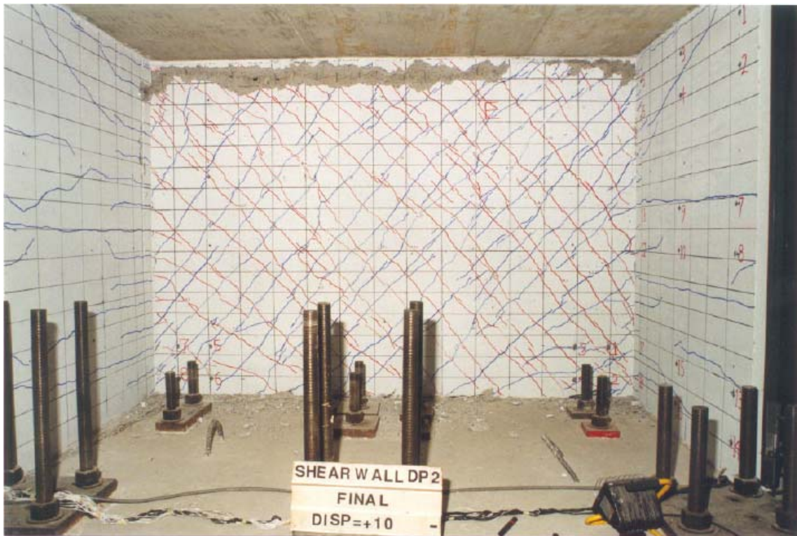
Figure C-314 Condition of wall DP2 at 0.50% drift [Palermo and Vecchio (2002)]
