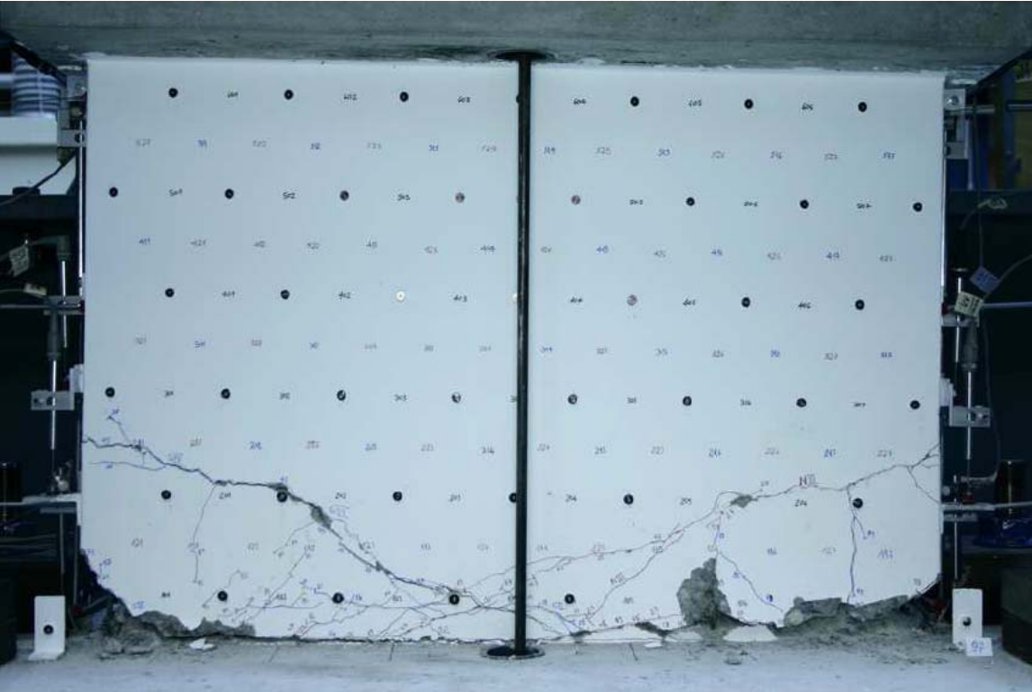
Figure C-95 Condition of wall M4 at -2.05% drift (2 nd cycle) [Greifenhagen et al. (2005)]
