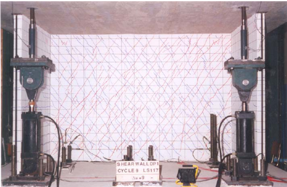
Figure C-297 Condition of wall DP1 at 0.45% drift [Palermo and Vecchio (2002)]
