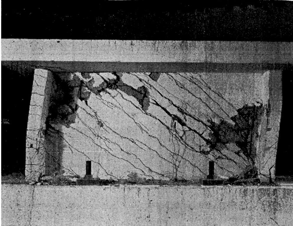
Figure C-265 Condition of wall B1-1 at the end of the test (drift > 8%) [Barda et al. (1977)]
