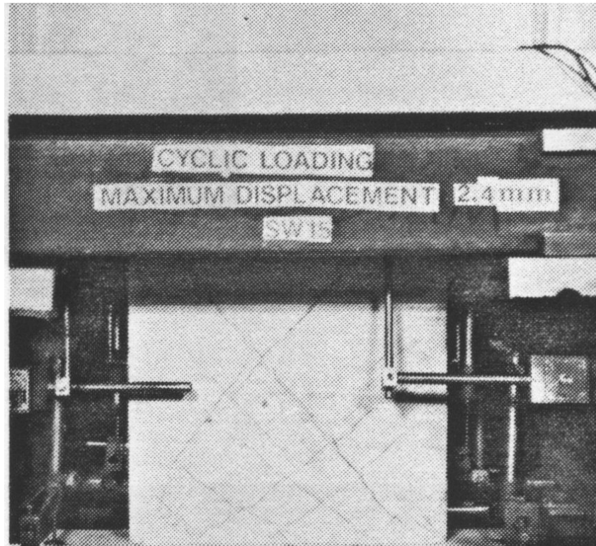
Figure C-131 Condition of wall SW15 at 0.48% drift [Lopes and Elnashai (1991)]
