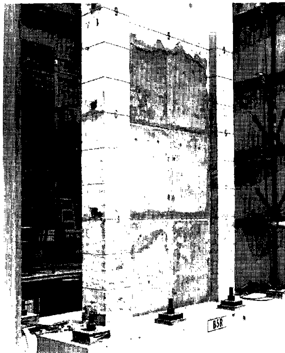
Fig. A-28 Specimen B5R After Completion of Repairs
