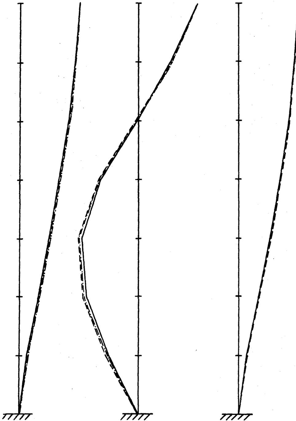
Fig. 10. Mode shapes for Example 3 ( — exact, ---- Timoshenko beam, -·-·- shear beam). The third mode is a longitudinal mode and the amplitude indicates vertical displacement.
