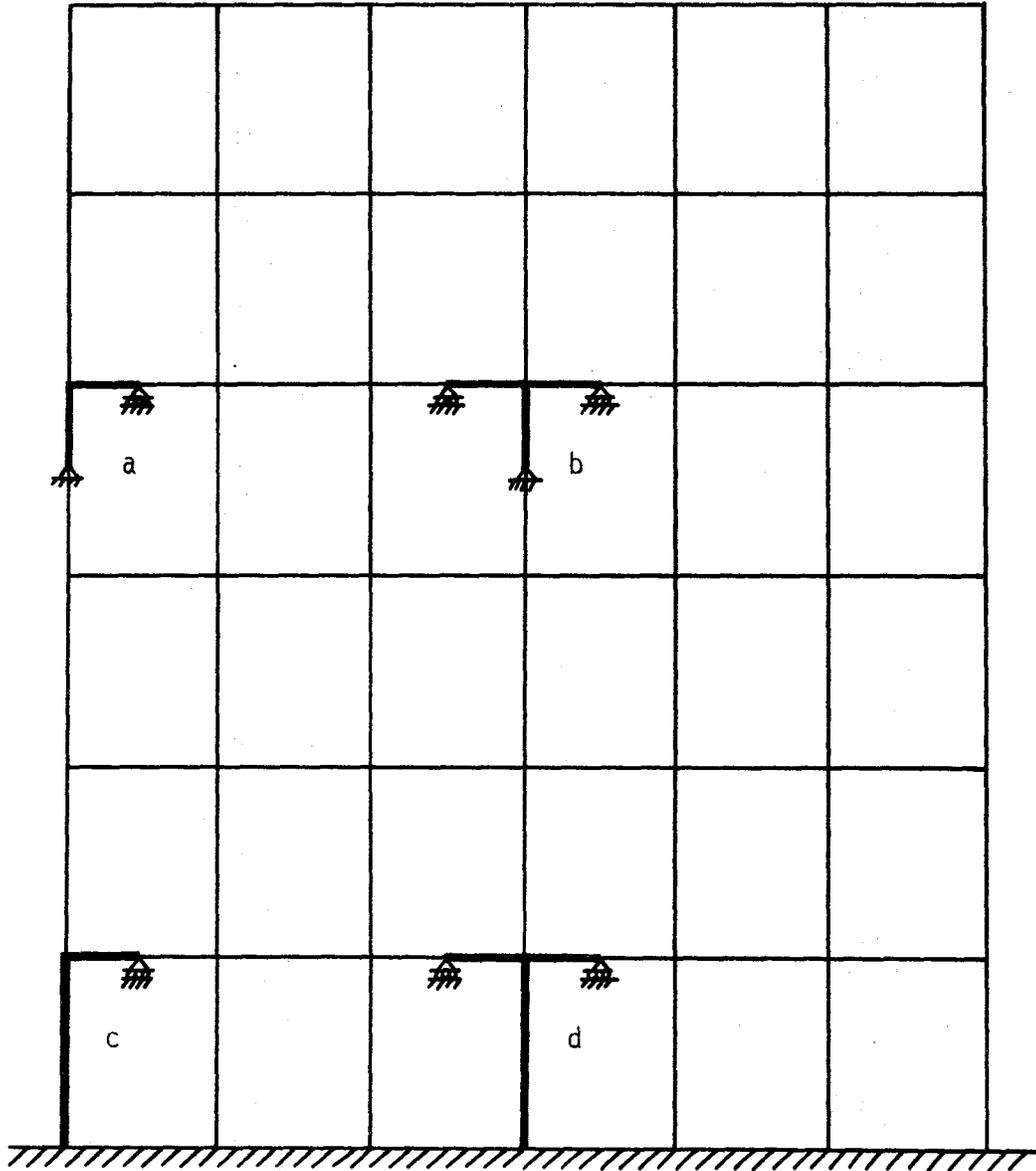
Fig. 1. Four types of substructures.
