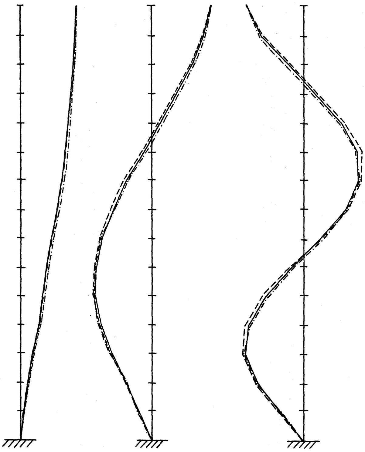
Fig. 8. Mode shapes for Example 2 ( — exact, ---- Timoshenko beam, - · - · - shear beam).
