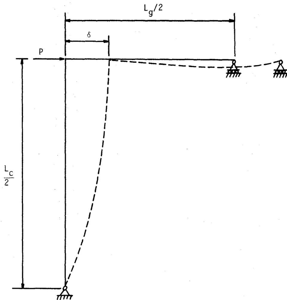
Fig. 2. Effective shear rigidity of Substructure Type a.
