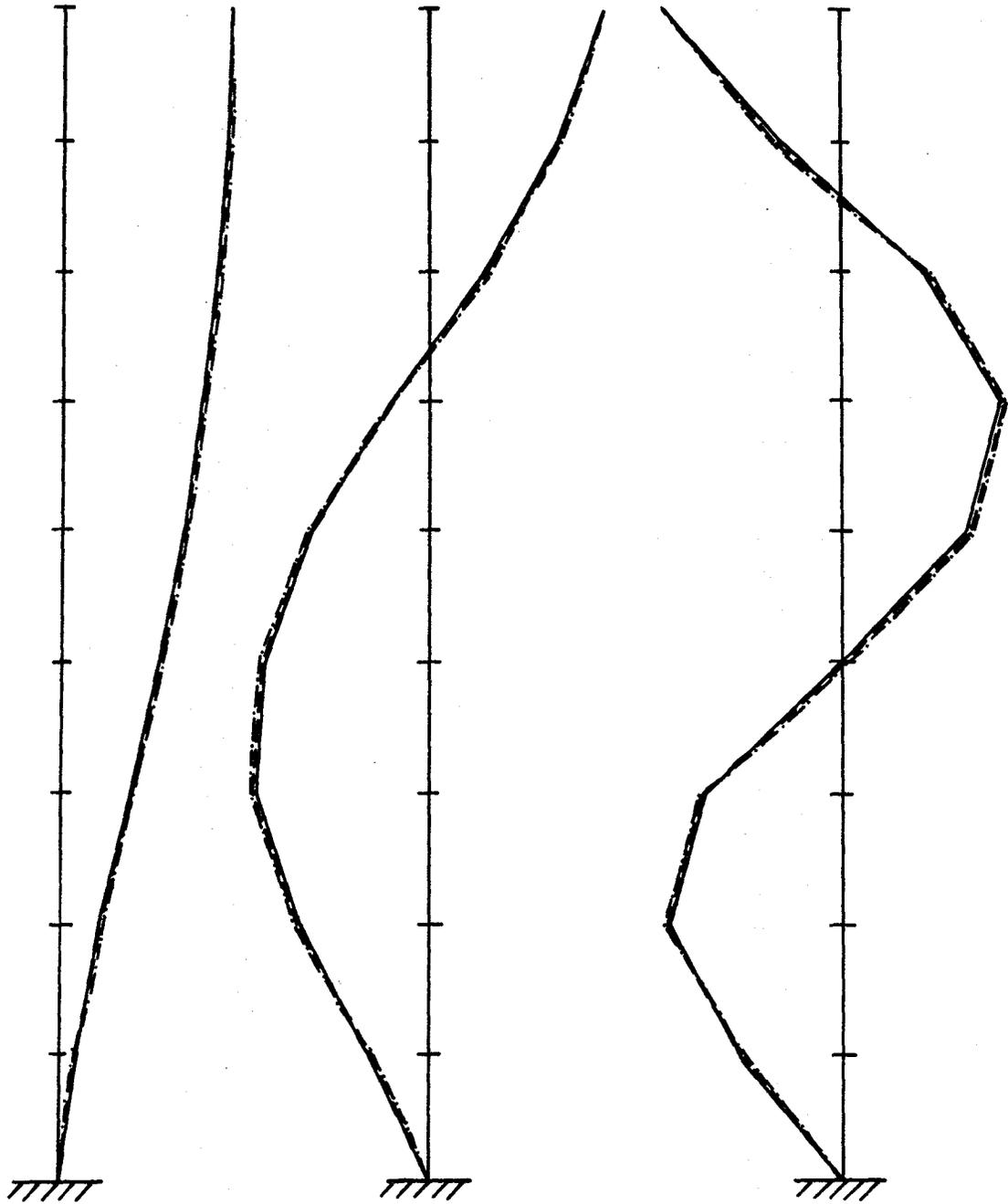
Fig. 6. Mode-shapes for Example 1 ( — exact, ---- Timoshenko beam, -.-.- Shear beam).
