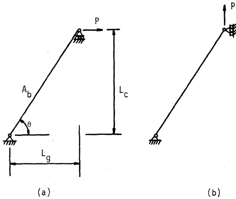
Fig. 4. Effective shear and bending stiffness of a brace.
