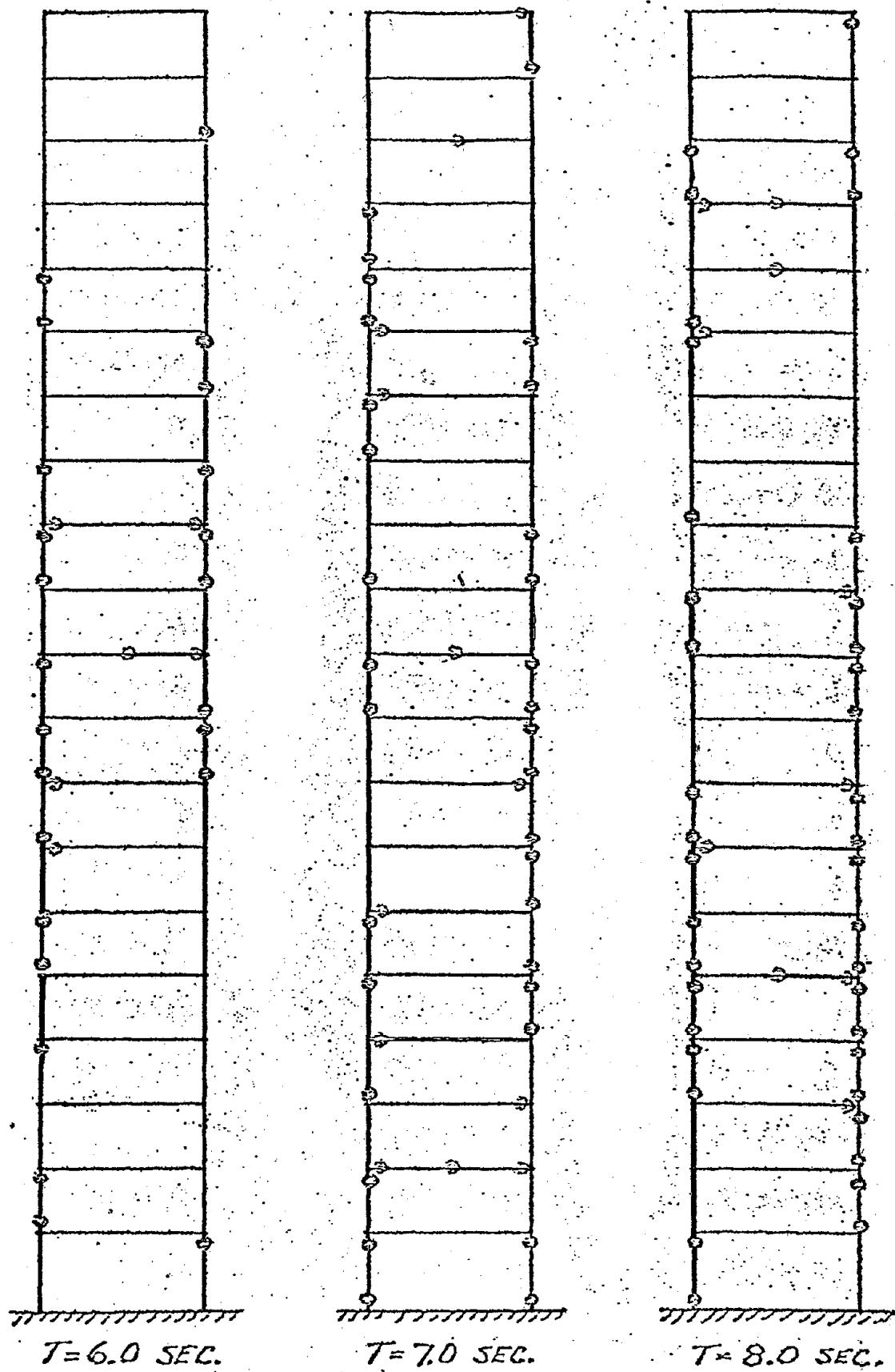
Fig. 4-67 Plastic Hinge Location, MWD Frame
