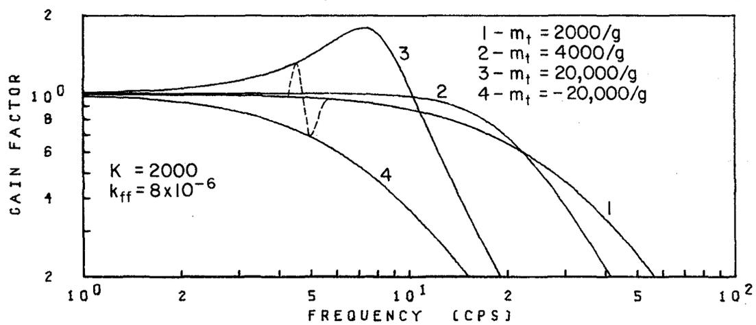
FIG. 3.9 COMPUTED FREQUENCY RESPONSES FOR DIFFERENT EFFECTIVE TABLE MASSES
