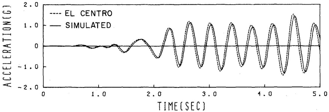
(b) Response of linear structure to El Centro and simulated El Centro motion
