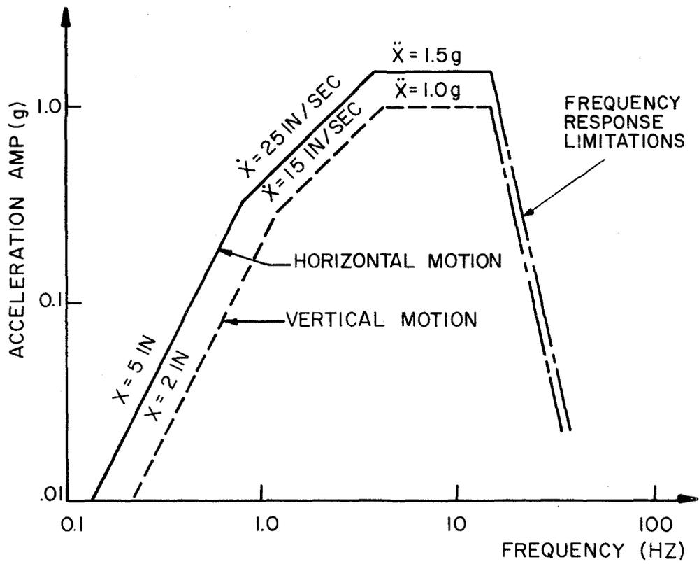
FIG. 1.1 LIMITATIONS ON THE DYNAMIC PERFORMANCE OF A PARTICULAR SHAKING TABLE
