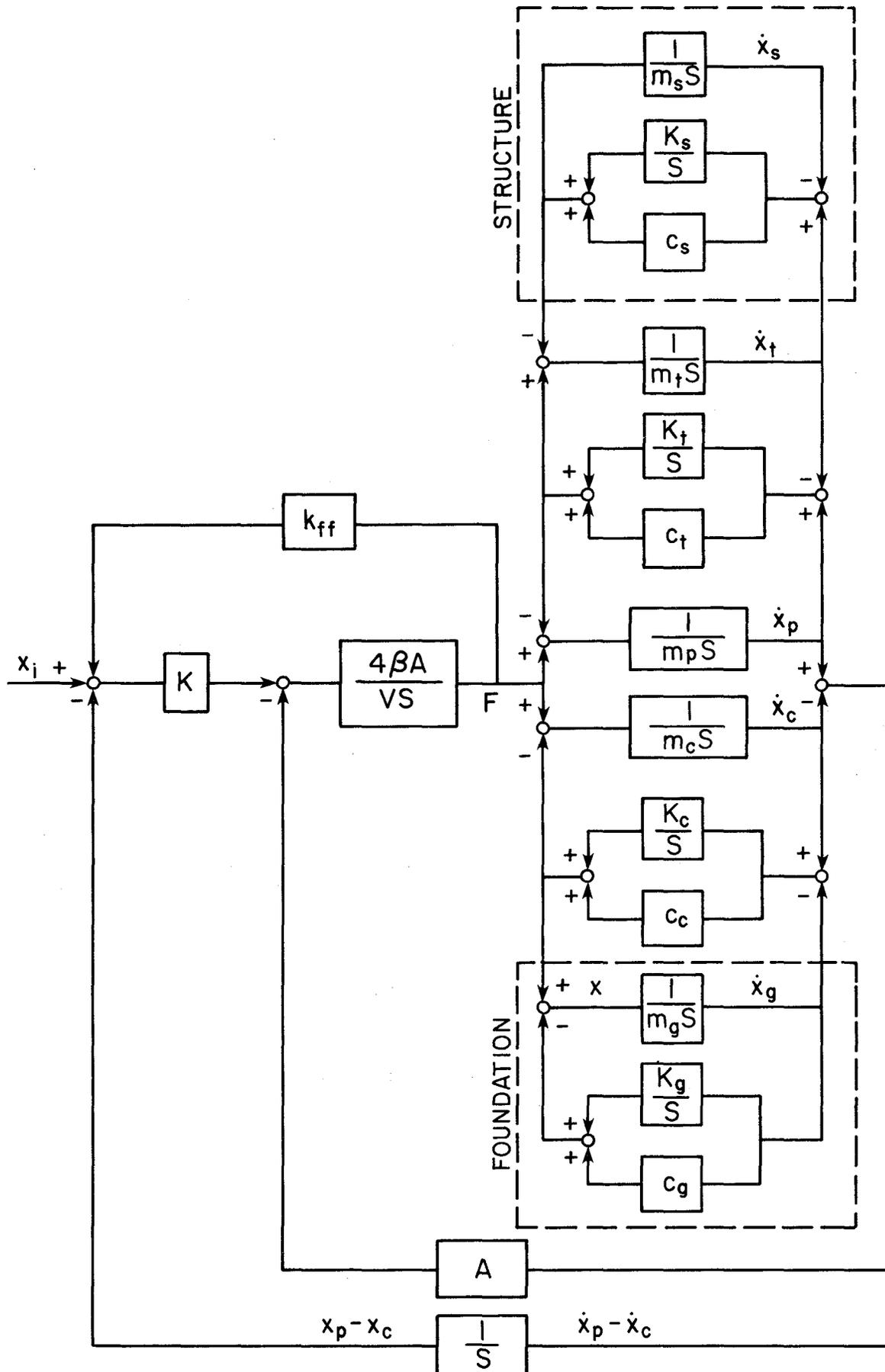
FIG. 3.12 SHAKING TABLE WITH FLEXIBLY COUPLED STRUCTURE AND FOUNDATION
