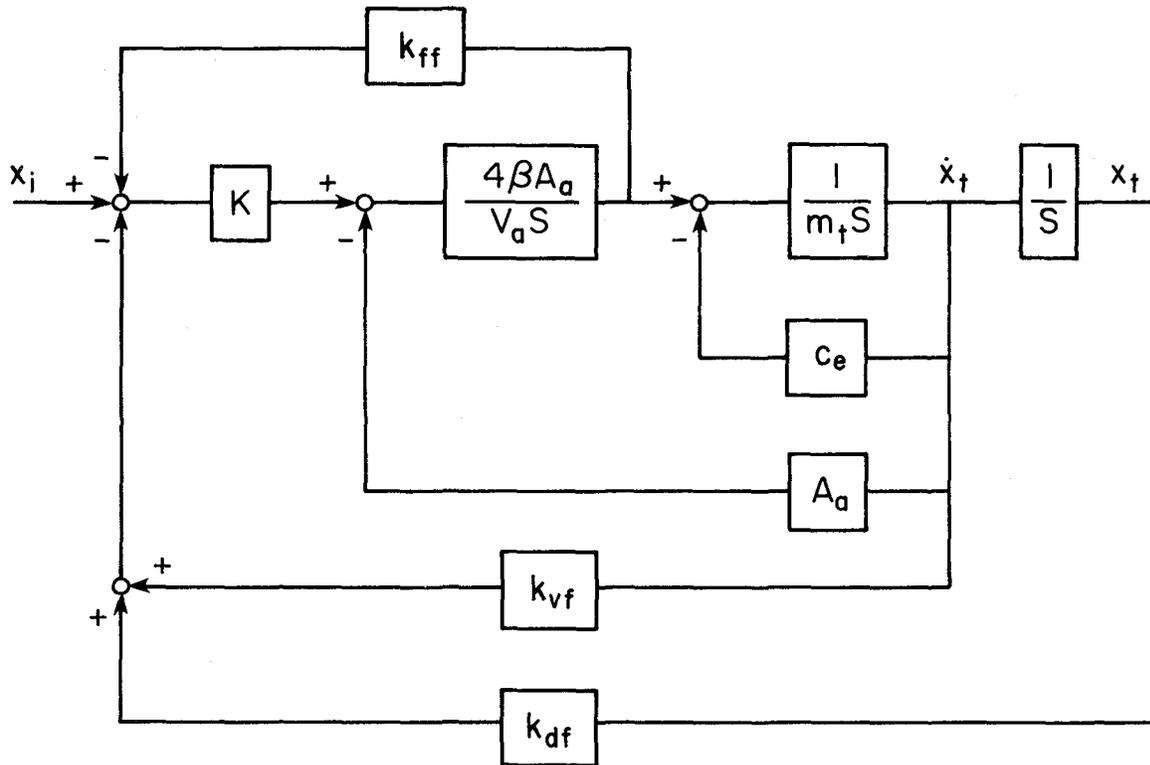
FIG. 3.4 SHAKING TABLE CLOSED LOOP CONTROL SYSTEM
