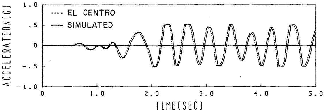
(c) Response of nonlinear structure to El Centro and simulated El Centro motion
