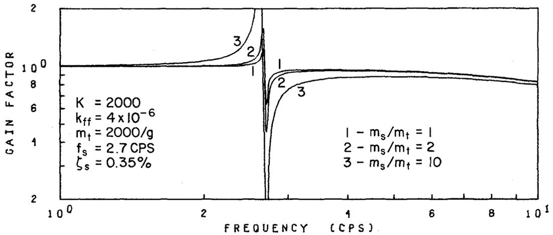
(b) Effects of varying ratio of structure and table masses
