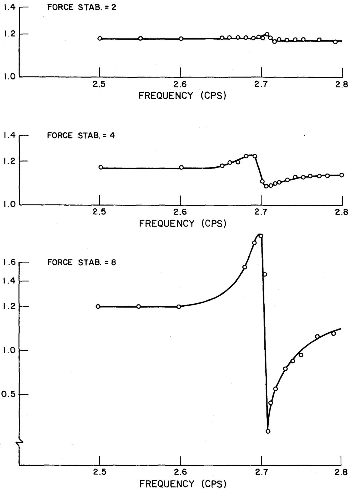
FIG. 2.5 FREQUENCY RESPONSES OF 2000 lb TABLE WITH RESONANT STRUCTURE AND VARYING AMOUNTS OF FORCE FEEDBACK
