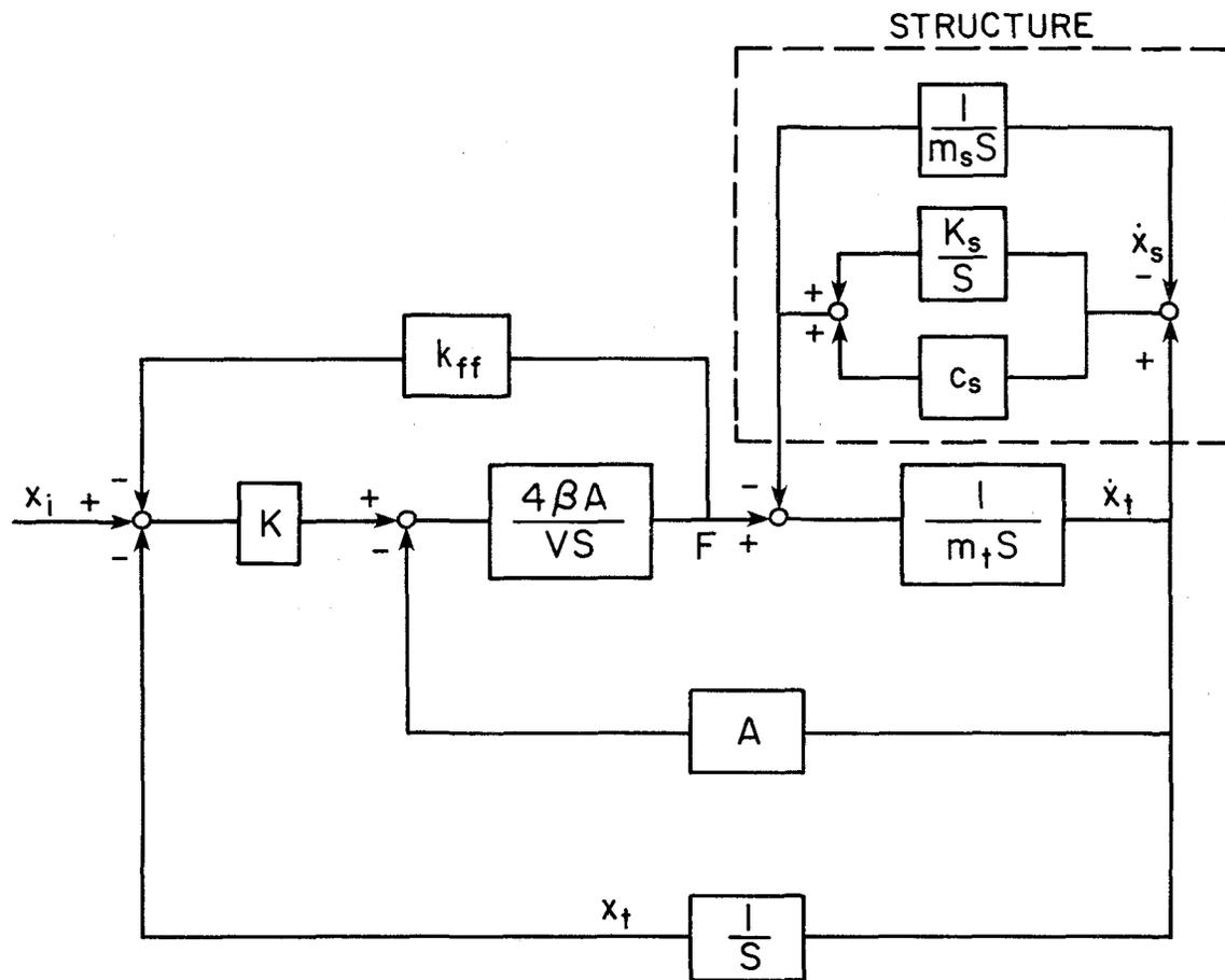
FIG. 3.7 SHAKING TABLE WITH STRUCTURE
