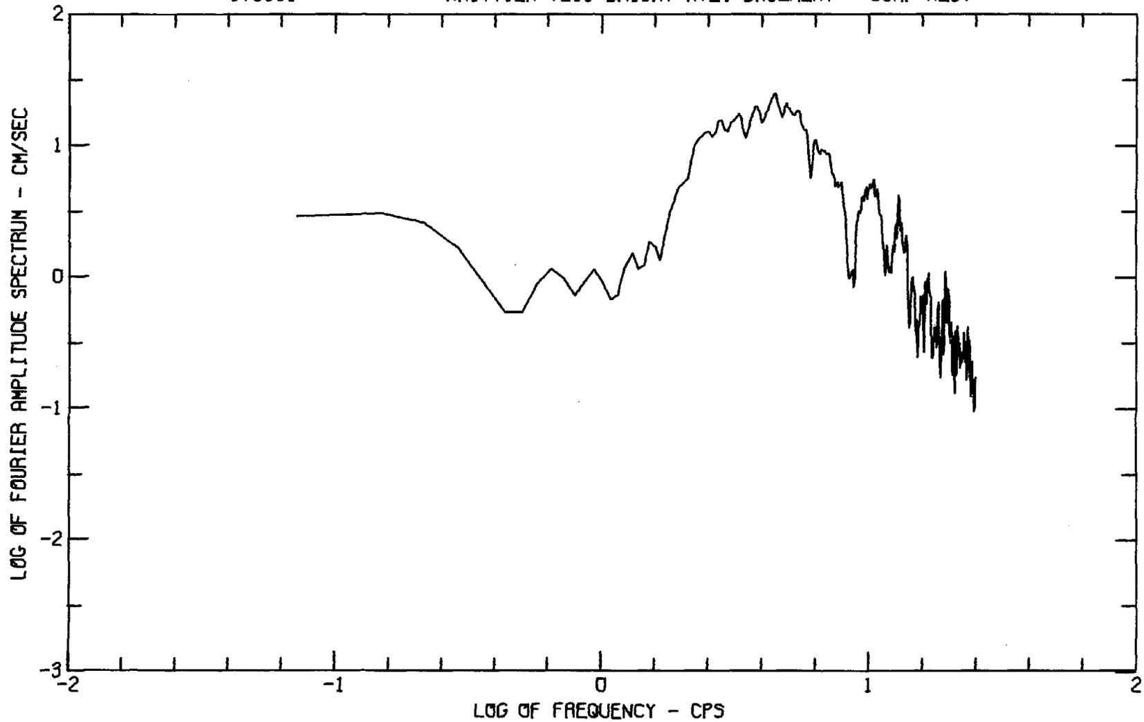
FOURIER AMPLITUDE SPECTRUM OF ACCELERATION
