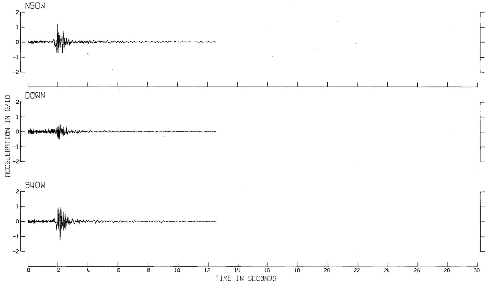
Fig. 35-b Uncorrected Accelerograms (Left Abutment)
