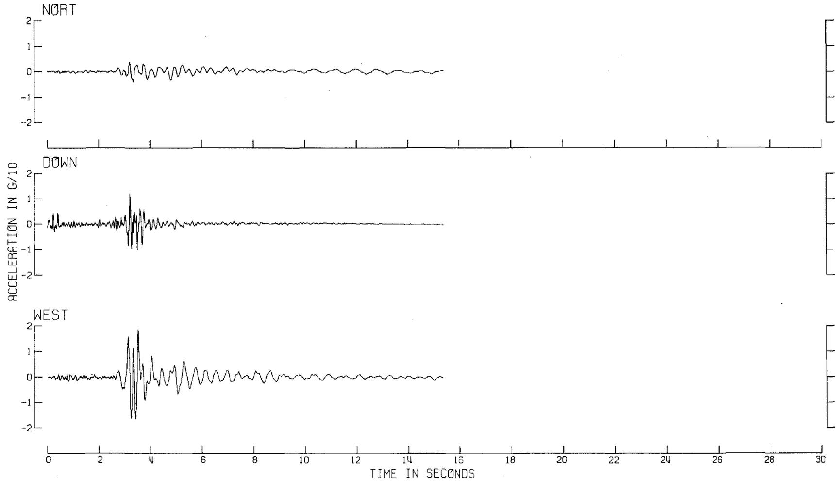
Fig. 6-c Uncorrected Accelerograms (10th Floor)
