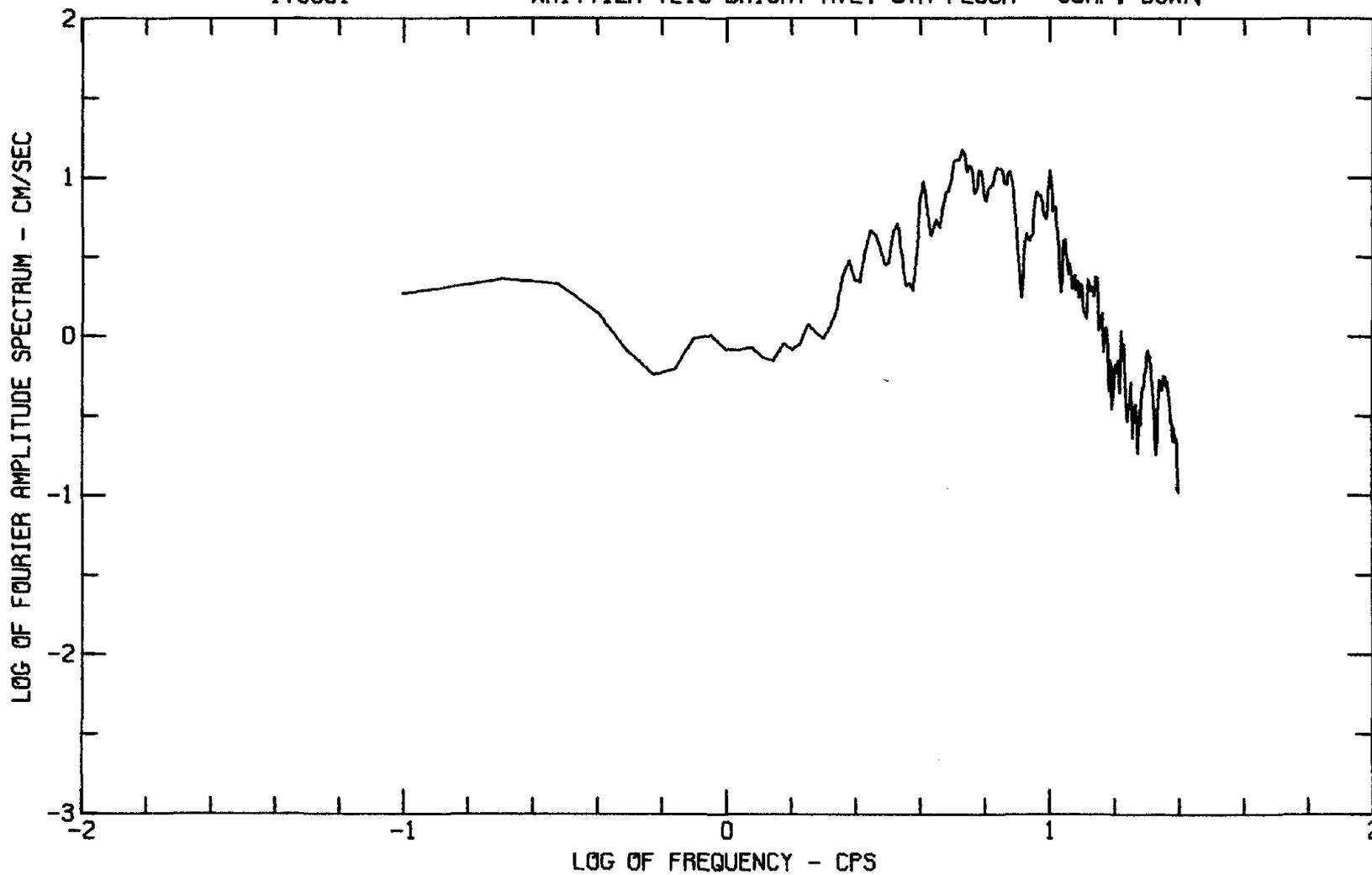
FOURIER AMPLITUDE SPECTRUM OF ACCELERATION
