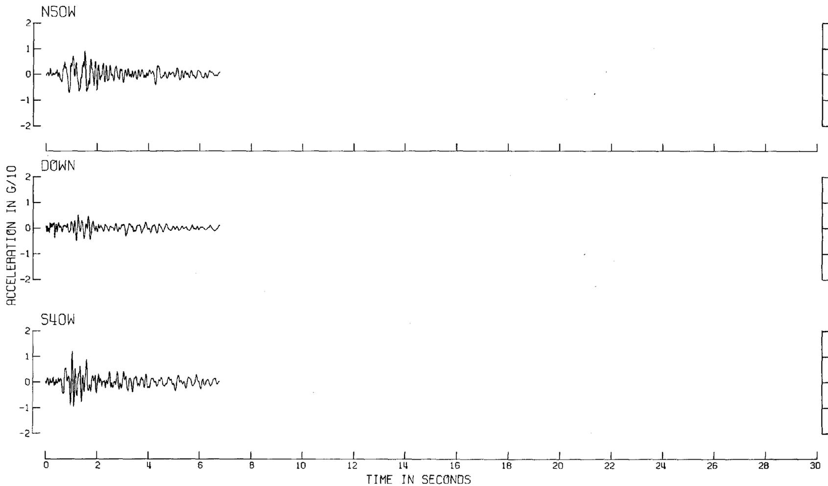
Fig. 64-b Uncorrected Accelerograms (Crest)
