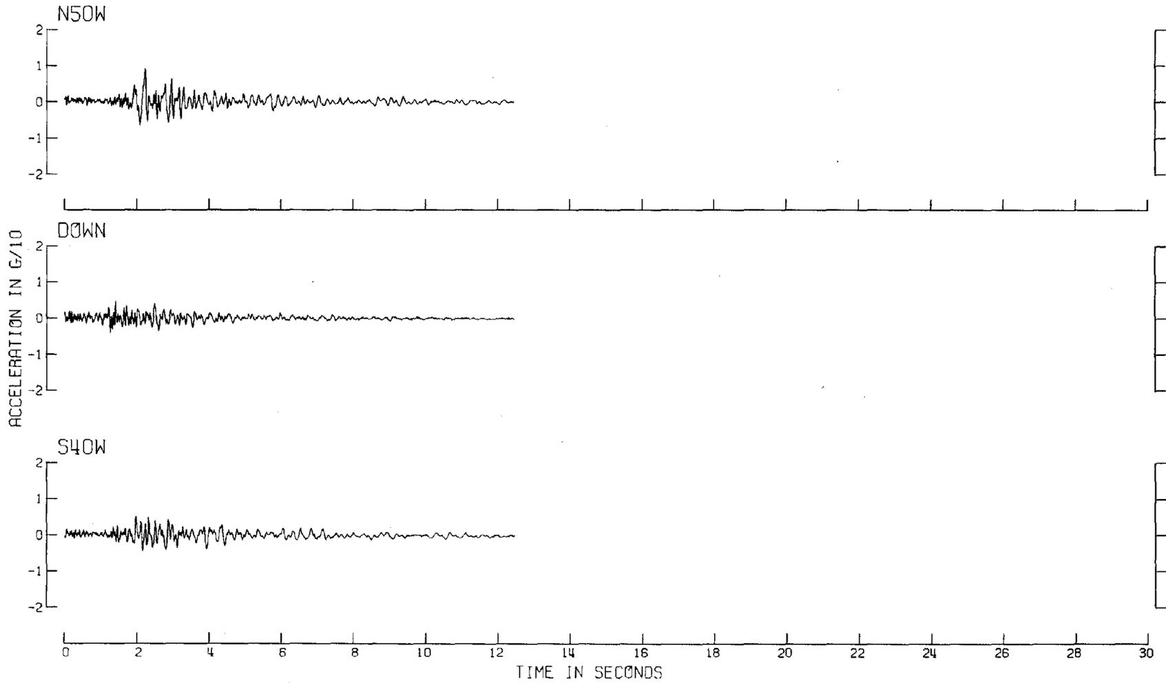
Fig. 64-a Uncorrected Accelerograms (Downstream)
