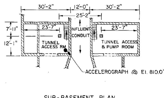
STRUCTURAL DETAILS OF THE HEADHOUSE (R. B. DIEMER FILTRATION PLANT)
