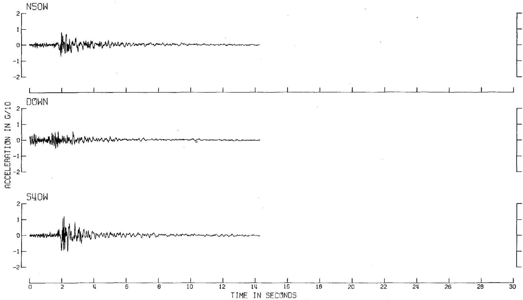
Fig. 35-c Uncorrected Accelerograms (Crest)
