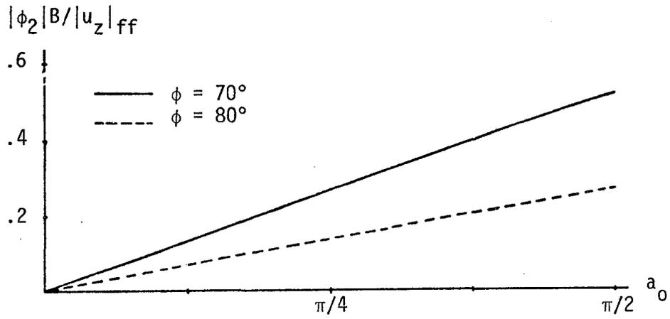
Figure 14 - Rocking Motion for SV-P Waves. Surface Foundations.
