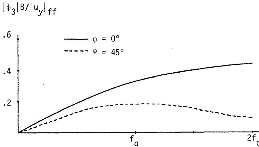
Figure 9 - Torsional Motion for SH Waves. Embedded Foundation.
