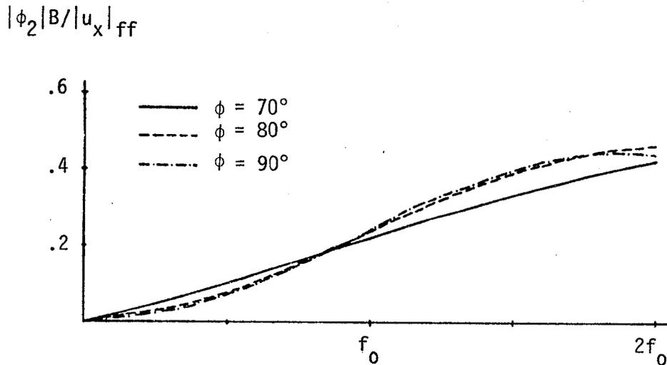
Figure 18 - Rocking Motion for SV-P Waves. Embedded Foundation.
