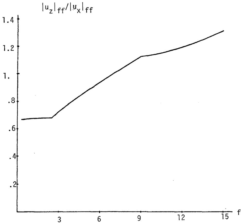
Figure 11 - Ratio of Amplitudes of Surface Motion for SV-P Waves.
