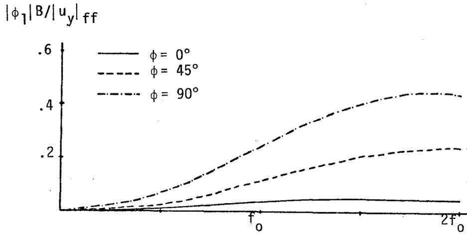
Figure 10 - Rocking Motion for SH Waves. Embedded Foundation.
