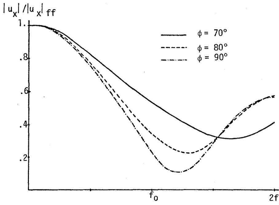
Figure 16 - Filtering of the Horizontal Motion for SV-P Waves.
