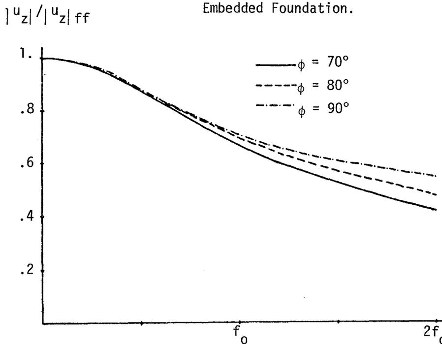
Figure 17 - Filtering of the Vertical Motion for SV-P Waves.
