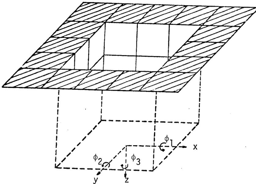
Figure 2 - Embedded Foundation
