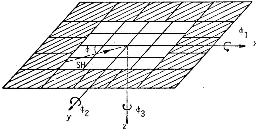
Figure 1 - Model for Surface Foundation and System of Coordinates
