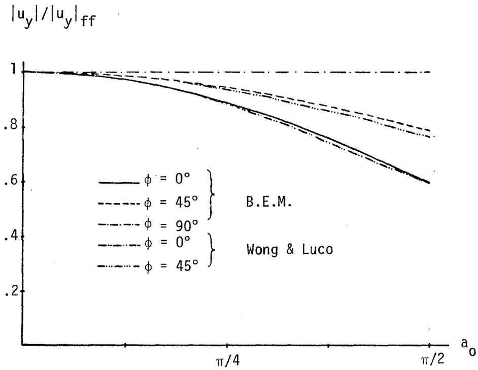
Figure 3 - Filtering of the Horizontal Motion for SH Waves.
