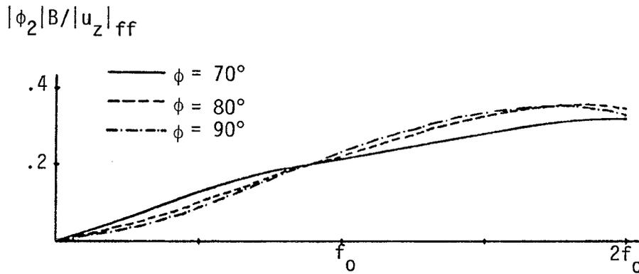
Figure 19 - Rocking Motion for SV-P Waves. Embedded Foundation.
