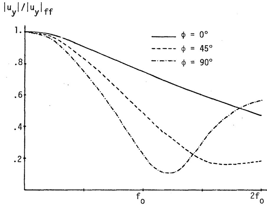
Figure 8 - Filtering of the Horizontal Motion for SH Waves.
