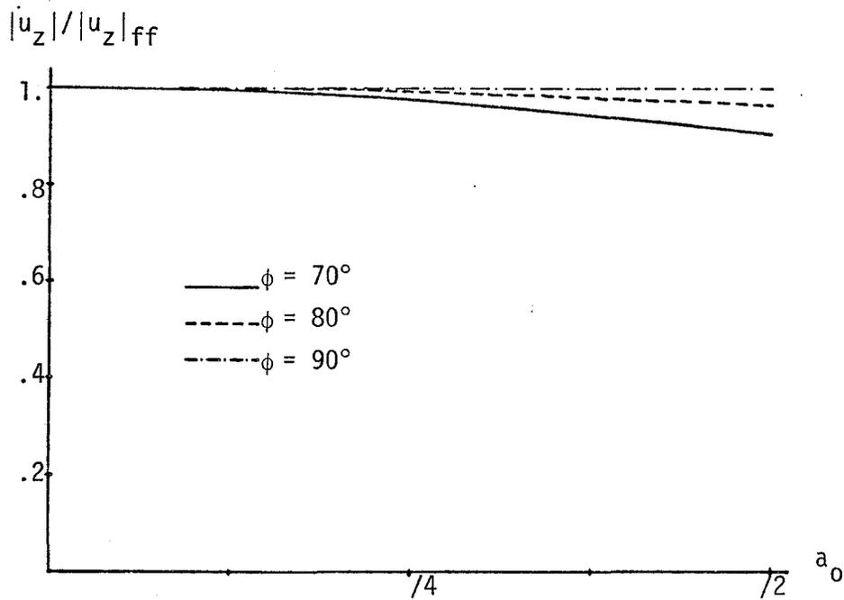
Figure 13 - Filtering of the Vertical Motion for SV-P Waves.
