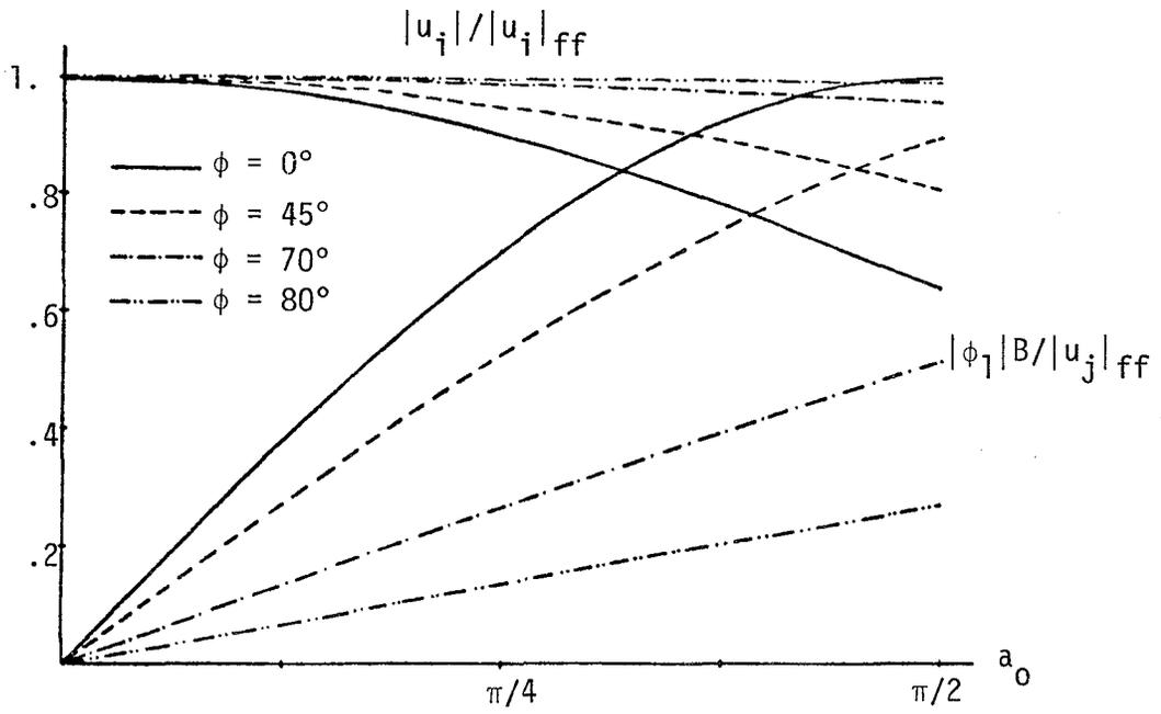
Figure 6 - Approximate Solution for the Filtering and Rotation by Unemori.
