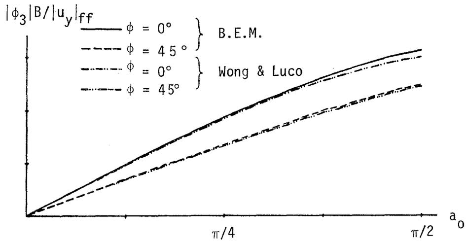
Figure 4 - Torsional Motion for SH Waves. Surface Foundation.
