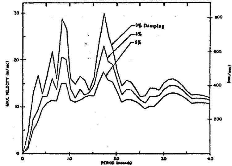
Fig. A2 Velocity Response Spectrum
