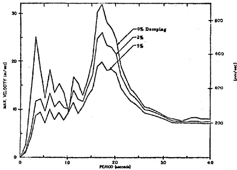
Fig. A7 Velocity Response Spectrum
