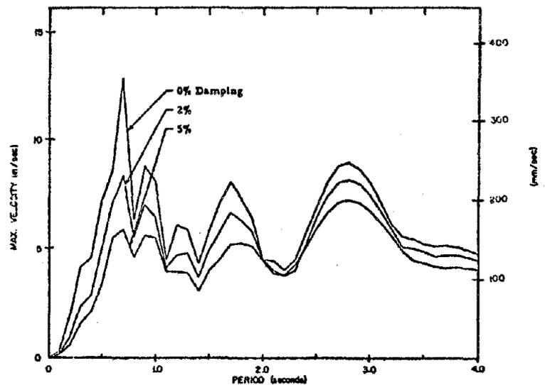
Fig. A8 Velocity Response Spectrum
