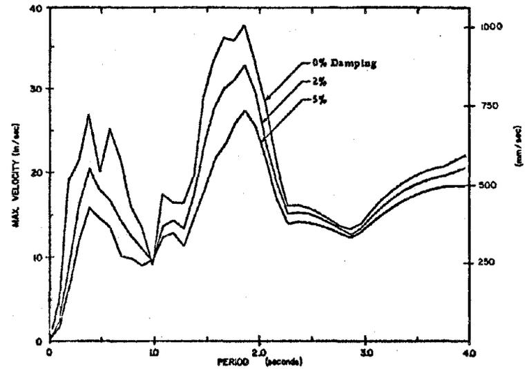
Fig. A6 Velocity Response Spectrum
