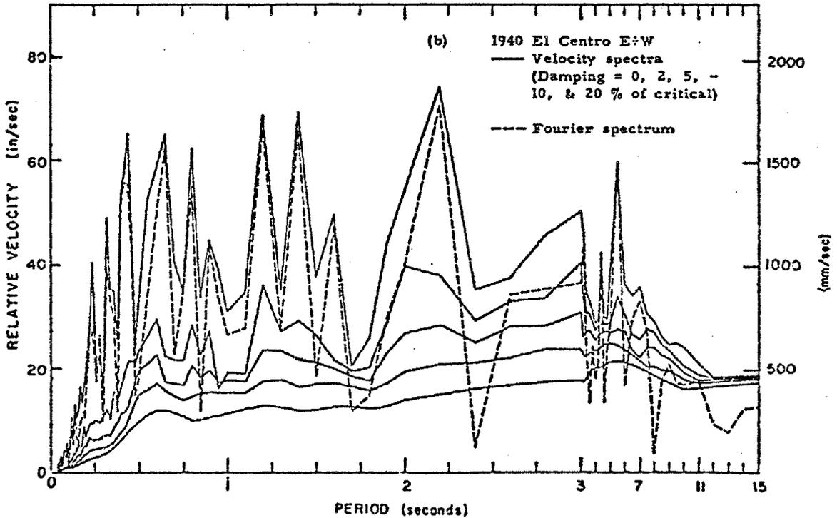
Fig. 3 Relative Velocity Response Spectra - 1940 El Centro Record
