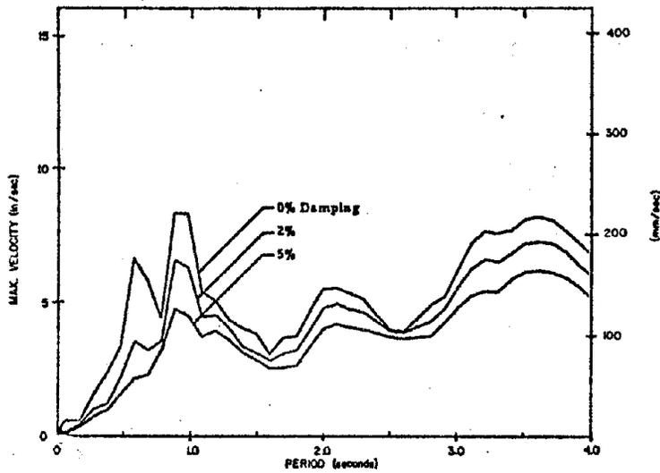
Fig. A41 Velocity Response Spectrum
