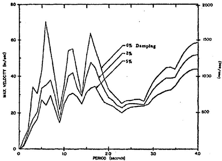
Fig. A39 Velocity Response Spectrum
