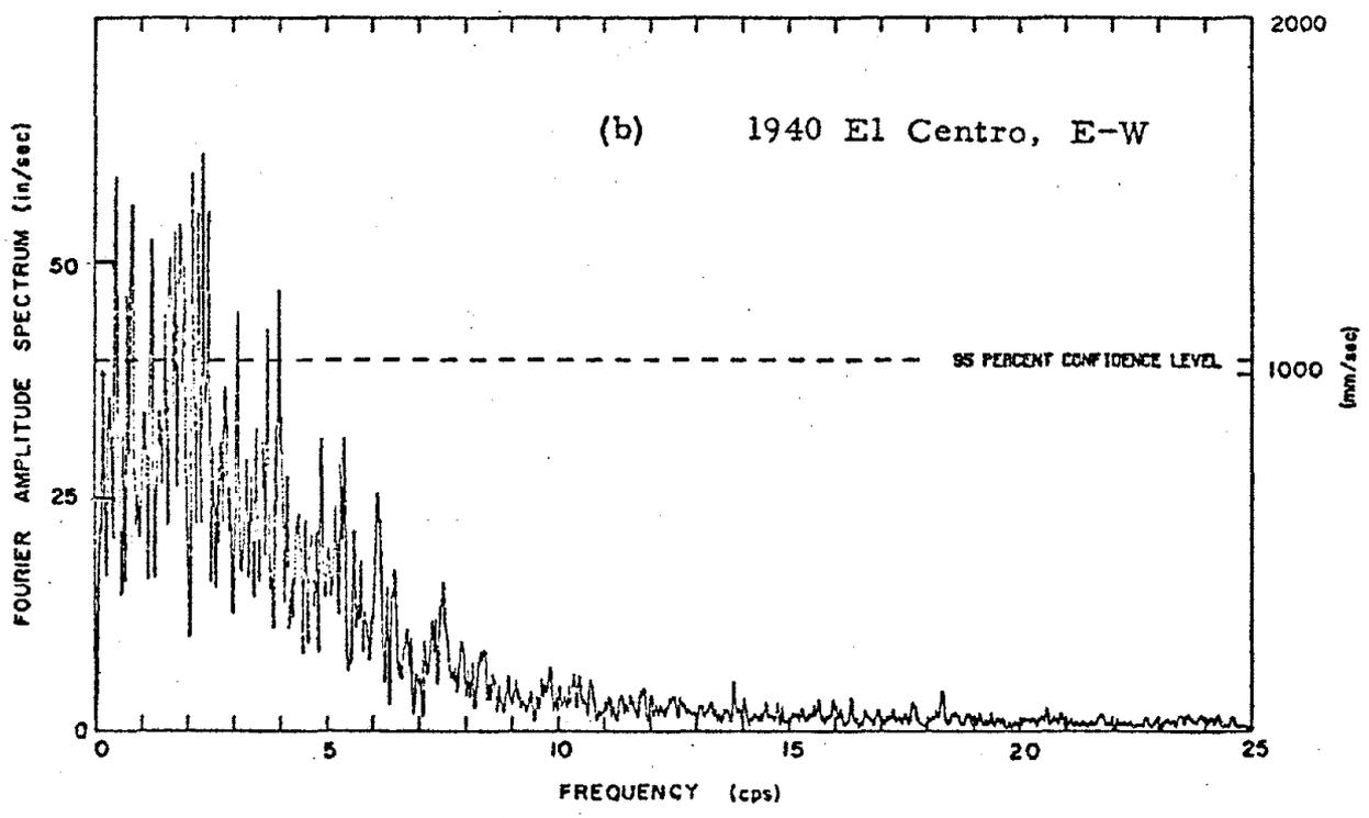
Fig. 2 Fourier Amplitude Spectrum - 1940 El Centro Record (from Ref. 19)
