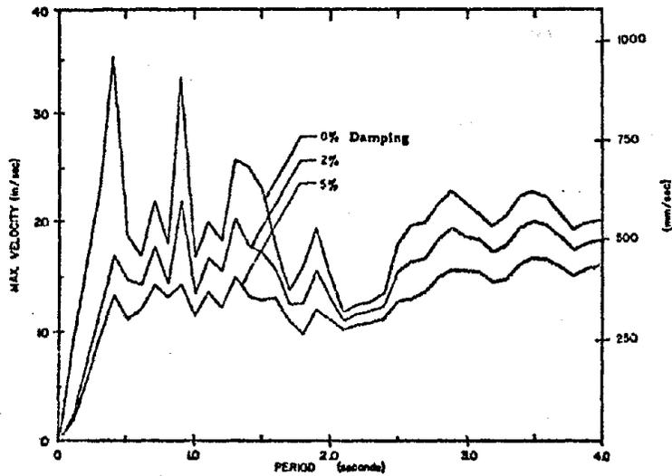
Fig. A35 Velocity Response Spectrum
