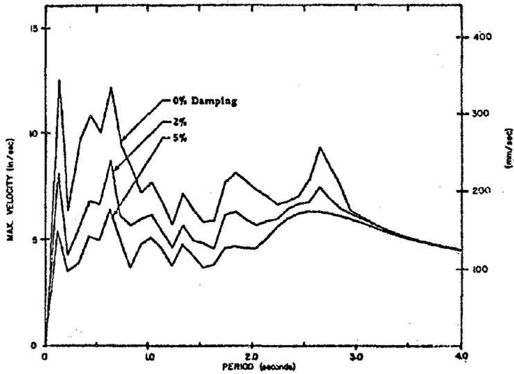
Fig. A5 Velocity Response Spectrum
