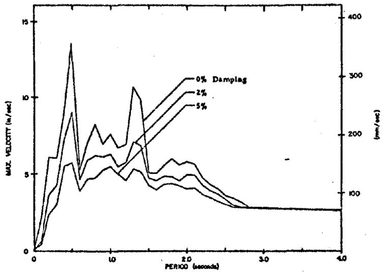
Fig. A31 Velocity Response Spectrum
