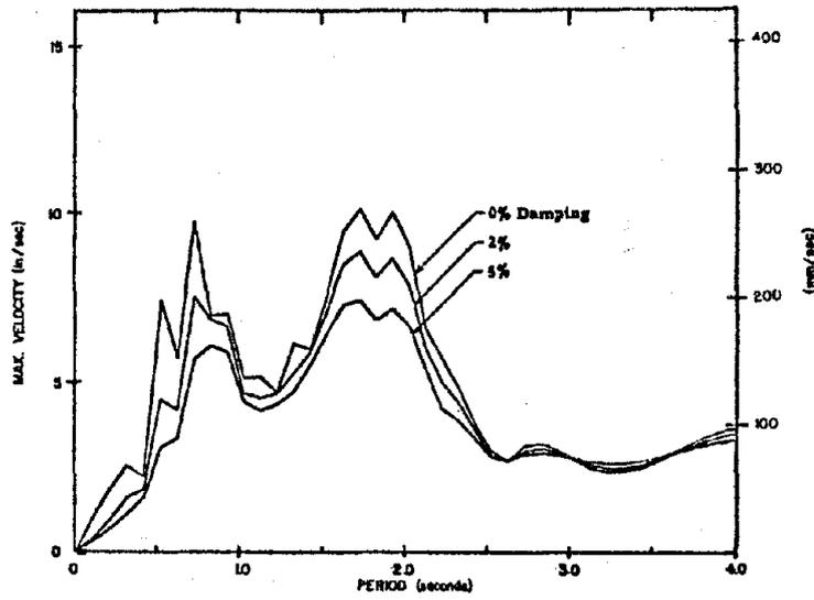
Fig. A17 Velocity Response Spectrum
