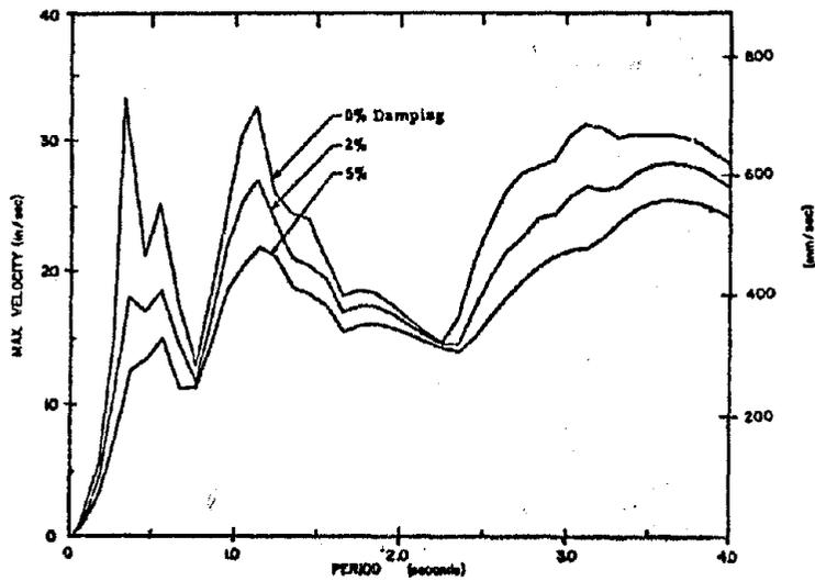
Fig. A11 Velocity Response Spectrum
