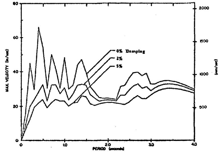
Fig. A32 Velocity Response Spectrum
