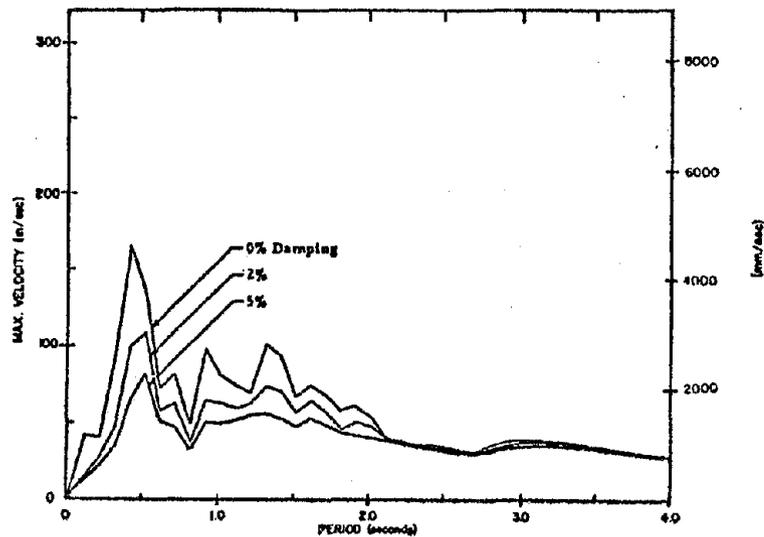
Fig. A3 Velocity Response Spectrum
