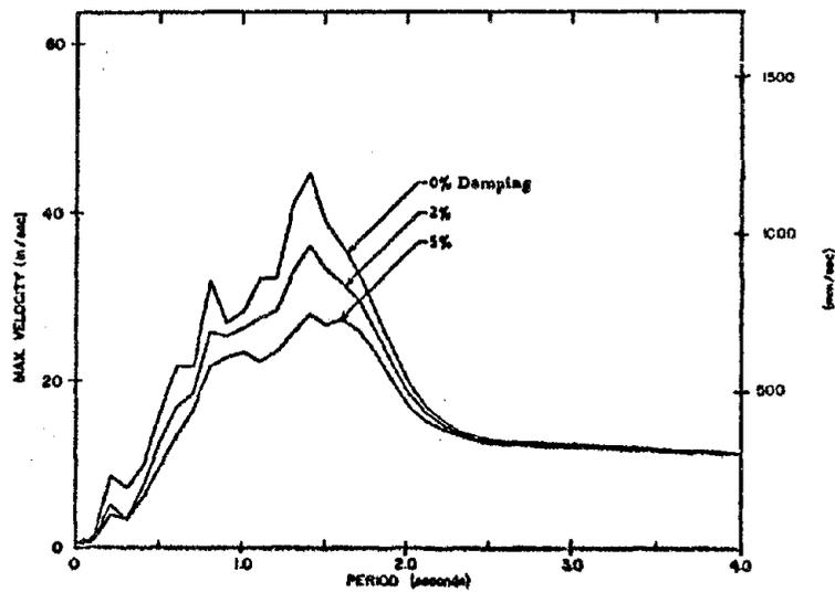
Fig. A16 Velocity Response Spectrum
