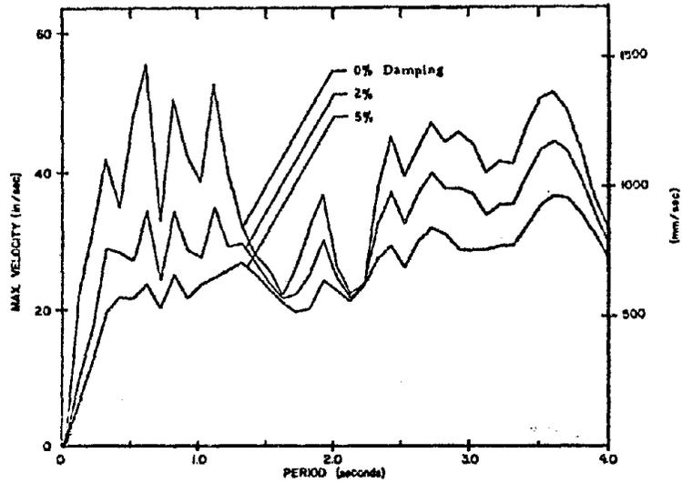
Fig. A33 Velocity Response Spectrum
