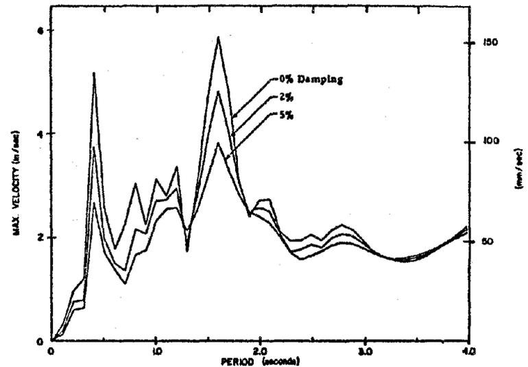
Fig. A22 Velocity Response Spectrum
