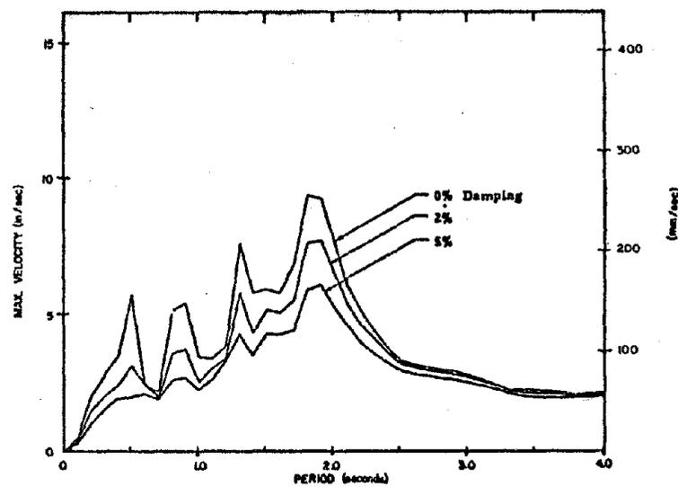
Fig. A26 Velocity Response Spectrum
