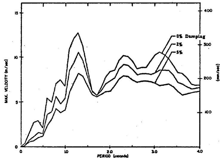
Fig. A42 Velocity Response Spectrum
