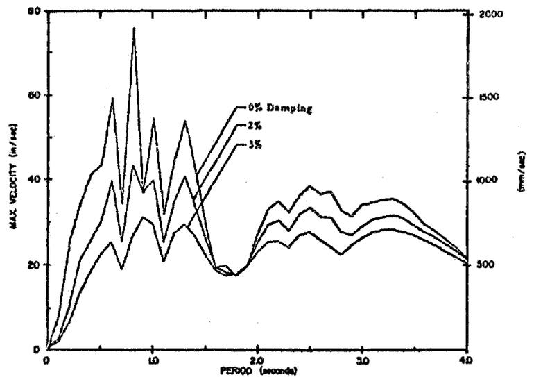
Fig. A40 Velocity Response Spectrum
