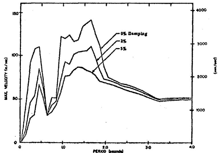
Fig. A4 Velocity Response Spectrum
