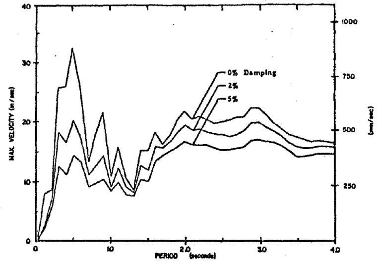
Fig. A34 Velocity Response Spectrum
