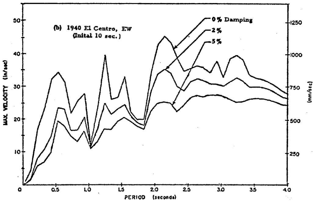
Fig. 4 Relative Velocity Response Spectra
