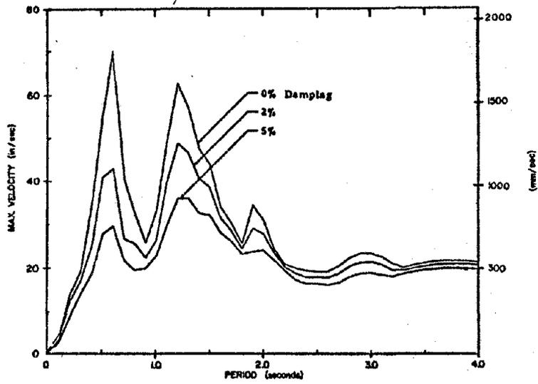
Fig. A29 Velocity Response Spectrum
