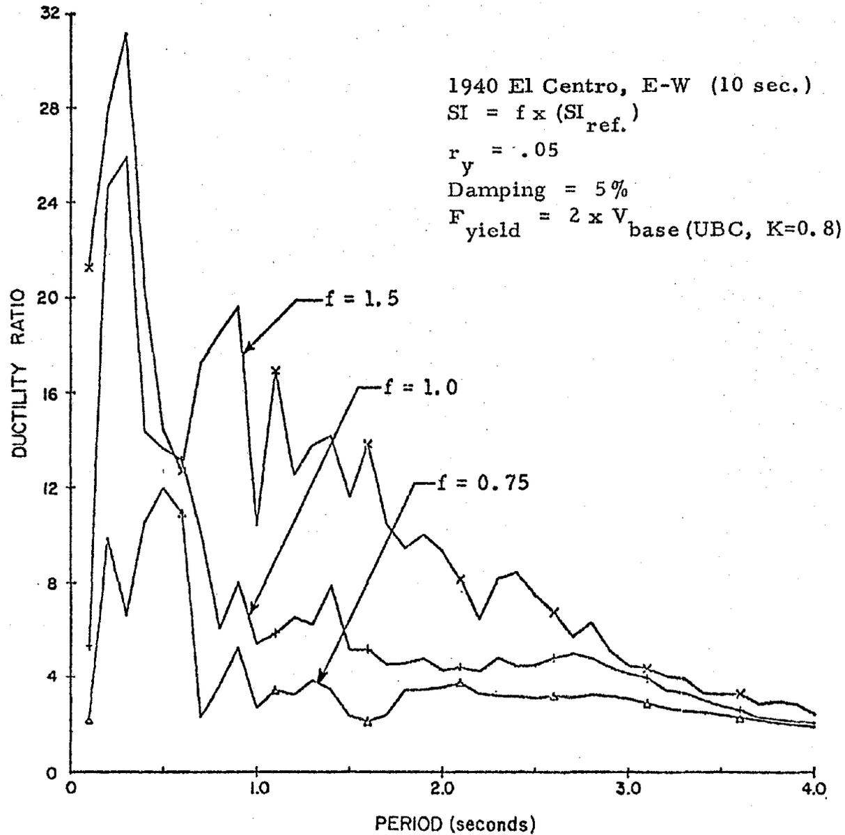
Fig. 9 Ductility Ratio versus Period for Bilinear Stable Hysteretic SDF Systems Subjected to Input Motions of Varying Intensity
