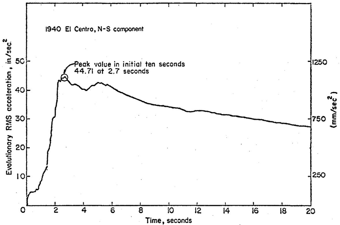
Fig. 6 Evolutionary RMS Acceleration versus Time
