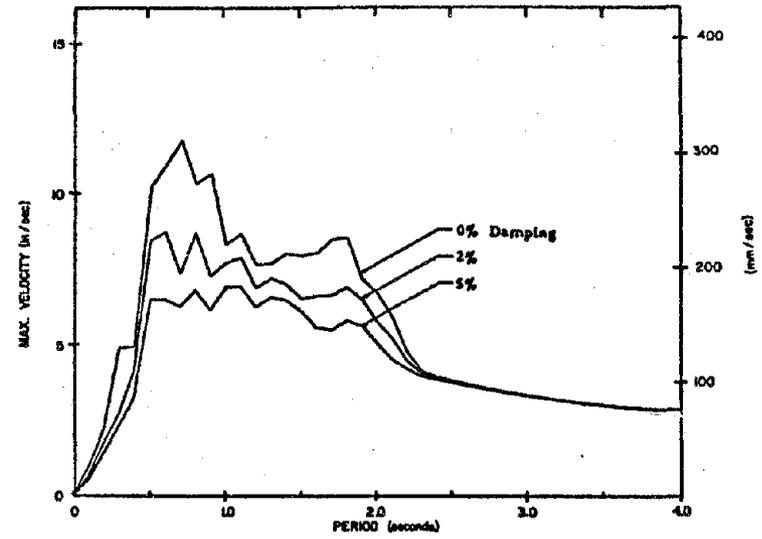
Fig. A30 Velocity Response Spectrum
