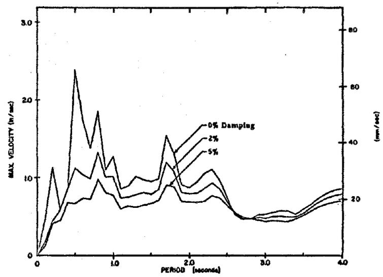
Fig. A14 Velocity Response Spectrum
