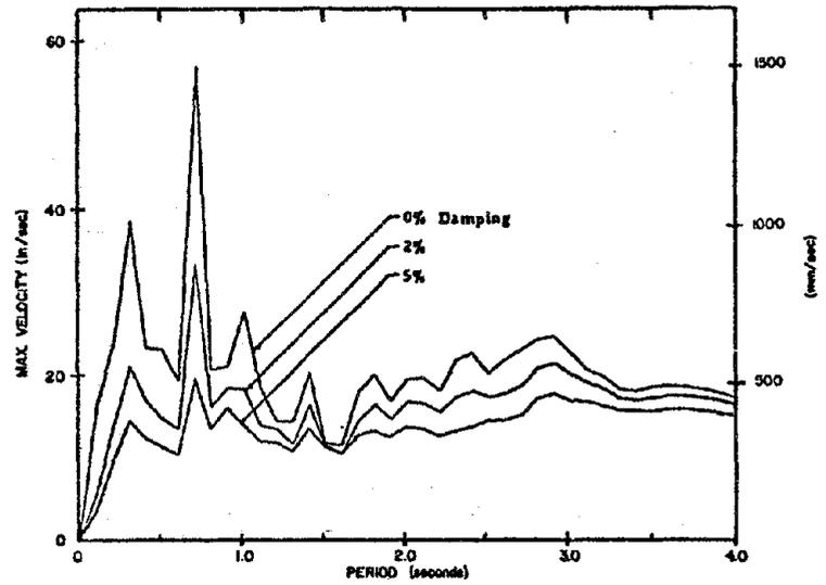
Fig. A38 Velocity Response Spectrum
