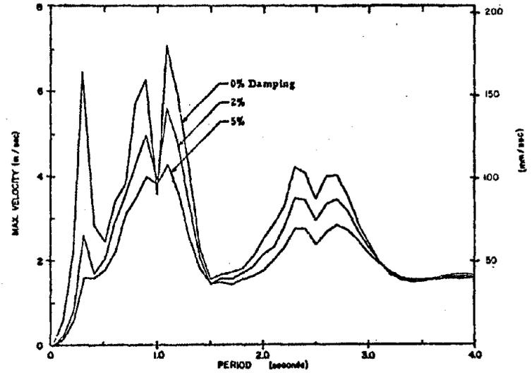
Fig. A10 Velocity Response Spectrum
