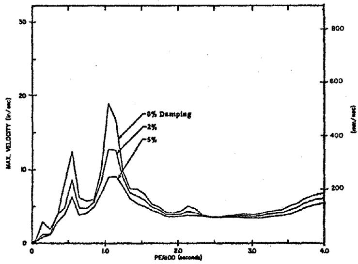
Fig. A13 Velocity Response Spectrum
