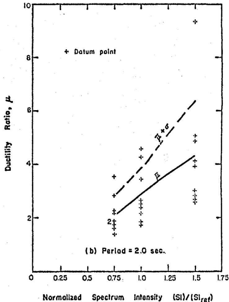
Fig. 11 Ductility Ratio versus Spectrum Intensity for Nine Input Motions
