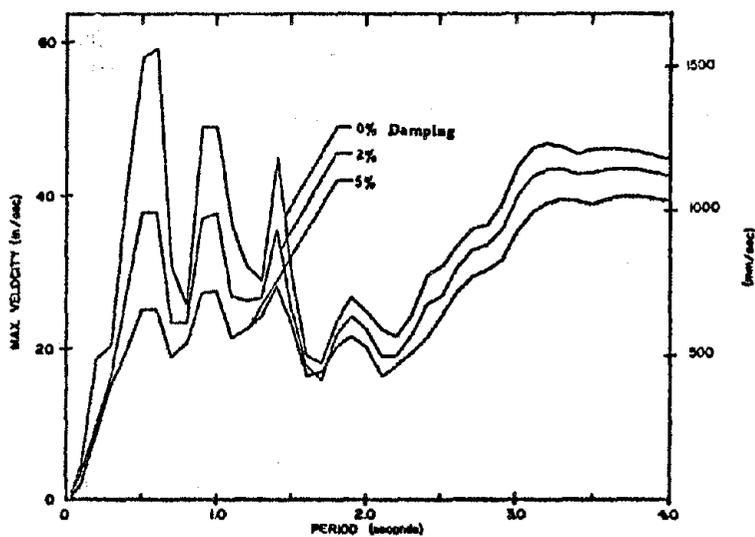
Fig. A28 Velocity Response Spectrum
