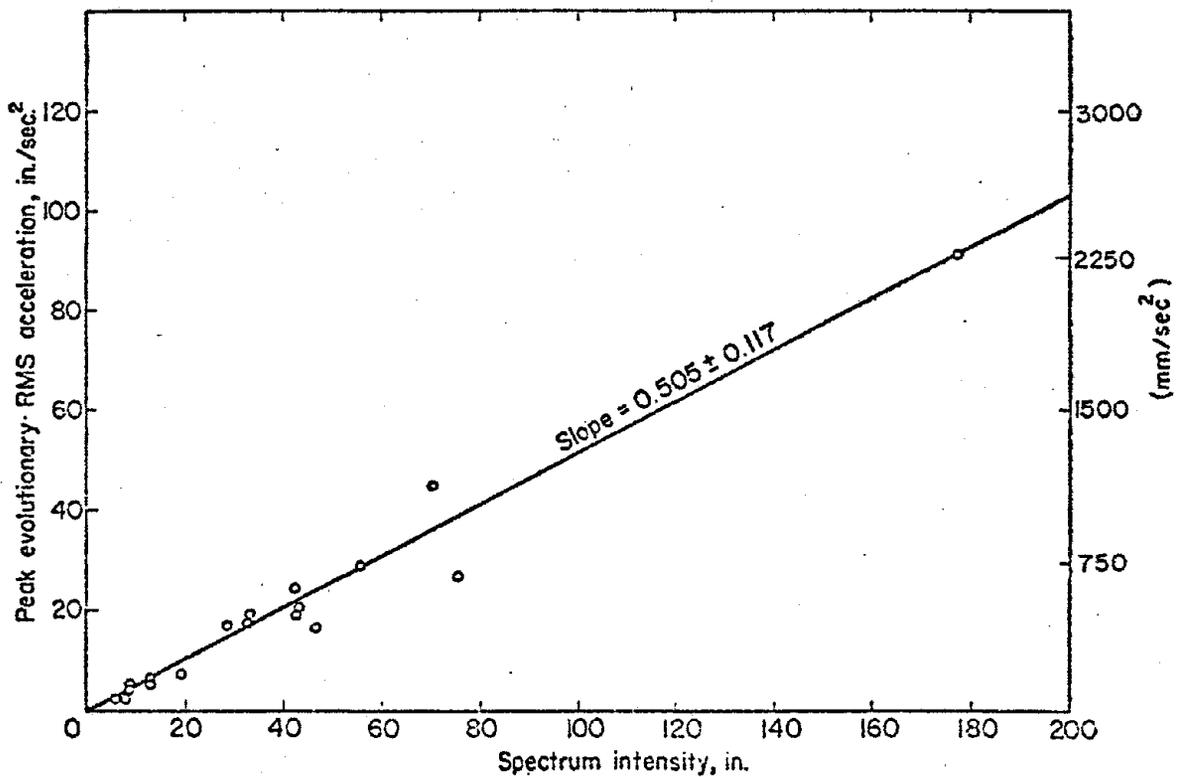
Fig. 7 Peak Evolutionary RMS Acceleration in First 10 Seconds vs. Spectrum Intensity for First 10 Seconds
