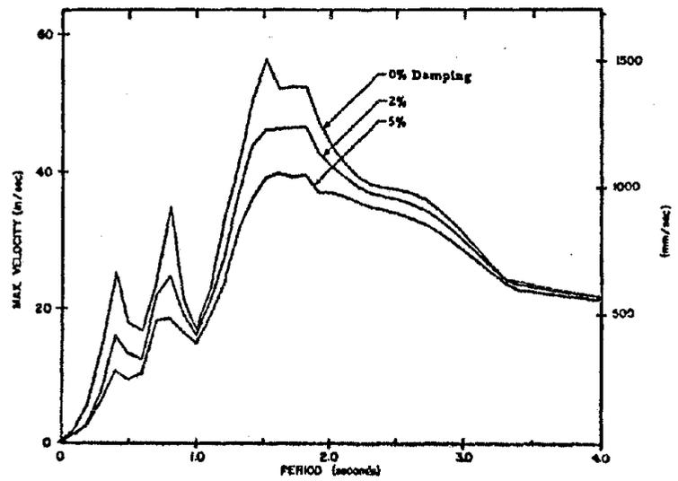
Fig. A15 Velocity Response Spectrum
