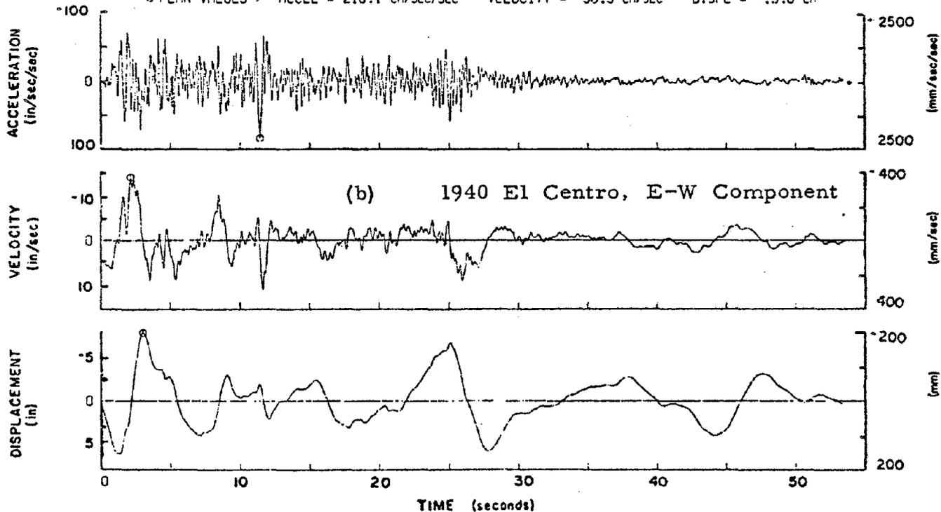
Fig. 1 Acceleration, Velocity and Displacement Histories
