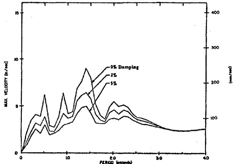
Fig. A24 Velocity Response Spectrum
