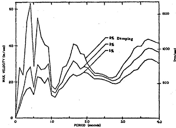
Fig. A37 Velocity Response Spectrum
