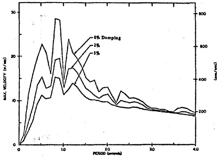
Fig. A1 Velocity Response Spectrum
