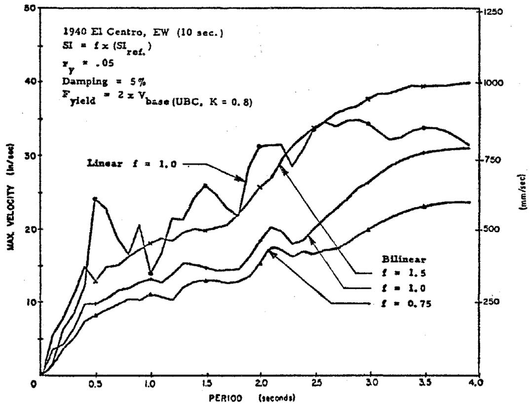
Fig. 8 Velocity Response Spectra for Linear and Bilinear Stable Hysteretic SDF Systems Subjected to Input Motions of Varying Intensity
