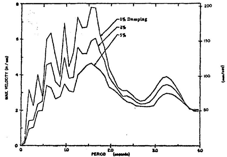
Fig. A12 Velocity Response Spectrum
