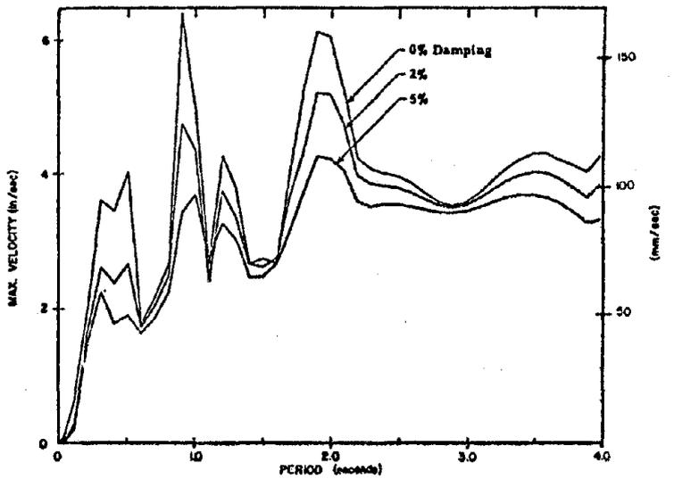
Fig. A20 Velocity Response Spectrum
