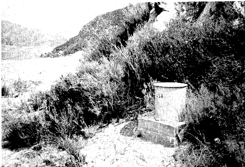
Fig. 6 East (left) abutment seismoscope
