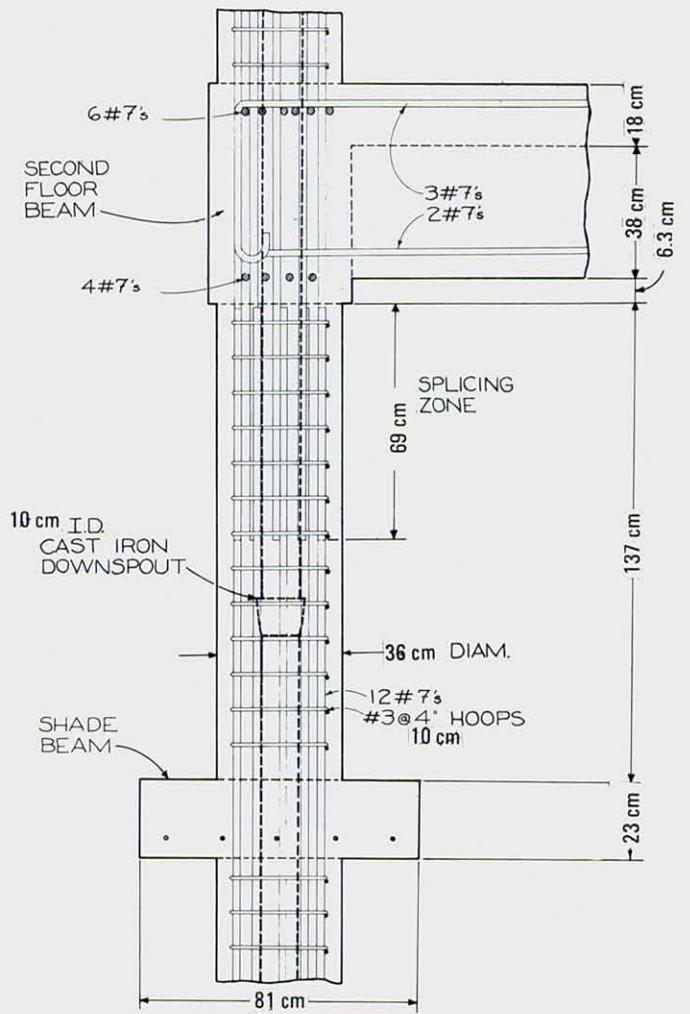
Figure 47. Column Splice and Joint Details
