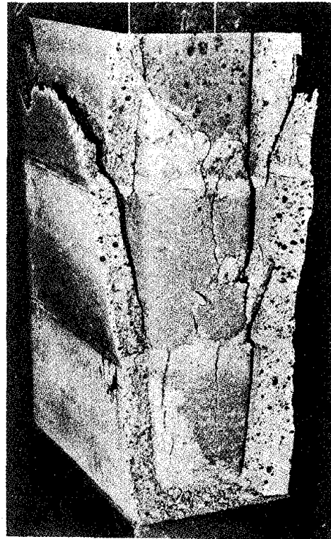
Fig. 6. Grout Core Tensile-Splitting
