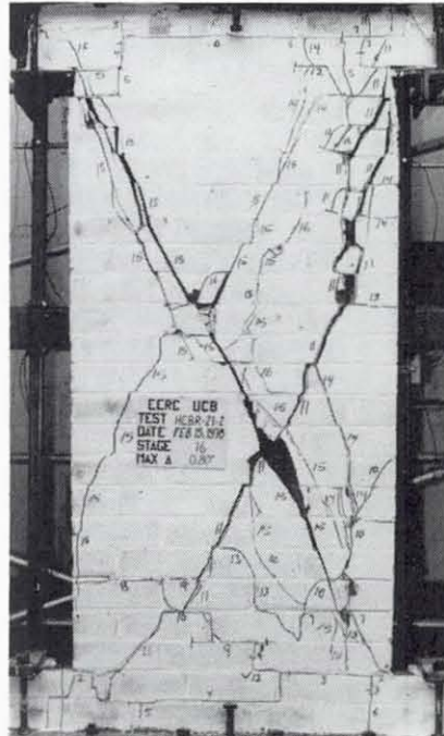
FIG. A.2 SUCCESSIVE CRACK FORMATION AND EXPERIMENTAL RESULTS TEST HCBR-21-2
