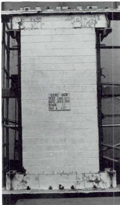
FIG. A.10 SUCCESSIVE CRACK FORMATION AND EXPERIMENTAL RESULTS TEST CBRC-21-1
