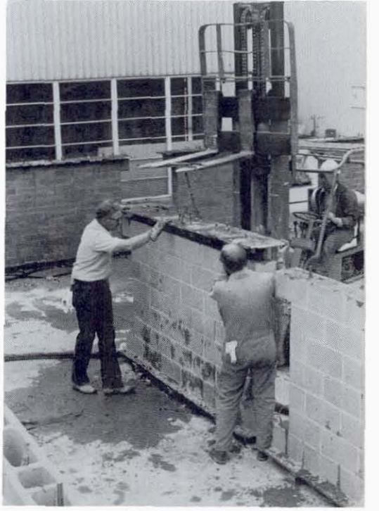
FIG. 2.2 CONSTRUCTION OF TEST SPECIMENS
