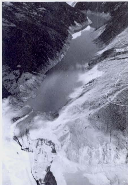
FIGURE 17. Air photo taken July 7, 1974 looking upstream from the debris dam showing the debris fall back zone and some areas of mud splatter in the foreground.
