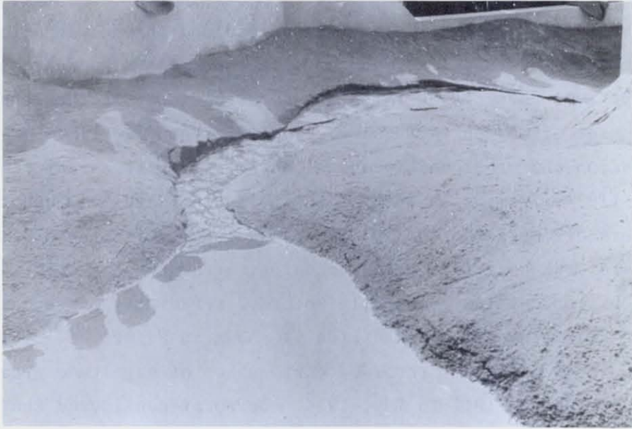
FIGURE 44. Hydraulic model looking downstream during peak flood.
