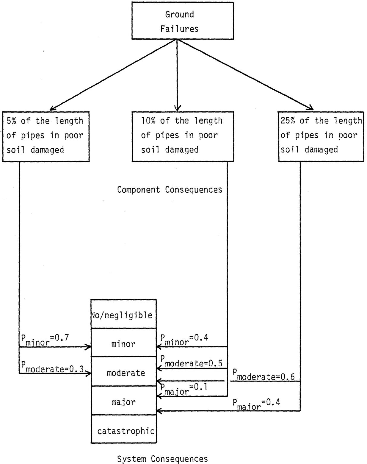
Figure 5.1 - Component and System Consequences for the MDC Water System
