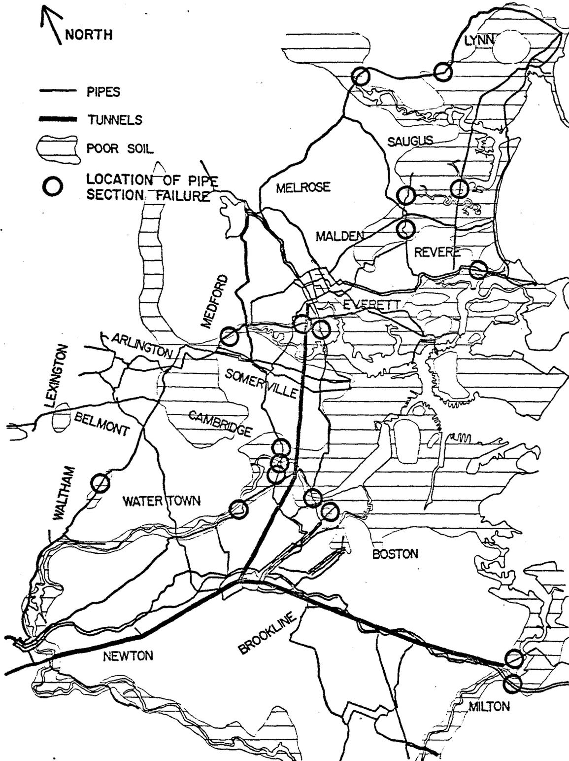
Figure A.1 - 25% Pipe Failure in Poor Soil: Simulation Case 1
