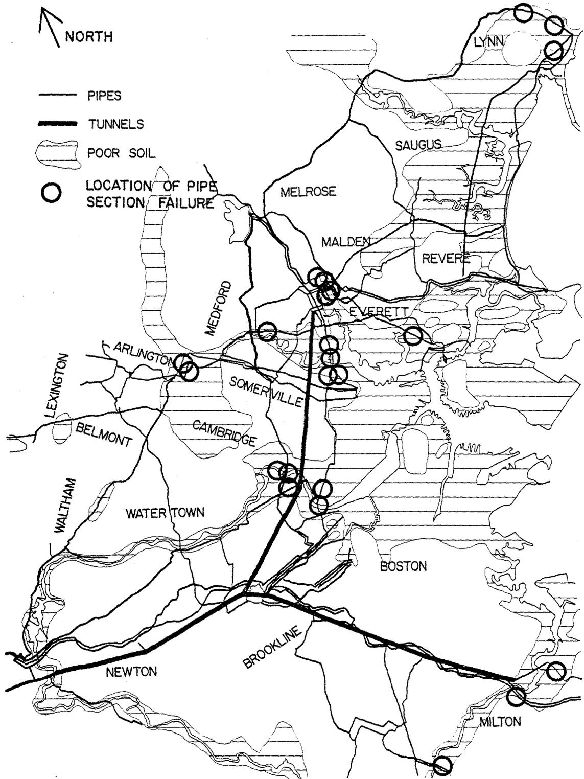
Figure A.2 - 25% Pipe Failure in Poor Soil: Simulation Case 2
