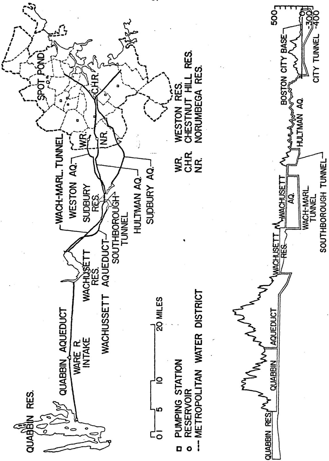
Figure 4.1 - General Plan of the M.D.C. Water System (MDC - Metropolitan Water System)
