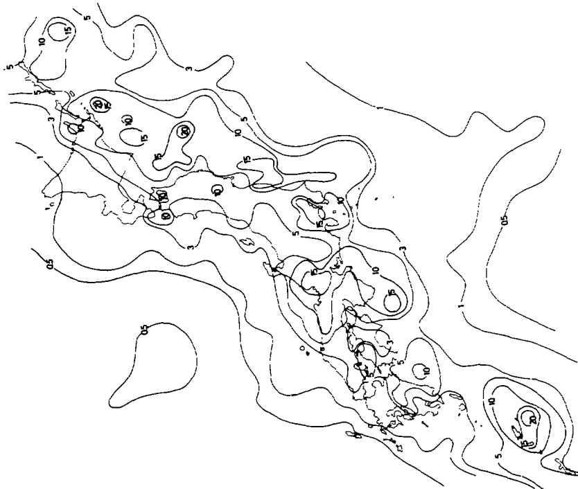
Fig. 2 An example of regional distribution of the maximum velocity amplitude (kine) expected at the base rock for return period 100 years.
