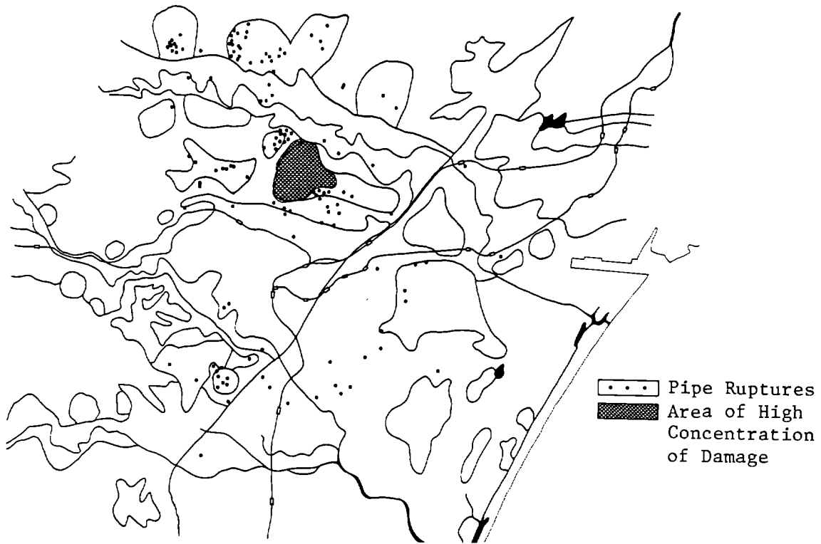
Fig.3.3. Location of Ruptures in Water Distribution Mains.
