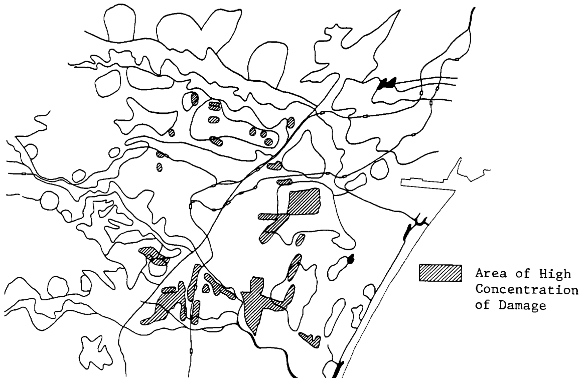
Fig.3.4. Location of Areas with Heavy Damage to Power Distribution Facilities.
