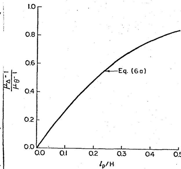
Fig. 3: Ductilities and plastic hinge length
