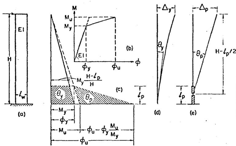
Fig. 1: Moments and deformations in a cantilever wall
