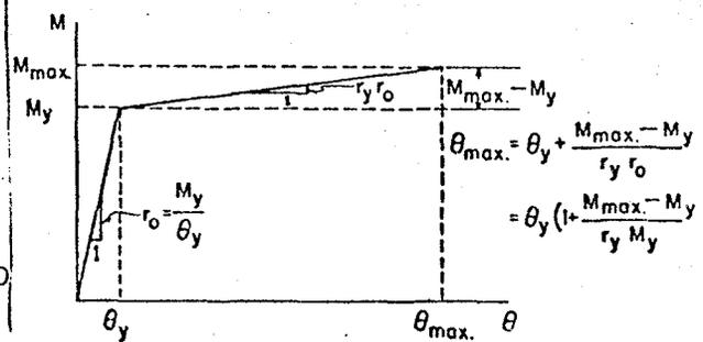
Fig. 4: Moment-rotation characteristics of plastic hinge
