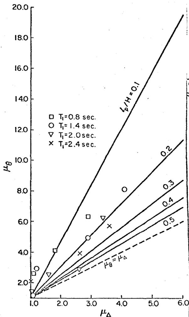
Fig. 2: Rotational ductility vs. displacement ductility
