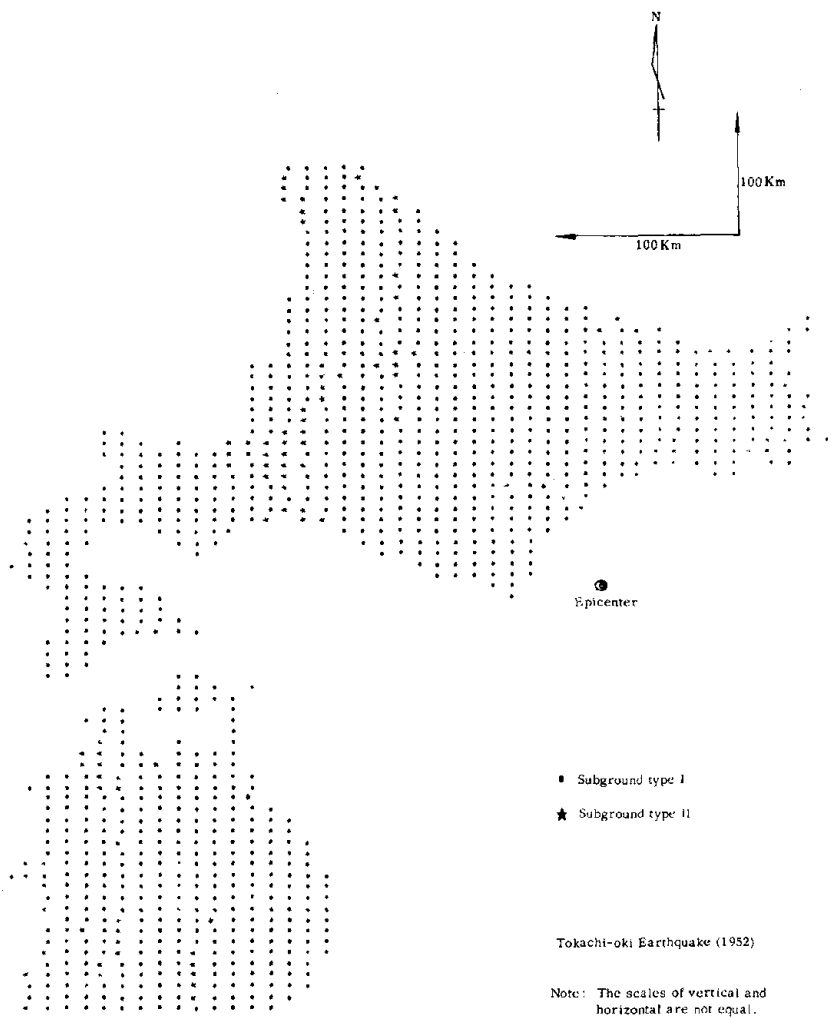
Fig. 3 An Example of Subground Types
