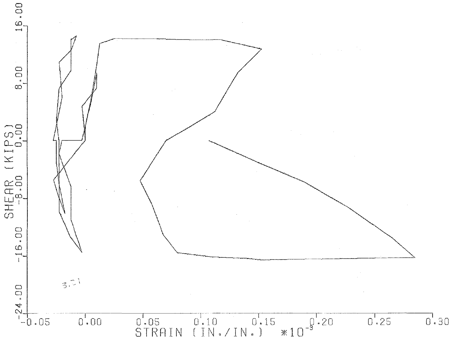
Figure 3.21 Specimen 2, strain on packaging band next to joint for deflection cycles 1, 4, and 7.
