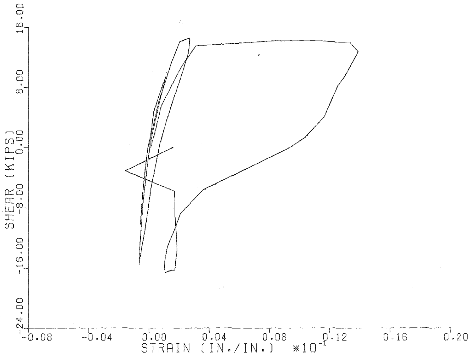
Figure 3.18 Specimen 2, average strain on bottom No. 7 bars, 1-in. from joint for deflection cycles 1, 4, and 7.
