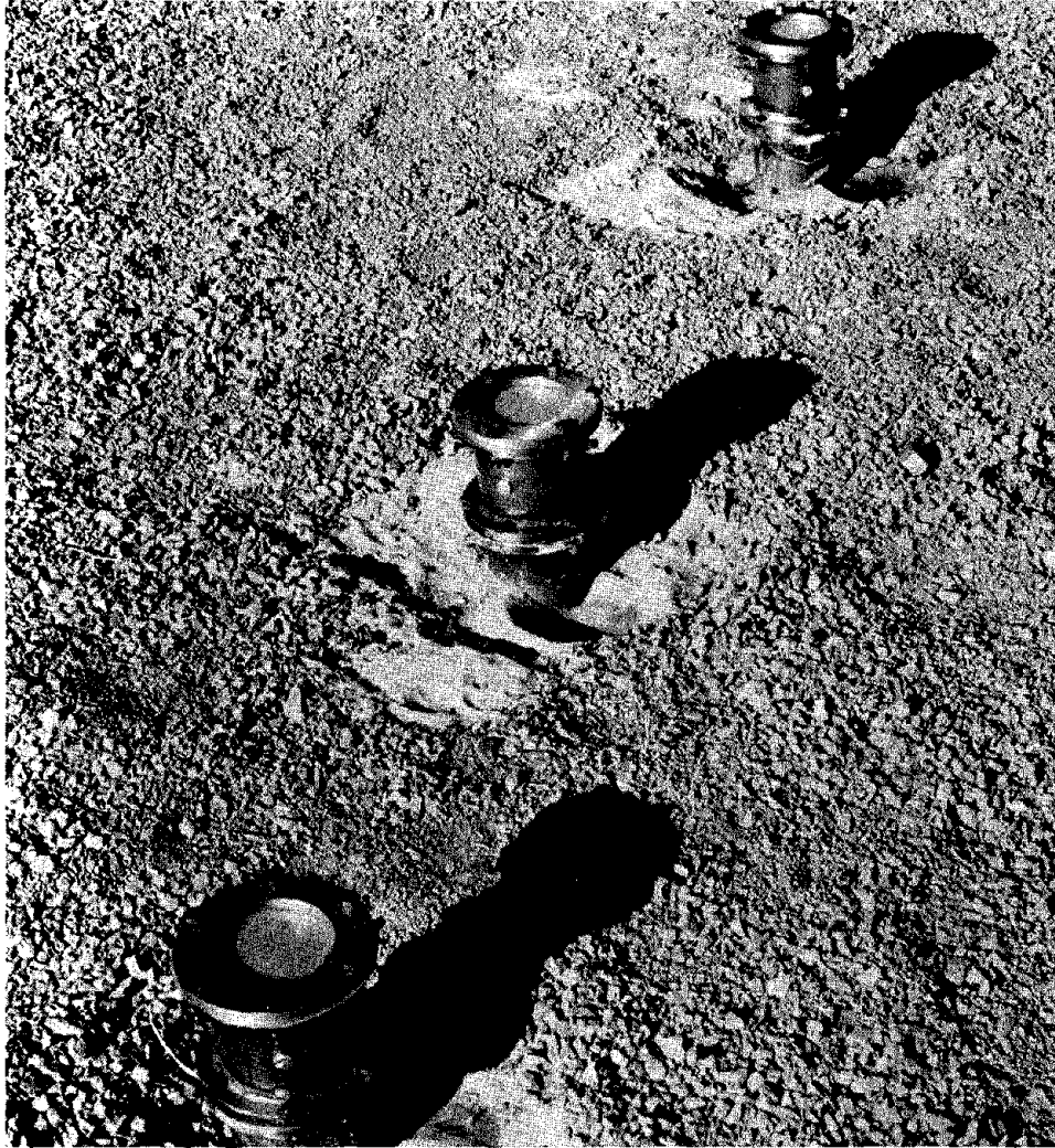
FIGURE 15 CLOSE-UP OF THREE SOURCES IN ARRAY (Before hook-up of detonation system)
