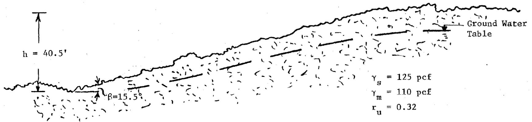
FIGURE 3. GEOMETRY OF THE SLOPE USED IN CASE STUDY
