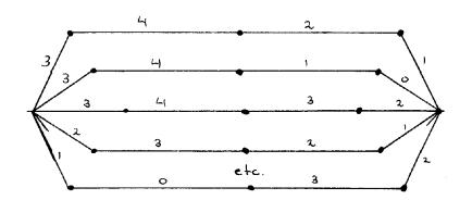
Using any one of the three schemes developed earlier in this report now becomes much easier due to the reduced complexity of the network, i.e., series systems in parallel.
