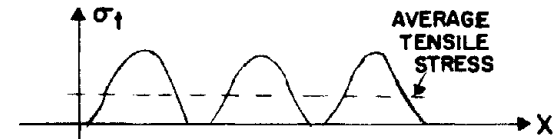
Fig. 6.7c Concrete stress distribution along AXIS 1-1
