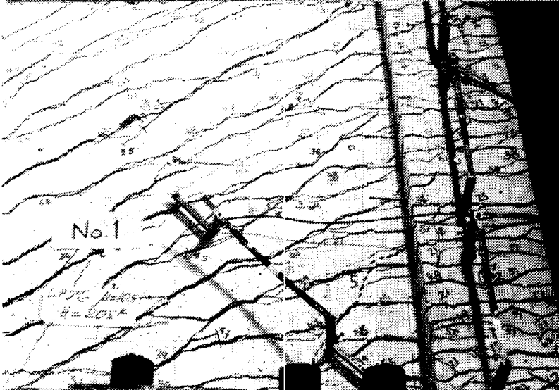
Fig. 4.8 Tension Cracks in South Panel and Column, Specimen 3
