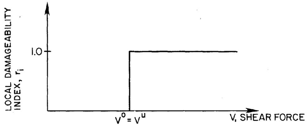
FIGURE 3.5 PARAMETER FOR ASSESSMENT OF DAMAGE DUE TO SHEARING FORCE IN A COLUMN
