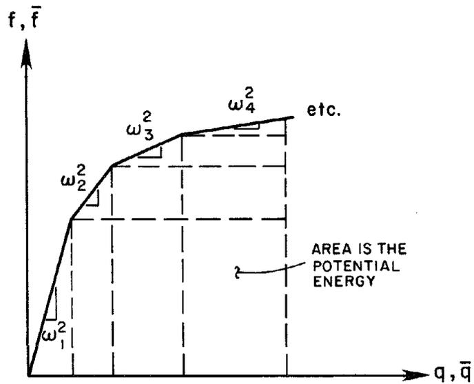
FIGURE 6.4 FORCE-DISPLACEMENT RELATIONSHIP FOR NONLINEAR INCREMENTS WITH A FORCE DISTRIBUTION OF CONSTANT SHAPE
