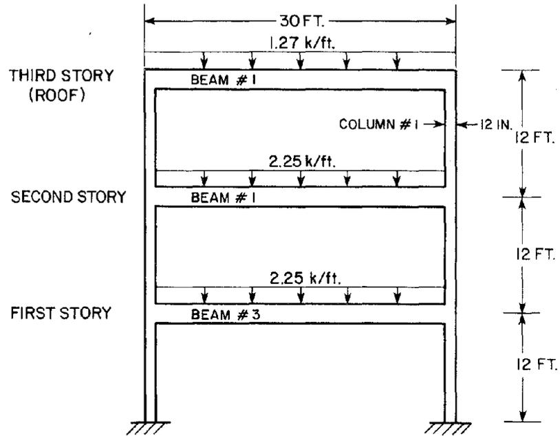
FIGURE 7.5 EXTERIOR XX FRAME OF MODEL STRUCTURE, SECTION II-II
