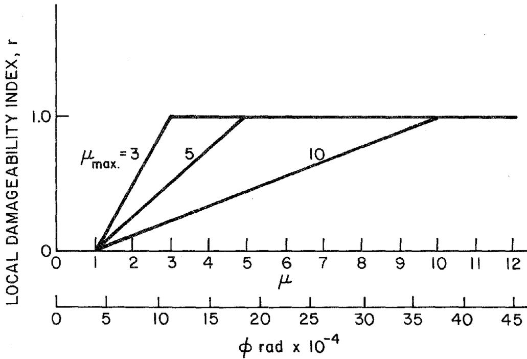
FIGURE 7.15 DAMAGEABILITY INDEX FOR THE FIRST STORY, CENTER COLUMN
