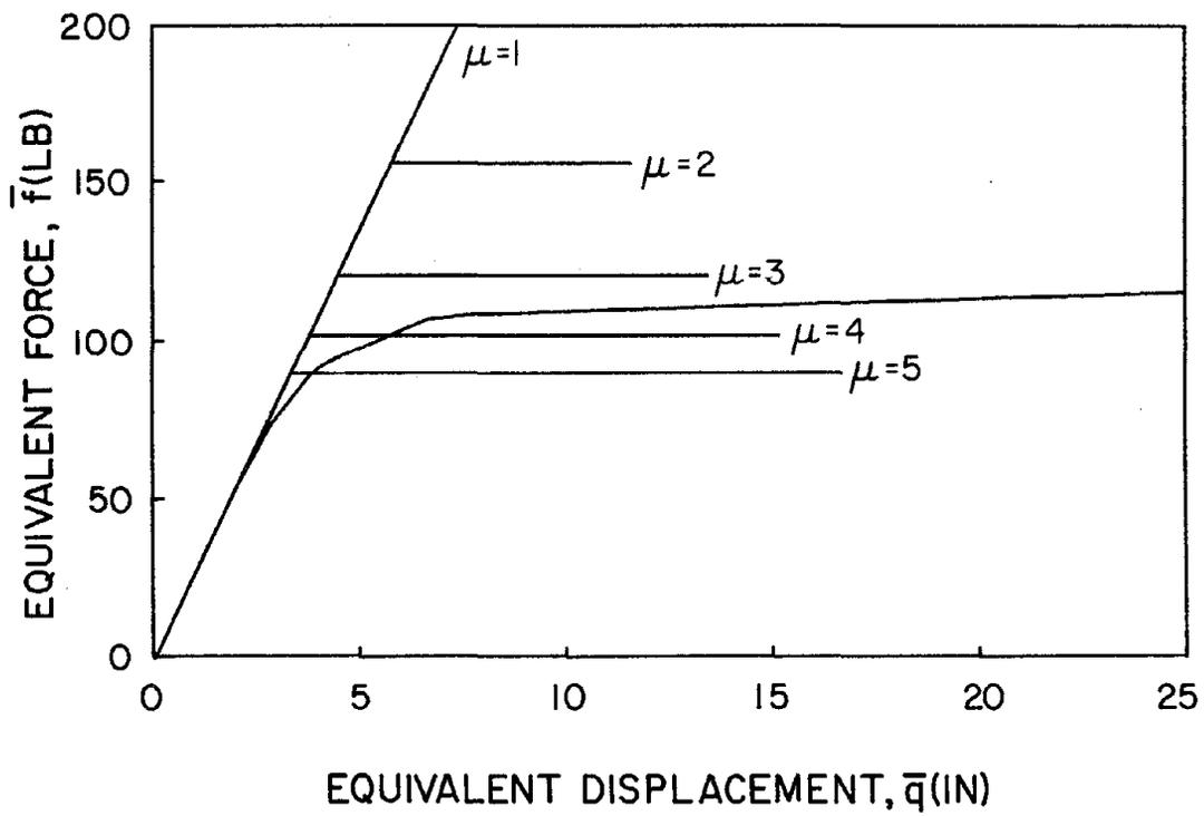
FIGURE 7.19 COMPARISON OF FORCE-DISPLACEMENT RELATIONSHIP FOR SPECTRA 1
