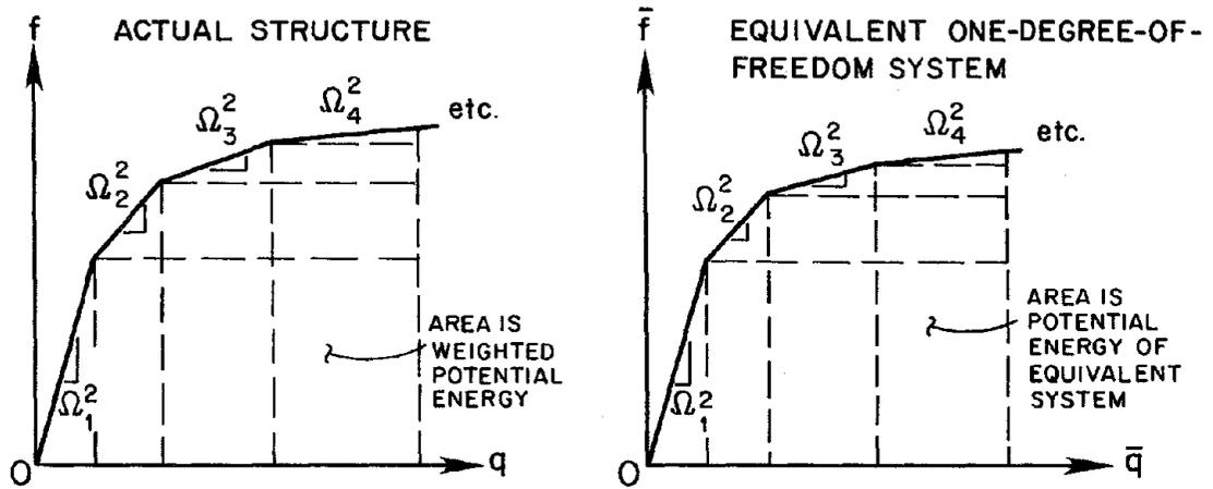
FIGURE 6.6 FORCE-DISPLACEMENT RELATIONSHIPS FOR NONLINEAR INCREMENTS WITH MODIFIED FORCE DISTRIBUTIONS
