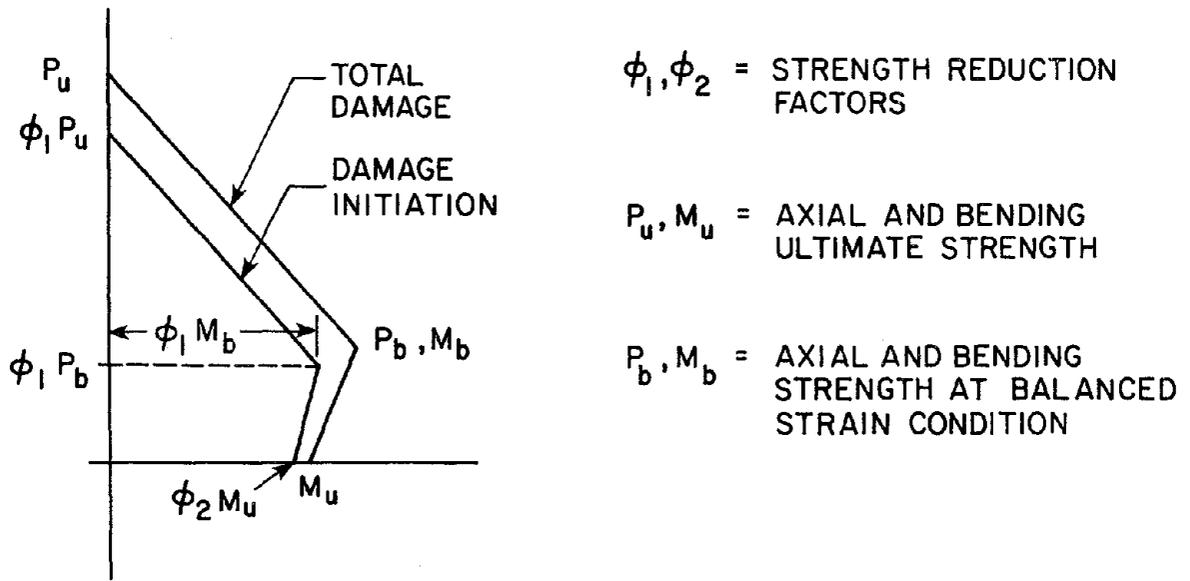
FIGURE 3.3 STRENGTH PARAMETERS FOR DAMAGE EVALUATION OF A COLUMN
