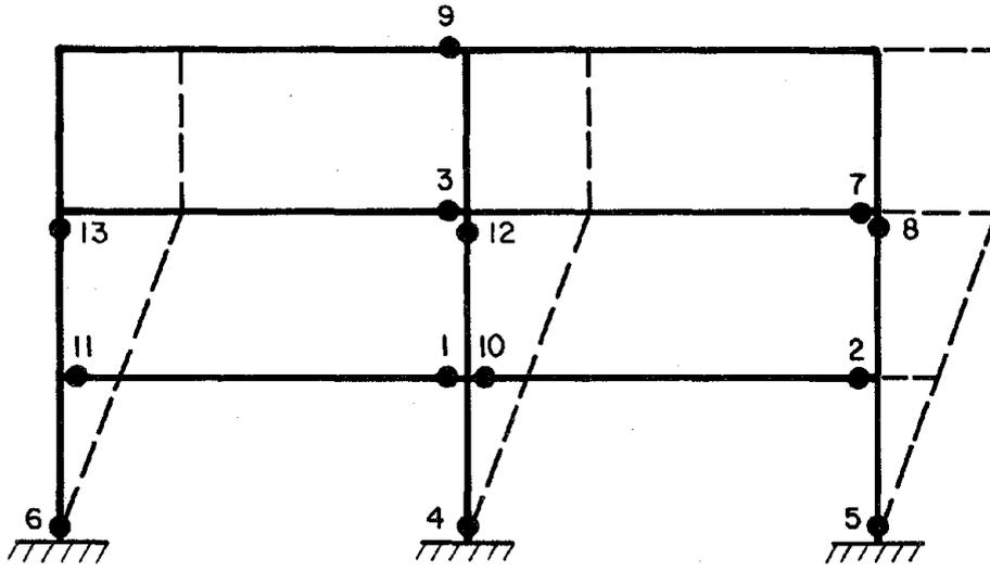
FIGURE 7.12 ORDER OF HINGES AND COLLAPSE MECHANISM
