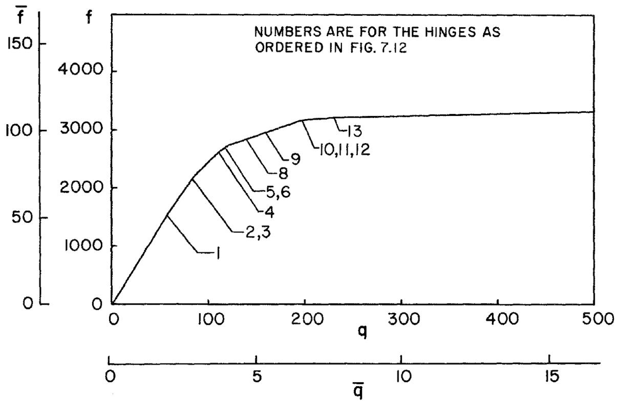
FIGURE 7.13 FORCE-DISPLACEMENT RELATIONSHIP
