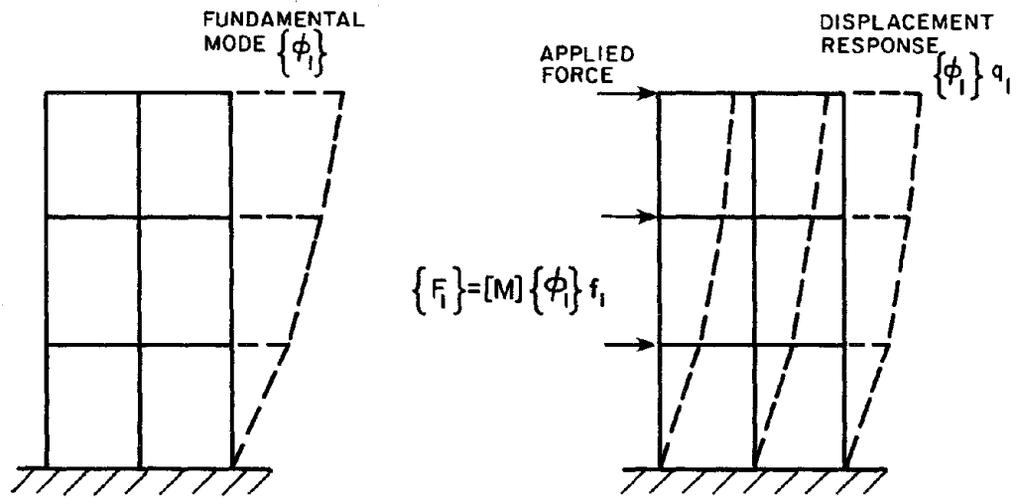
FIGURE 6.1 LINEAR ELASTIC QUASI-STATIC RESPONSE
