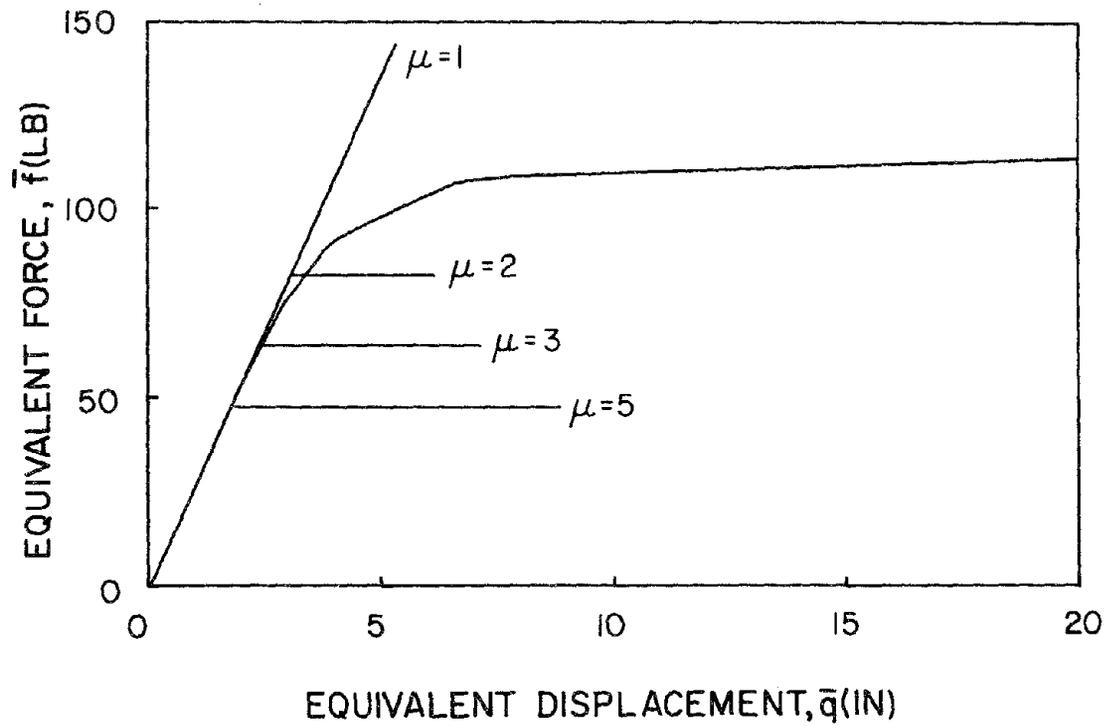
FIGURE 7.20 COMPARISON OF FORCE-DISPLACEMENT RELATIONSHIP FOR SPECTRA 2
