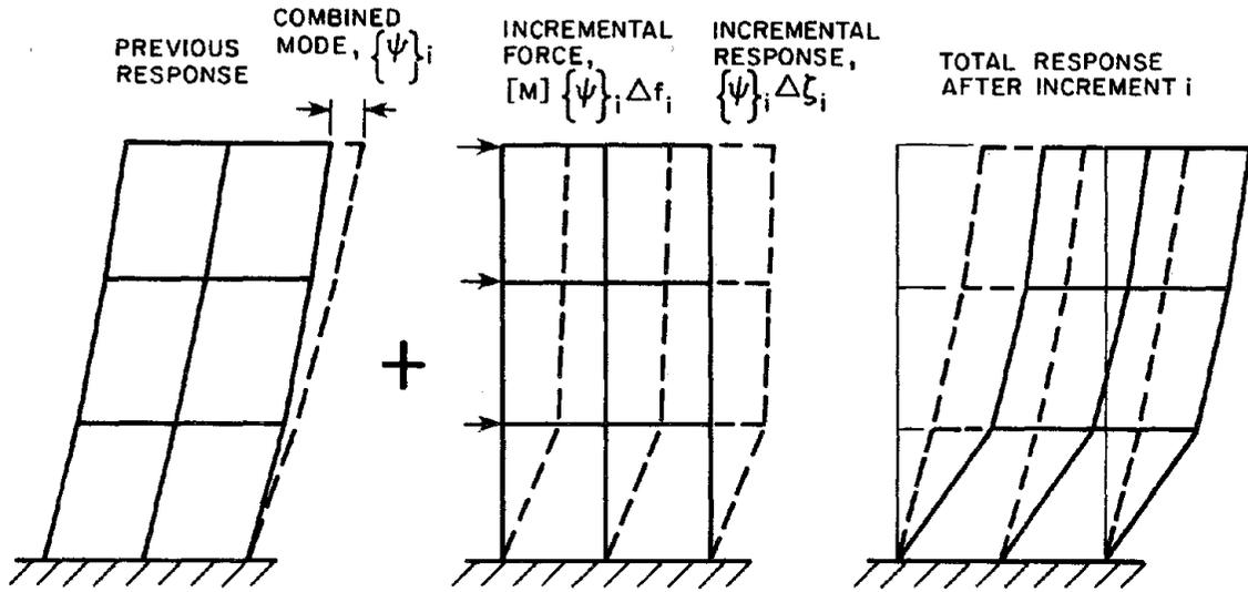
FIGURE 6.5 INCREMENT OF NONLINEAR RESPONSE WITH MODIFIED FORCE DISTRIBUTION
