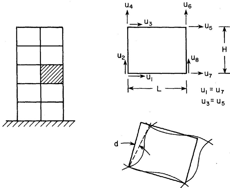
FIGURE 3.1 DEMAND PARAMETER FOR AN INFILLED WALL
