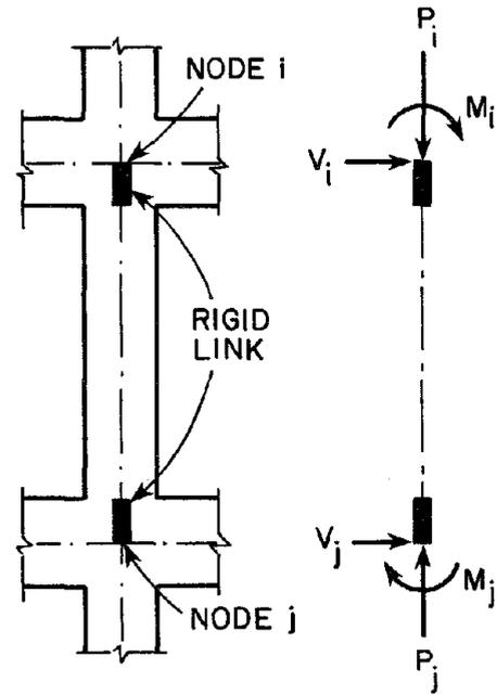
FIGURE 4.4 TYPICAL COLUMN MODEL
