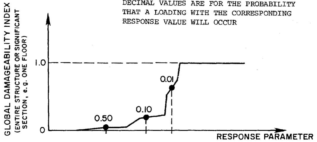
FIGURE 2.1 TYPICAL DAMAGEABILITY PROFILE FOR A CONTINUOUS QUASI-STATIC ANALYSIS
