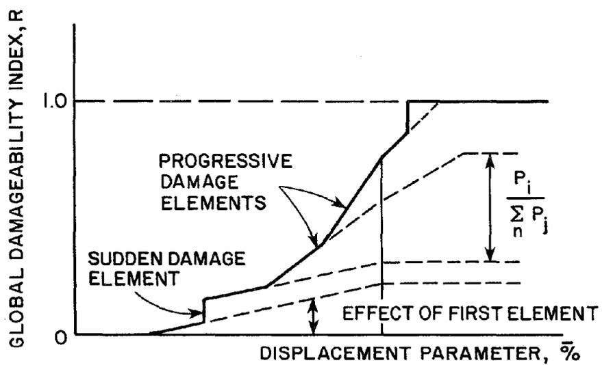
FIGURE 7.1 GLOBAL DAMAGEABILITY FOR A QUASI-STATIC RESPONSE ANALYSIS
