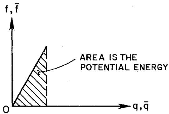
FIGURE 6.2 FORCE-DISPLACEMENT RELATIONSHIP FOR ELASTIC RESPONSE
