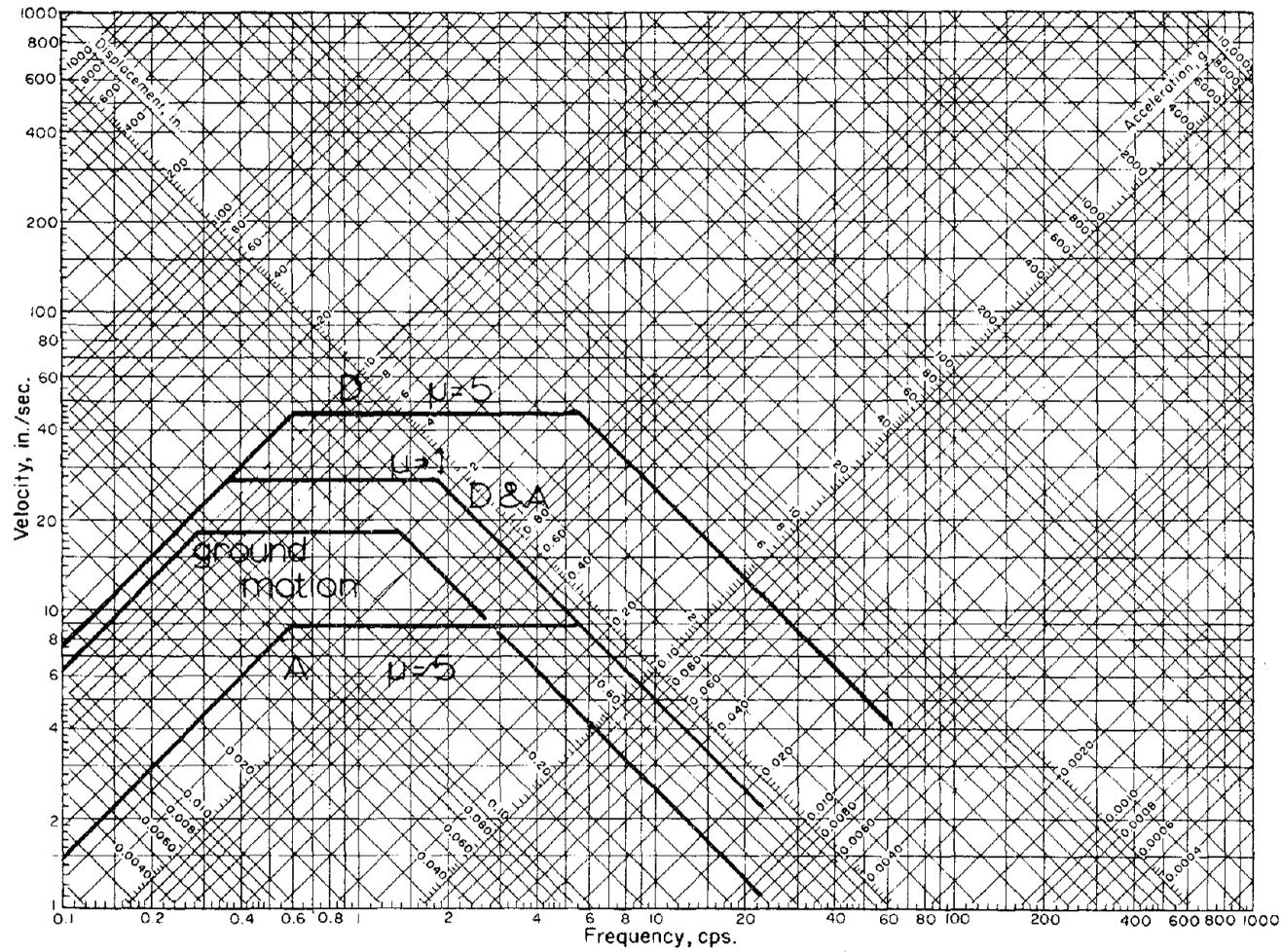
FIGURE 7.18 ELASTO-PLASTIC RESPONSE SPECTRA [15]
