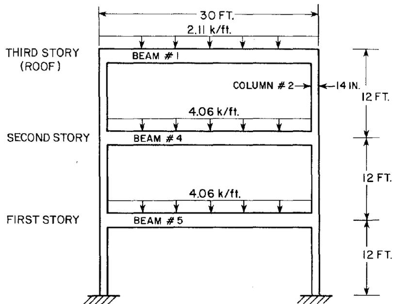
FIGURE 7.6 INTERIOR XX FRAME OF MODEL STRUCTURE, SECTION III-III
