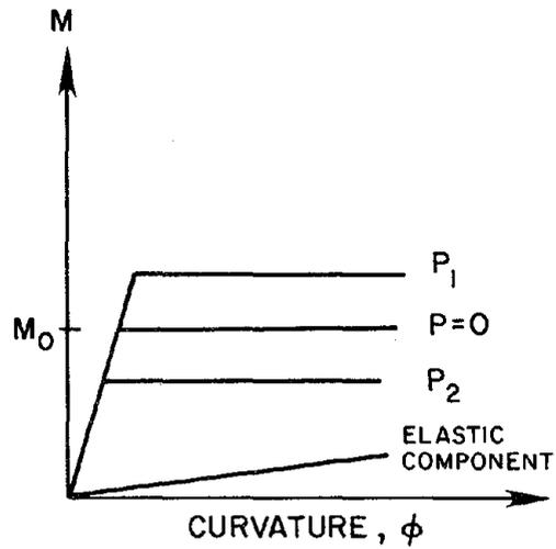
FIGURE 4.5 YIELD CRITERIA FOR A COLUMN ELEMENT
