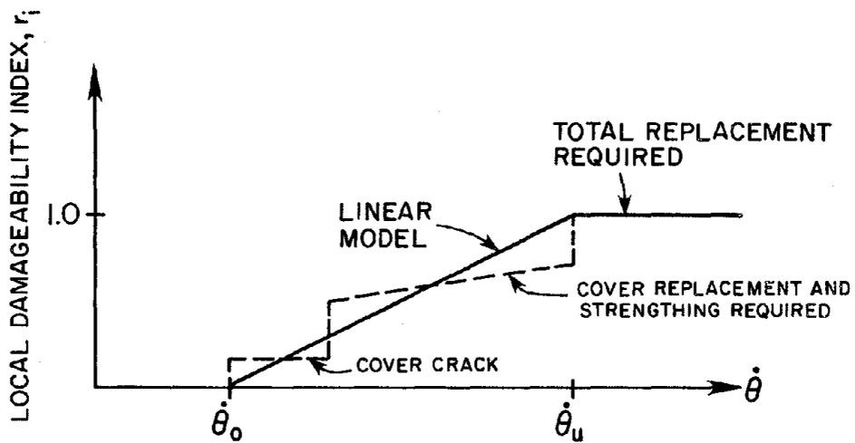
FIGURE 3.4 PARAMETER FOR DEGREE OF DAMAGE OF A COLUMN
