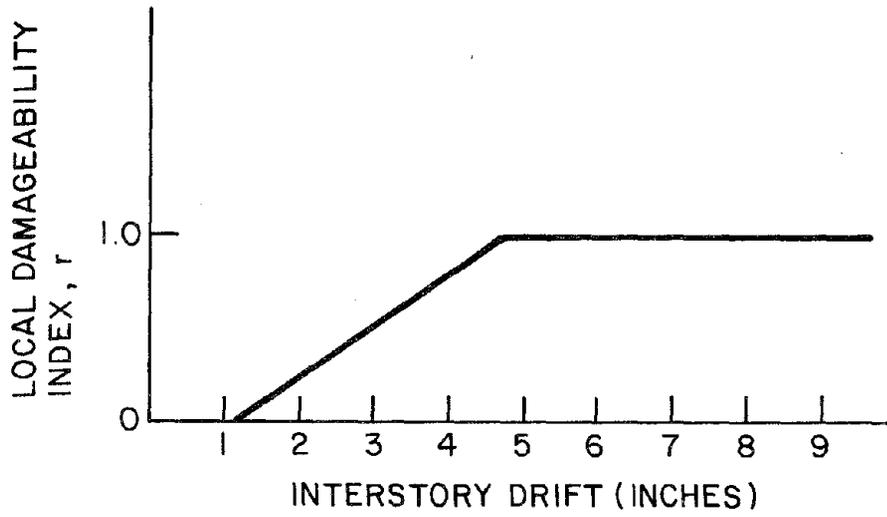
FIGURE 7.14 DAMAGEABILITY INDEX FOR PARTITIONS
