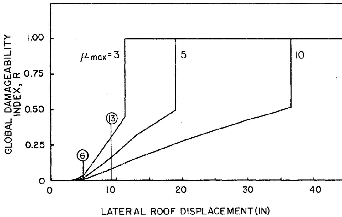
FIGURE 7.17 GLOBAL DAMAGEABILITY INDEX AND LATERAL ROOF DISPLACEMENT
