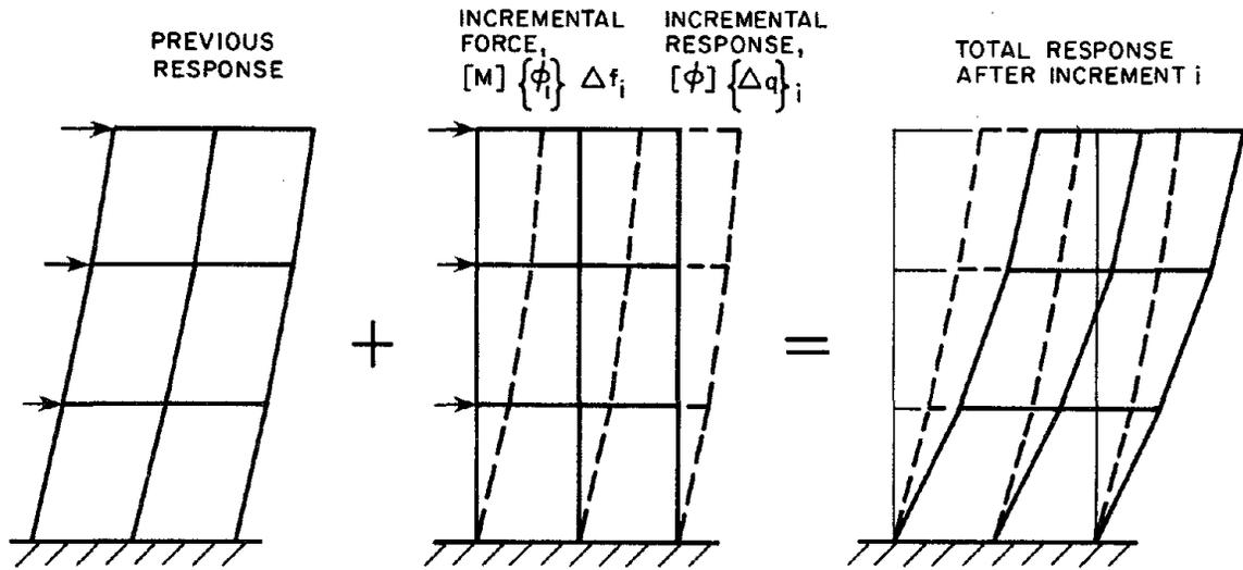
FIGURE 6.3 INCREMENT OF NONLINEAR RESPONSE WITH FORCE DISTRIBUTION OF CONSTANT SHAPE
