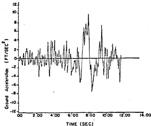
Figure 1. Example of a Subcritical Excitation with El Centro Intensity
