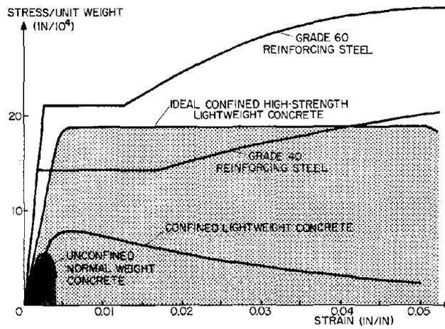
FIG. 2 STRESS PER UNIT WEIGHT - STRAIN DIAGRAMS FOR DIFFERENT CONCRETES AND REINFORCING STEELS
