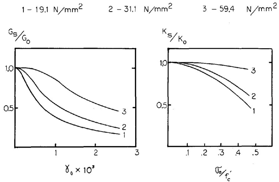
Figure 21: Secant Shear and Bulk Moduli for Three Concretes (7)
