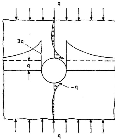
Fig. 2: Stress distribution around a circular hole in an infinite plate under unidirectional compressive load.
