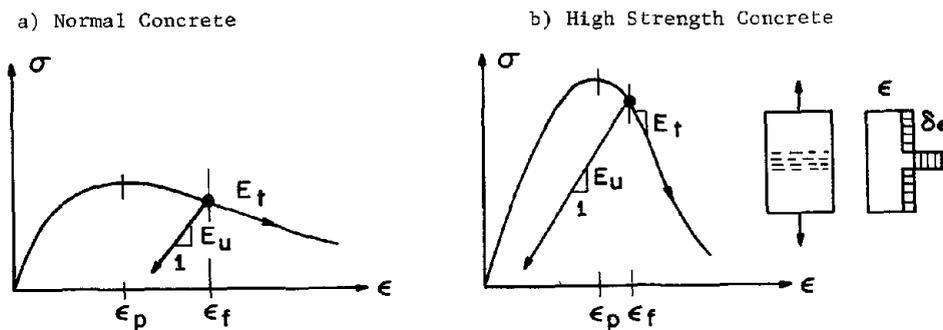
Fig. 2 Failure Strain  $\epsilon_f$  in Relation to Peak Strain  $\epsilon_p$ , and Bifurcation Giving Rise to Unstable Strain Localizations
