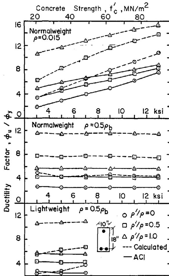
Fig. 7 Ductility ratios versus  $f'_c$  for reinforced concrete beams (Ref. 8)
