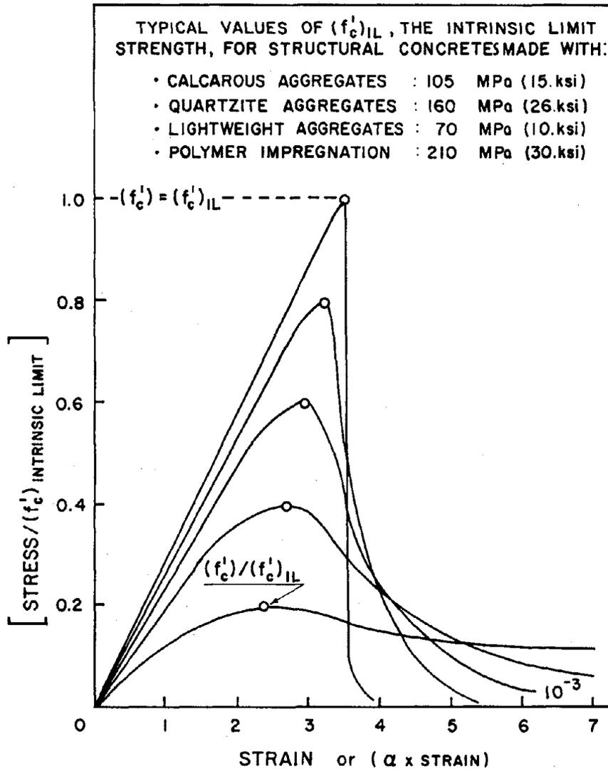
Fig. 2 Conceptual representation of the stress-strain curve of concretes in function of the intrinsic limit strength
