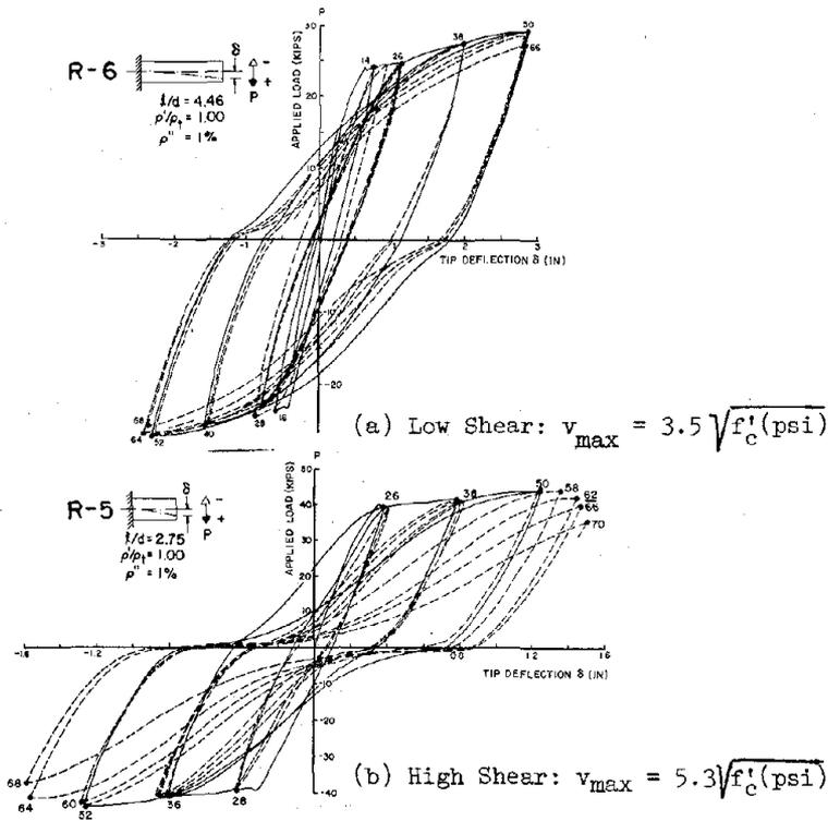
FIG. 20 COMPARISON OF HYSTERETIC BEHAVIOR OF REINFORCED CONCRETE AS AFFECTED BY DIFFERENT AMOUNTS OF SHEAR FORCE (48)
