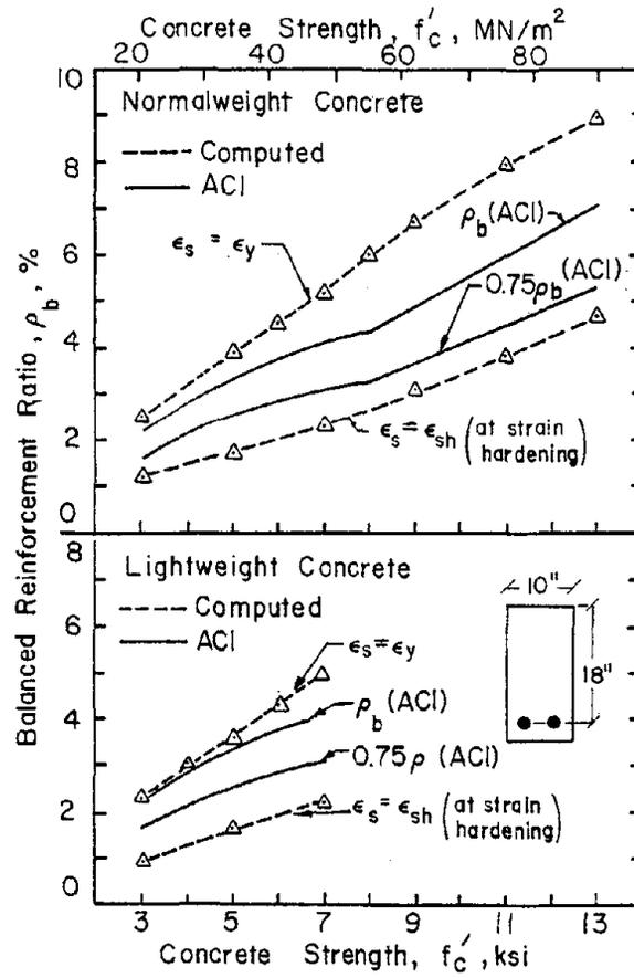
Fig. 9 Balanced reinforcement ratio versus  $f'_c$  (Ref. 8)
