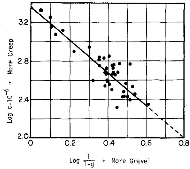
Figure 16: Effect of Aggregate Content on Creep (12)
