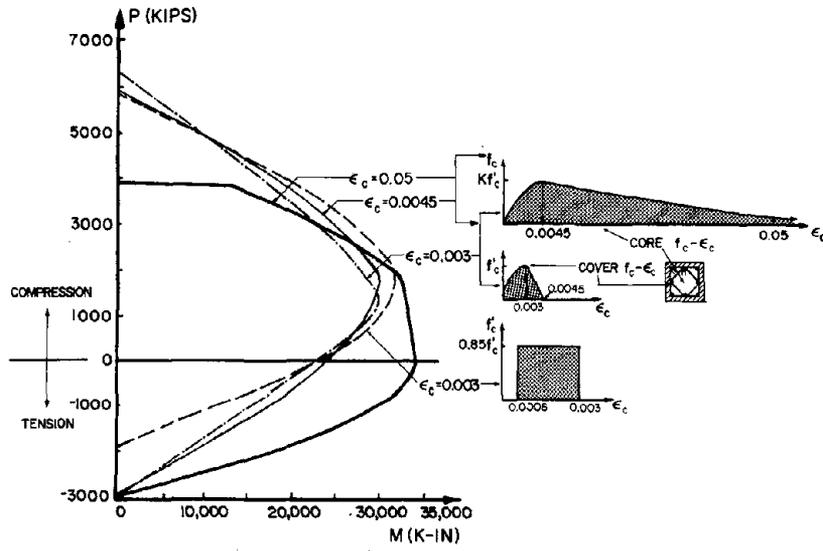
FIG. 11 COMPARISON OF P-M STRENGTH INTERACTION DIAGRAMS FOR THE SQUARE CROSS SECTION COLUMN OF FIG. 7 (31)
