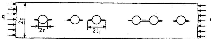
Fig. 4: Simplified simulation of a porous structure with randomly distributed pores.
