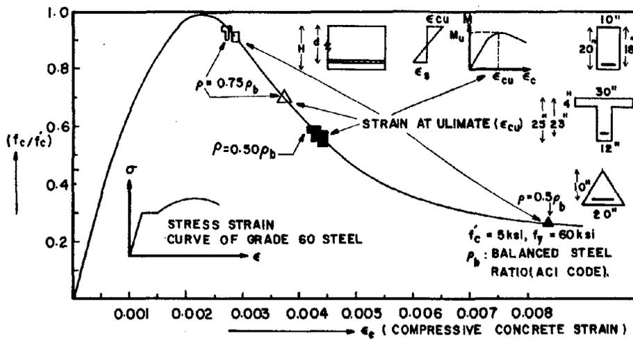
Fig. 4 Effect of cross sectional shape and reinforcement ratio on concrete strain  $\epsilon_{cu}$  at ultimate Ref. (3)
