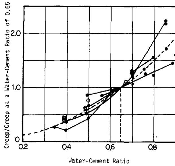
Figure 15: Effect of Water-Cement Ratio on Creep (12)
