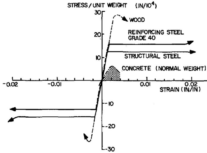
FIG. 1 STRESS PER UNIT WEIGHT - STRAIN DIAGRAMS FOR DIFFERENT STRUCTURAL MATERIALS
