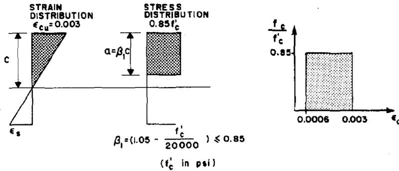
FIG. 10(a) EQUIVALENT STRESS BLOCK ASSUMPTIONS AND IMPLIED STRESS-STRAIN RELATIONSHIP FOR CONCRETE
