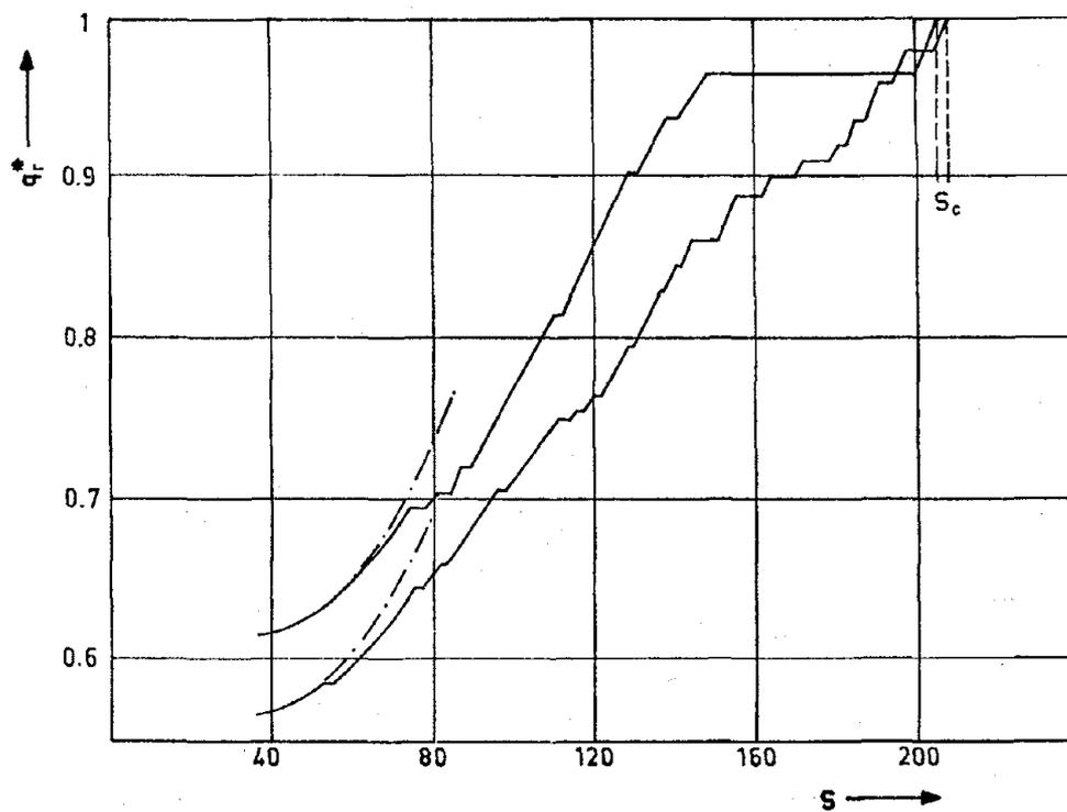
Fig. 5: Total crack length  $S$  (see equ. (6)) as function of load. Two runs of randomly distributed pores are shown. The means distance of the pores has been chosen to be four times the radius ( $r=1$ ) and a sample with 100 pores has been studied by this computer simulation.
