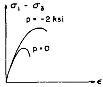
Fig. 4 Effect of Confining Hydrostatic Pressure
