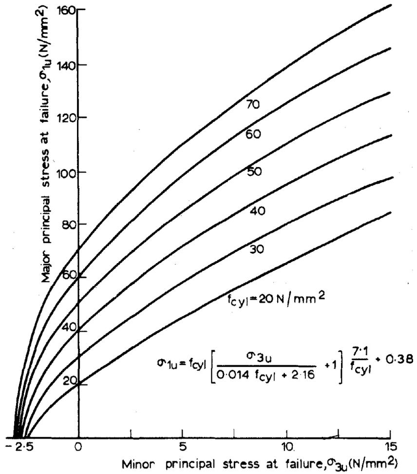
Figure 20: Failure stresses for various values of  $f_{cyl}$  (16)
