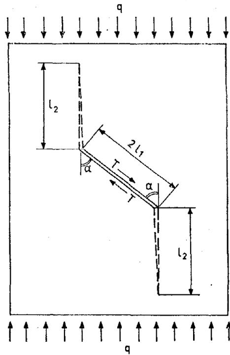
Fig. 6: Schematic representation of development of branching cracks and definitions of symbols used in corresponding equations.
