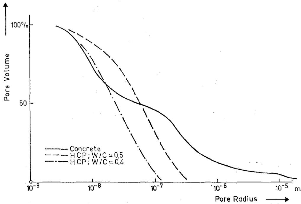
Fig. 1: Pores size distribution of concrete (solid line). For comparison corresponding distribution functions of hardened cement paste (HCP) with w/c-ratio 0,4 and 0,5 are shown by means of dashed lines.
