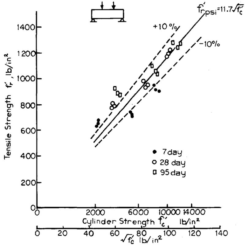
Figure 11: Tensile Strength based on Modulus of Rupture Test (4)
