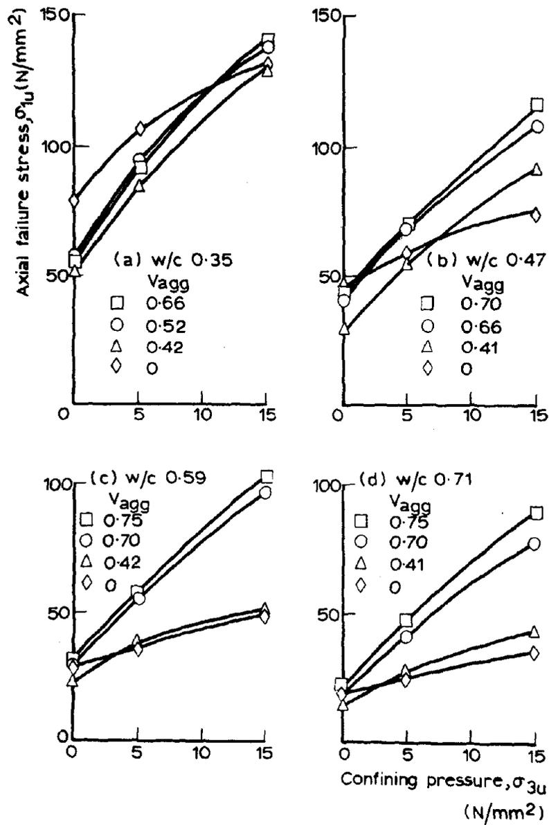
Figure 1: Influence of mix proportions on the strength of pastes and concretes in triaxial compression. ( 2 )
