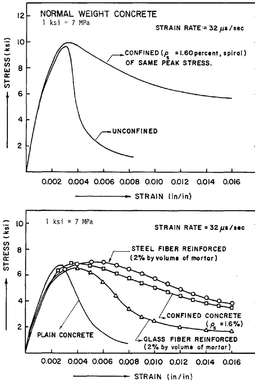
Fig. 8 Effect of confinement and fiber reinforcement on the ductility of concrete.
