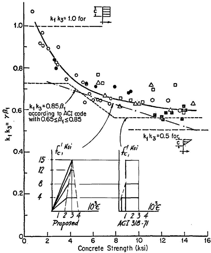
Figure 13:  $k_1 k_3$  versus concrete strength ( 4 )
