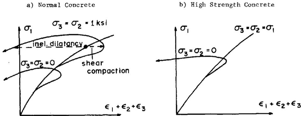
Fig. 3 Inelastic Dilatancy due to Shear and Shear Compaction
