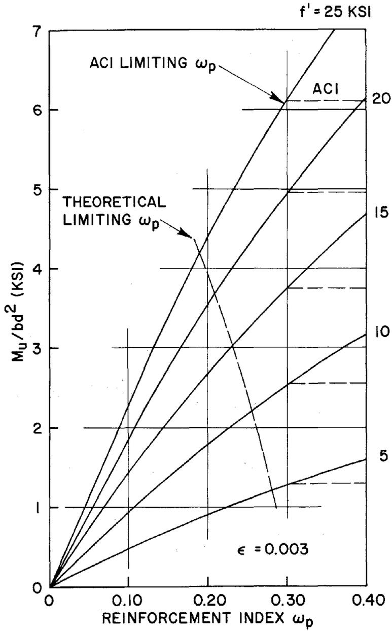
FIG. 4 MOMENT CAPACITY AS FUNCTION OF  $\omega_p$
