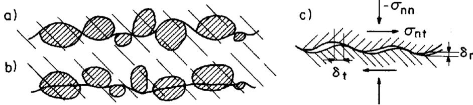
Fig. 7 Rough Crack in (a) Normal Concrete, (b) High Strength Concrete, and (c) Stress Transmission
