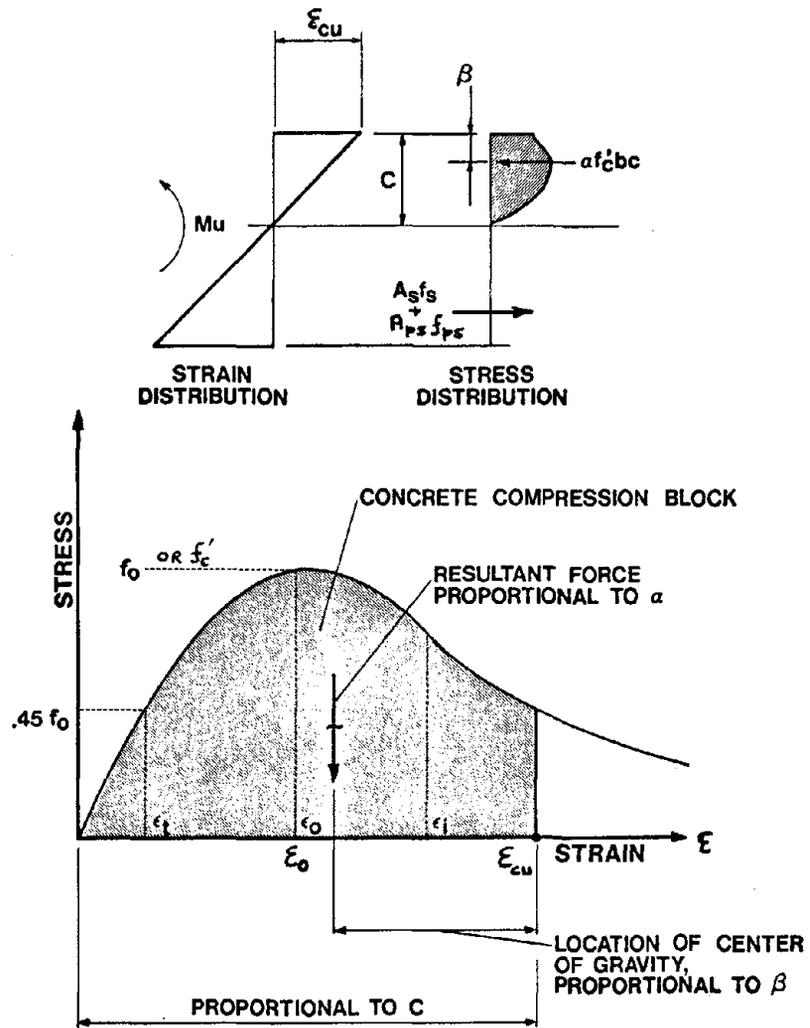
Fig. 5 Non identity of the peak strain of the concrete material  $\epsilon_0$  and the strain at ultimate capacity of the member  $\epsilon_{cu}$
