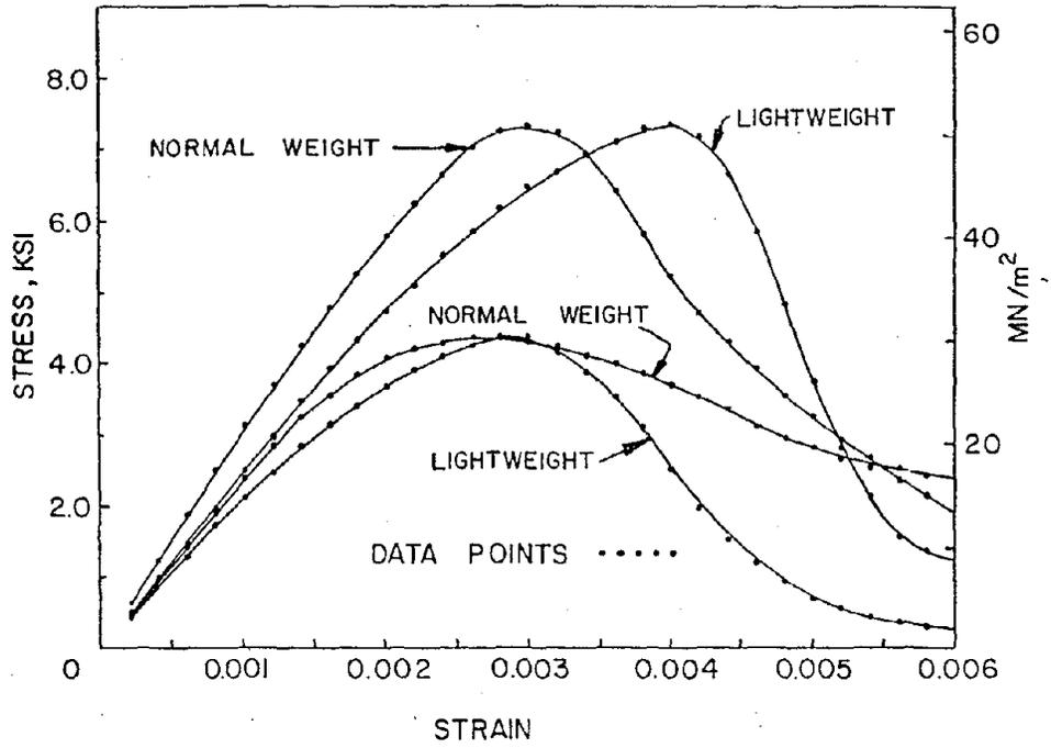
Fig. 1 Effect of Aggregates on the complete stress-strain curves of concrete (Ref. 5)
