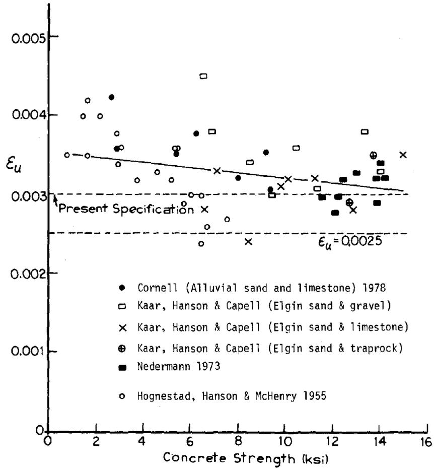
Figure 6: Ultimate Concrete Strain versus Concrete Strength (4)
