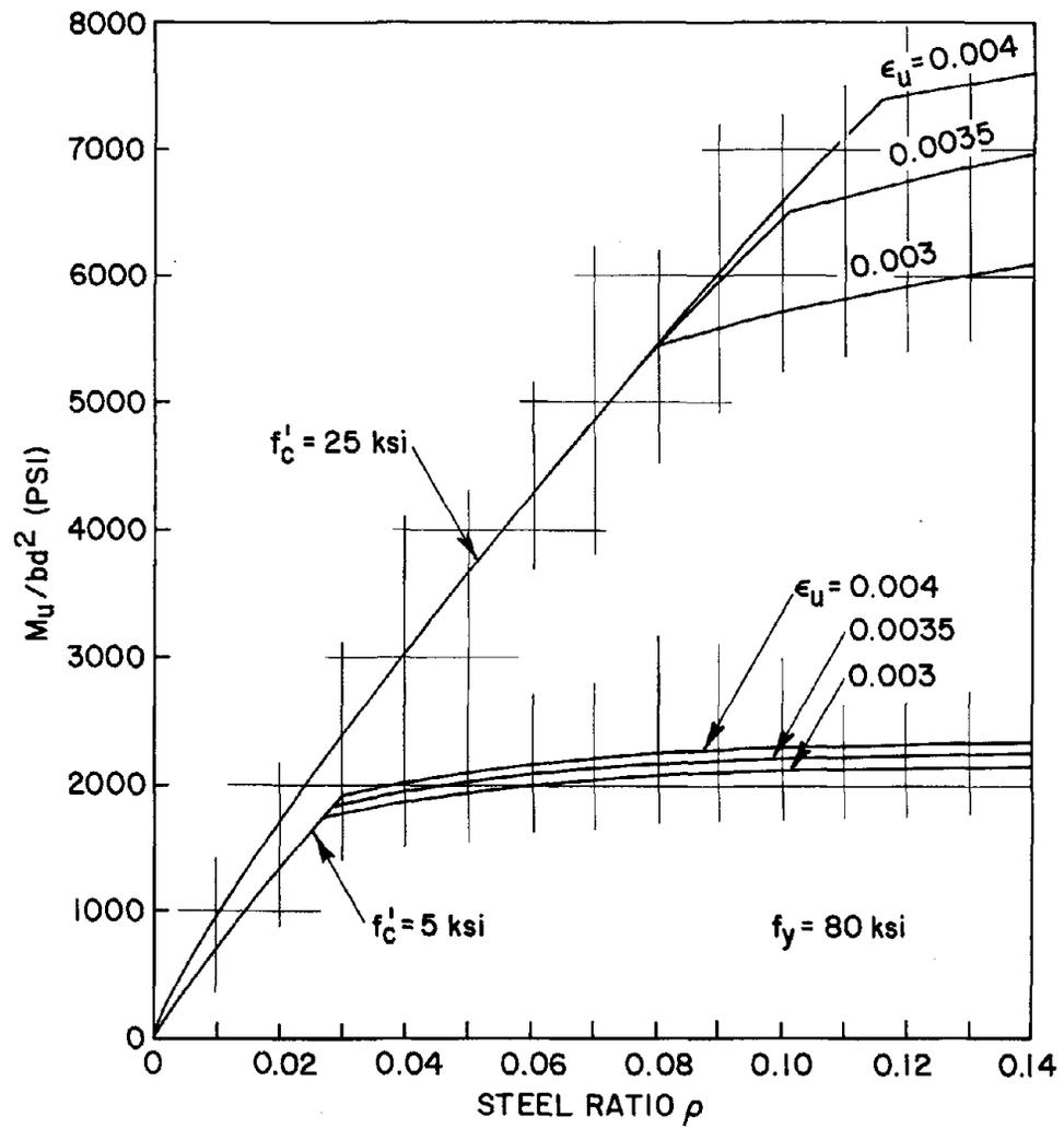
FIG. 3 EFFECT OF ULTIMATE CONCRETE STRAIN  $\epsilon_u$  ON
