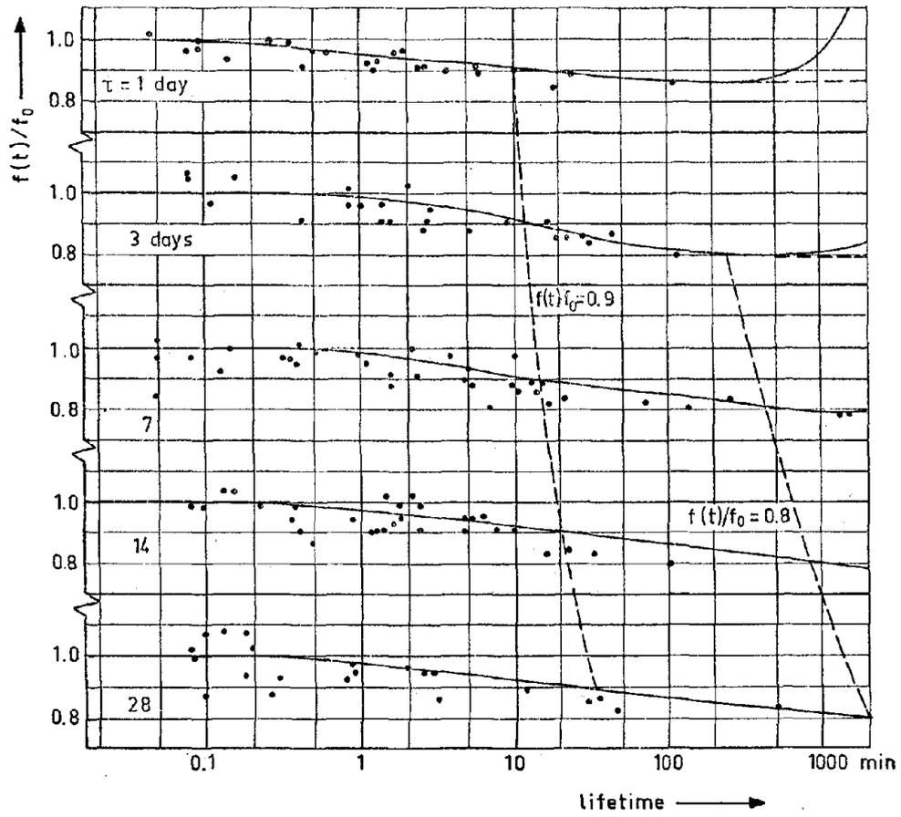
Fig. 12: Comparison of theoretical prediction of lifetime under high load with experimental results.
