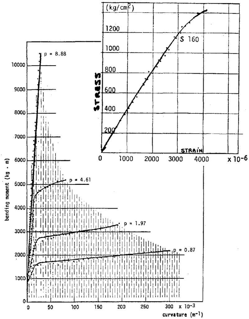
Fig. 6 Curvature versus bending moment for beams made with 160 MPa (23 ksi) concrete. (Ref. 7)
