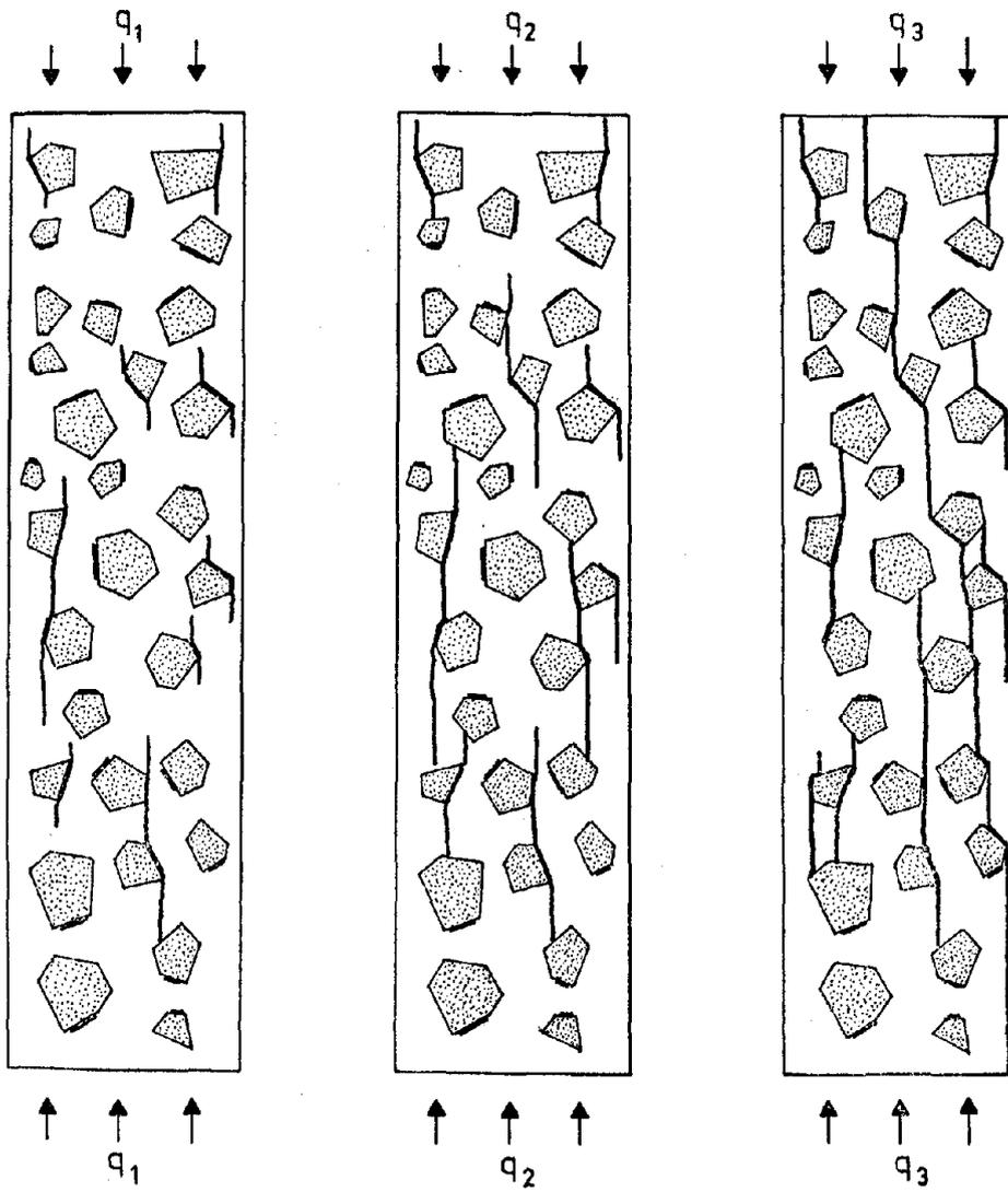
Fig. 10: Crack formation as calculated for normal concrete.
