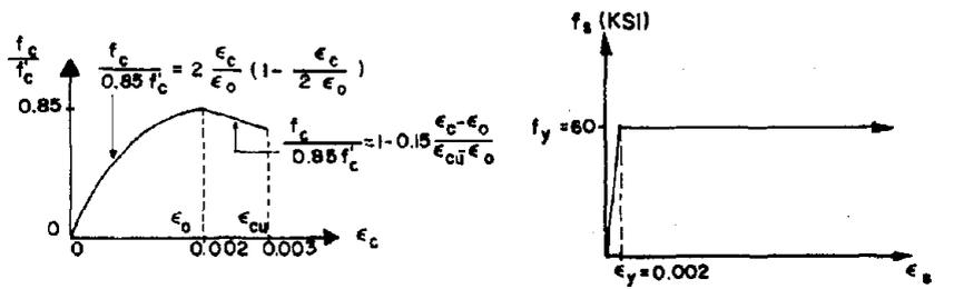
FIG. 10(b) HOGNESTAD STRESS-STRAIN RELATIONSHIP FOR CONCRETE
