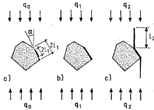
Fig. 7: Schematic representation of crack growth starting from an interface: (a-b) initial crack grows unstable along the interface: (b-c) stable branching cracks are developed.
