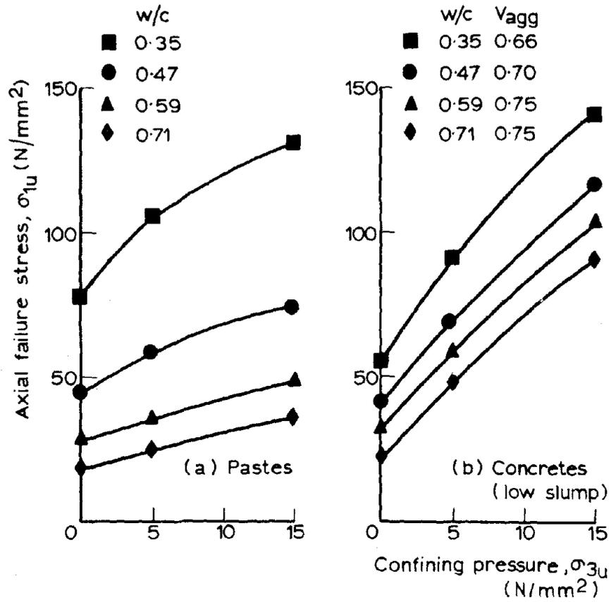
Figure 2: Influence of water/cement ratio on strength in triaxial compression. ( 2 )
