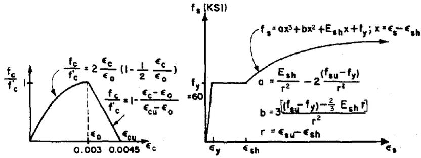
FIG. 9(a) STRESS-STRAIN RELATIONSHIP FOR CONCRETE COVER
