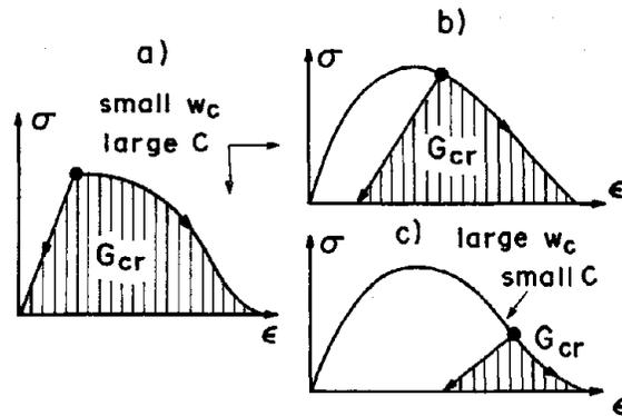
Fig. 6 Fracture Energy of Crack Band and Strain Localization
