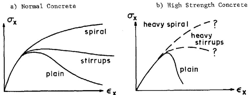
Fig. 1 Effect of Confining Reinforcement
