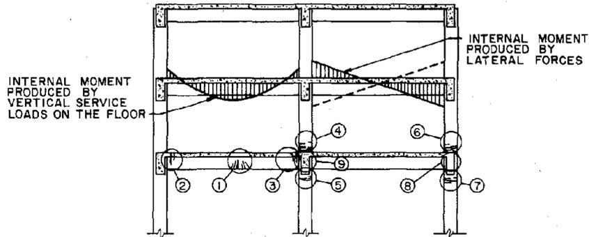
FIG. 16 TYPICAL CRITICAL REGIONS OF A REINFORCED CONCRETE MOMENT-RESISTING FRAME
