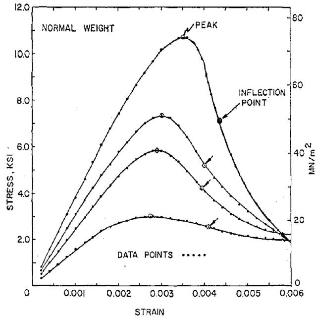
Fig. 3 Typical stress strain curves of same concrete tested at different ages (Ref. 5)
