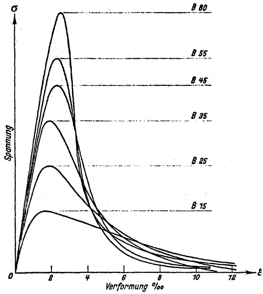
Figure 4: Complete Compressive Stress-Strain Curves ( 5 )
