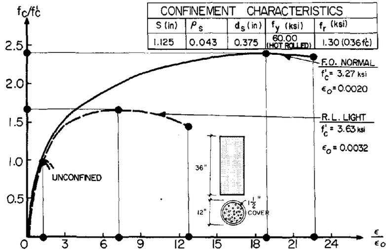
FIG. 14 NON-DIMENSIONAL STRESS-STRAIN RELATIONSHIPS FOR CONFINED, NORMAL, AND LIGHTWEIGHT CONCRETE (REF. 32)
