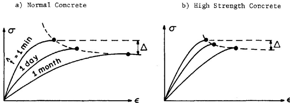
Fig. 8 Creep Isochrones and Long-Time Strength
