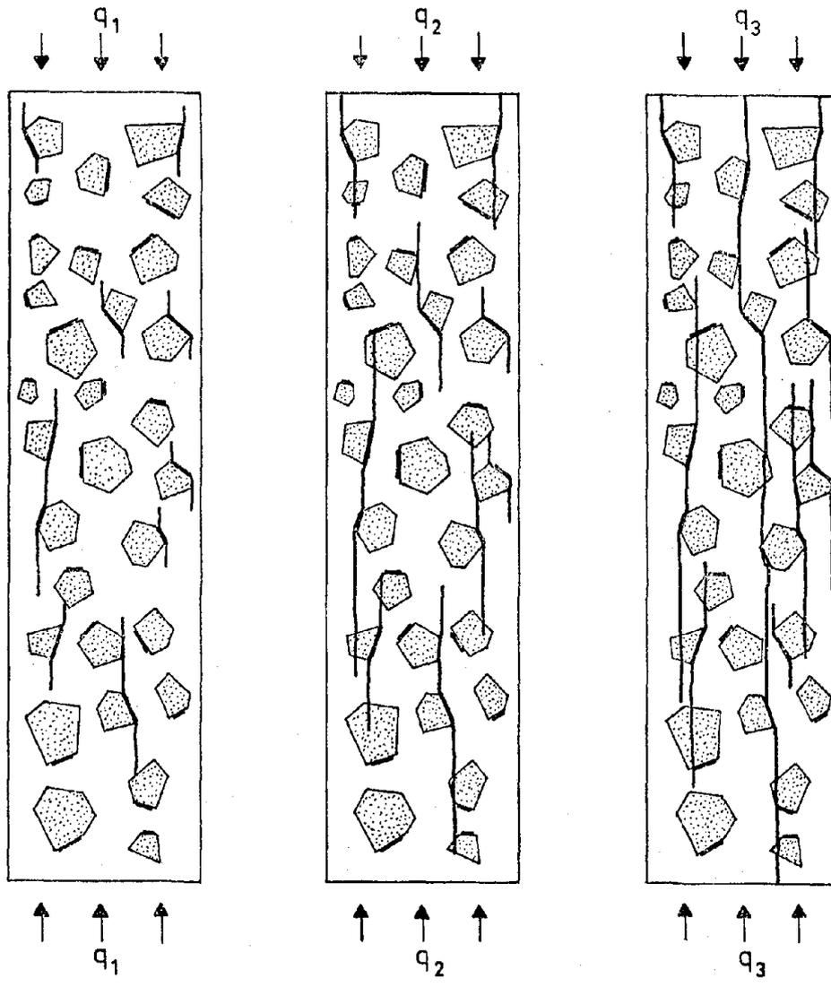
Fig. 11: Crack formation as calculated for high strength concrete.
