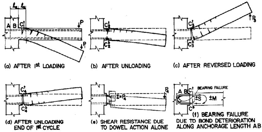
FIG. 19 EFFECT OF DEFORMATION REVERSAL ON REINFORCED CONCRETE FLEXURAL CRITICAL REGIONS (43)
