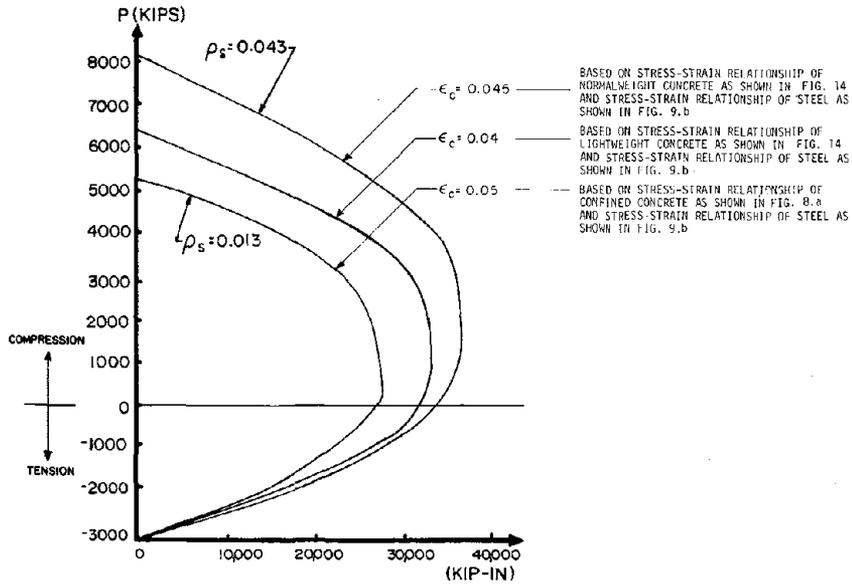
FIG. 13 EFFECT OF STRESS-STRAIN RELATIONSHIPS OF CONFINED CONCRETE (AS AFFECTED BY CONFINING PRESSURE AND AGGREGATE) ON THE P-M STRENGTH INTERACTION DIAGRAMS (31)
