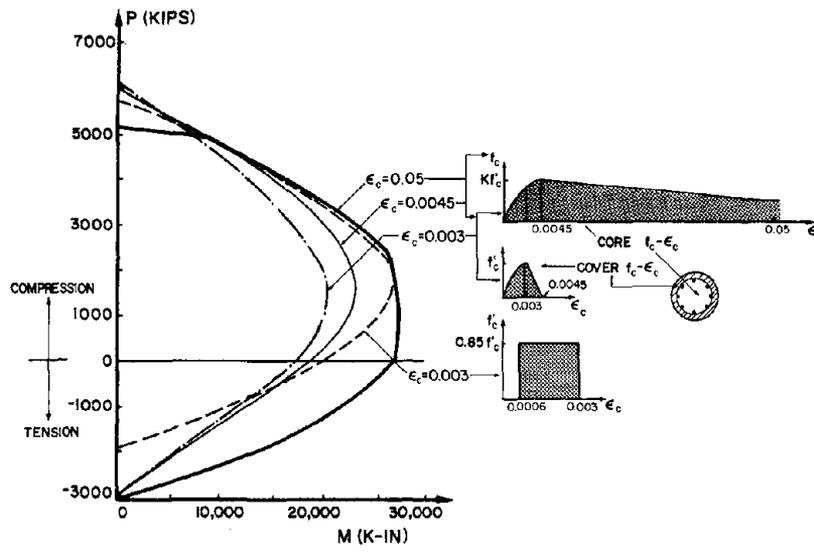
FIG. 12 COMPARISON OF P-M STRENGTH INTERACTION DIAGRAMS FOR THE CIRCULAR CROSS SECTION COLUMN OF FIG. 7 (31)
