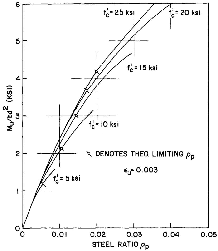
FIG. 5 MOMENT CAPACITY AS FUNCTION OF  $\rho_p$
