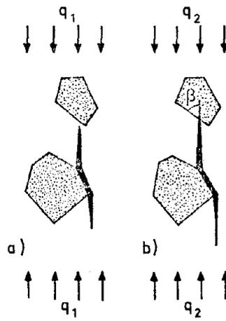
Fig. 8: A crack as created according to Fig. 7 meets a second inclusion.
