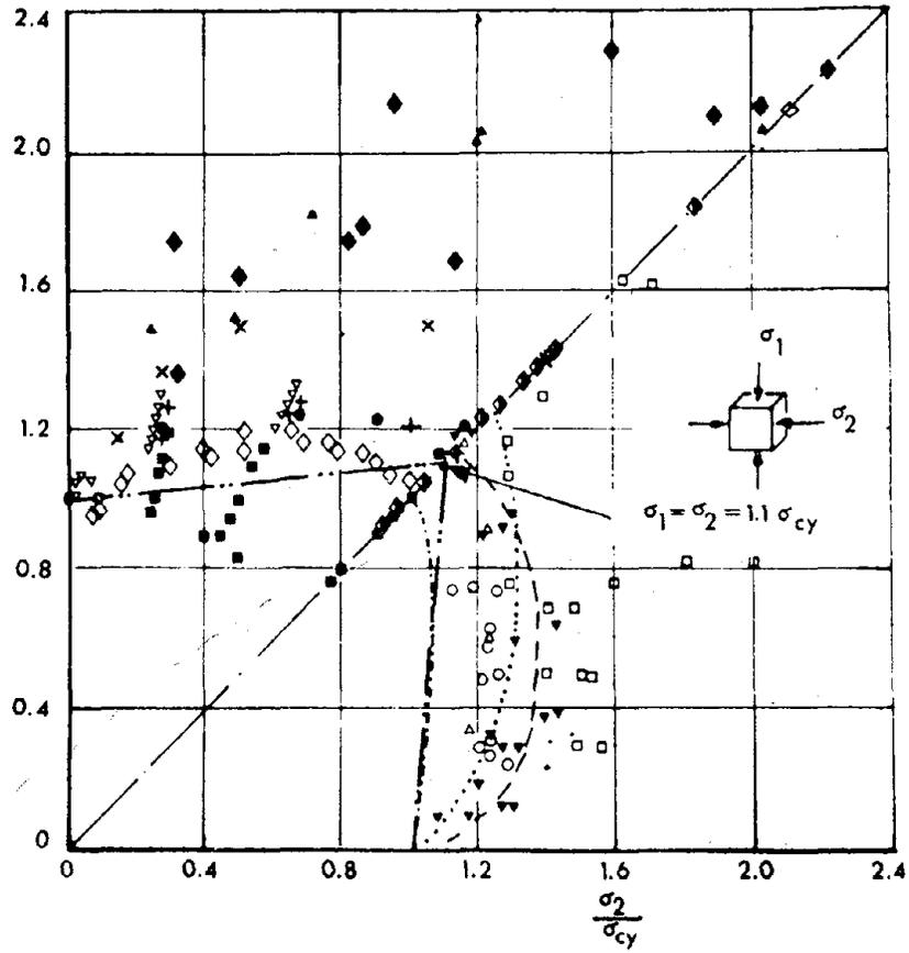
Figure 17: Failure under compression-compression-zero stress systems ( 15 )
