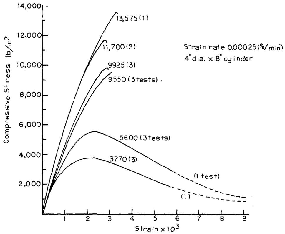
Figure 3: Compressive stress-strain curves (4)
