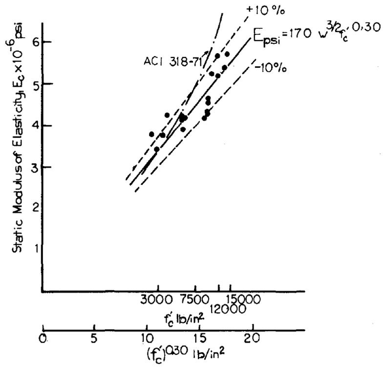
Figure 8: Static Modulus of Elasticity versus  $(f'_c)^{0.30}$  (4)
