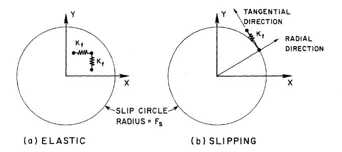
FIG. 5 STIFFNESS OF TANGENTIAL COMPONENT
