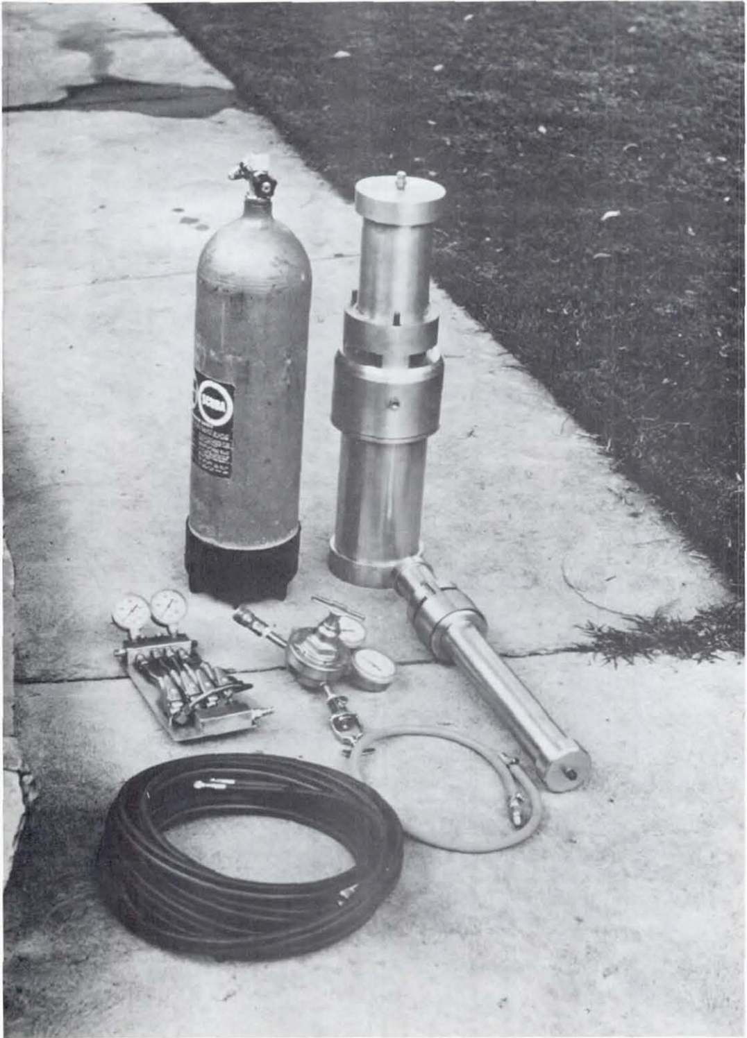
Fig. 11. Popper test instruments.
