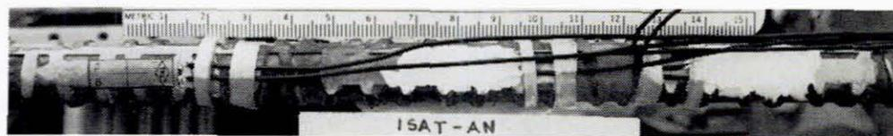
Figure 4.2 Strain gauges mounted on column reinforcing bar.
