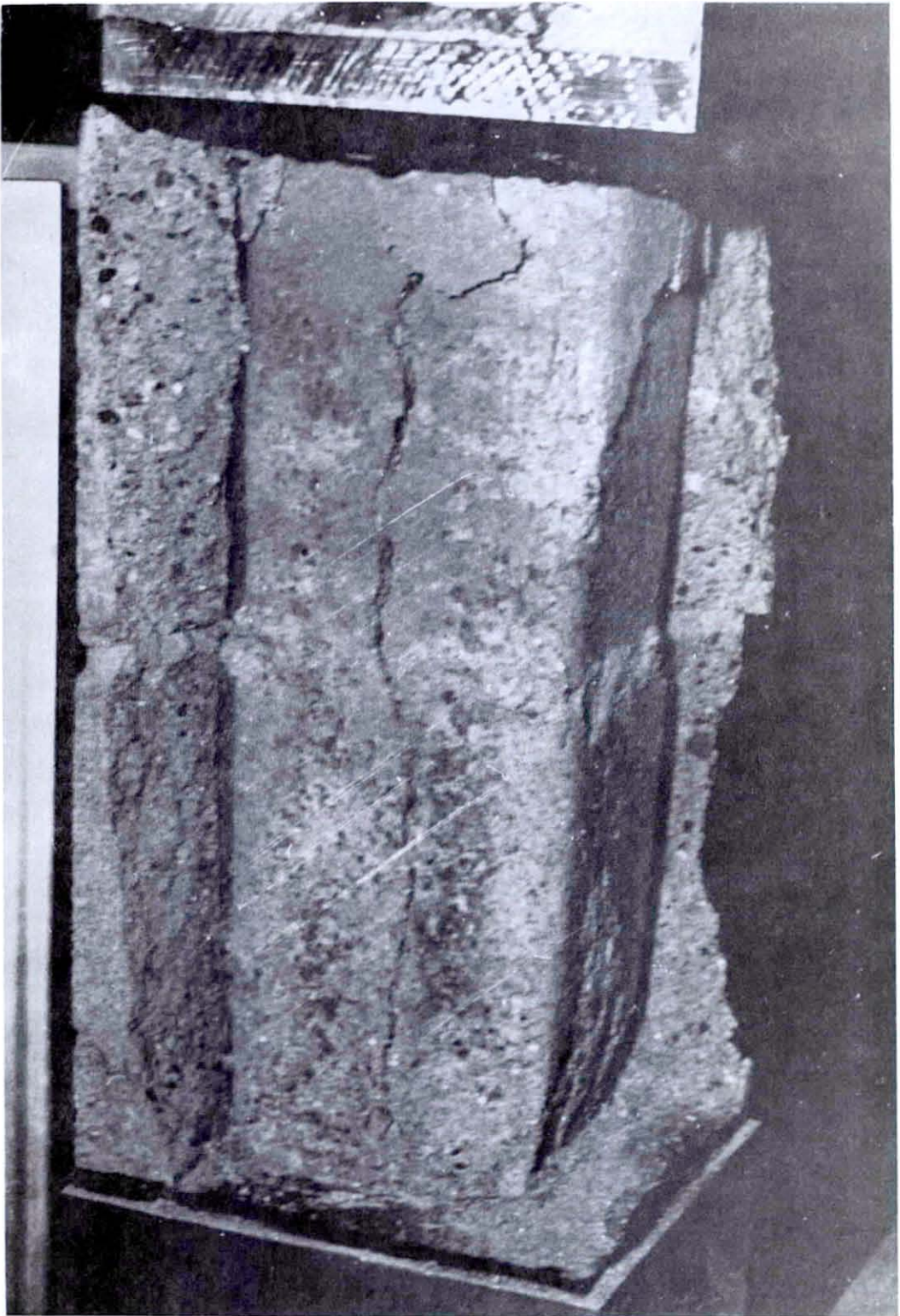
Fig. 3.3. Tensile Splitting of Two-Course Prism with Soft Cap
