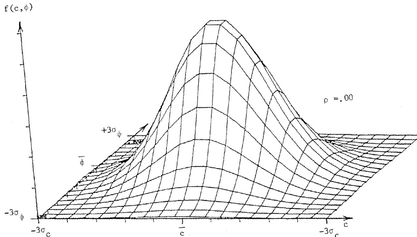
FIGURE 3-7. BIVARIATE NORMAL DISTRIBUTION FOR STRENGTH PARAMETERS OF ILLUSTRATIVE EXAMPLE
