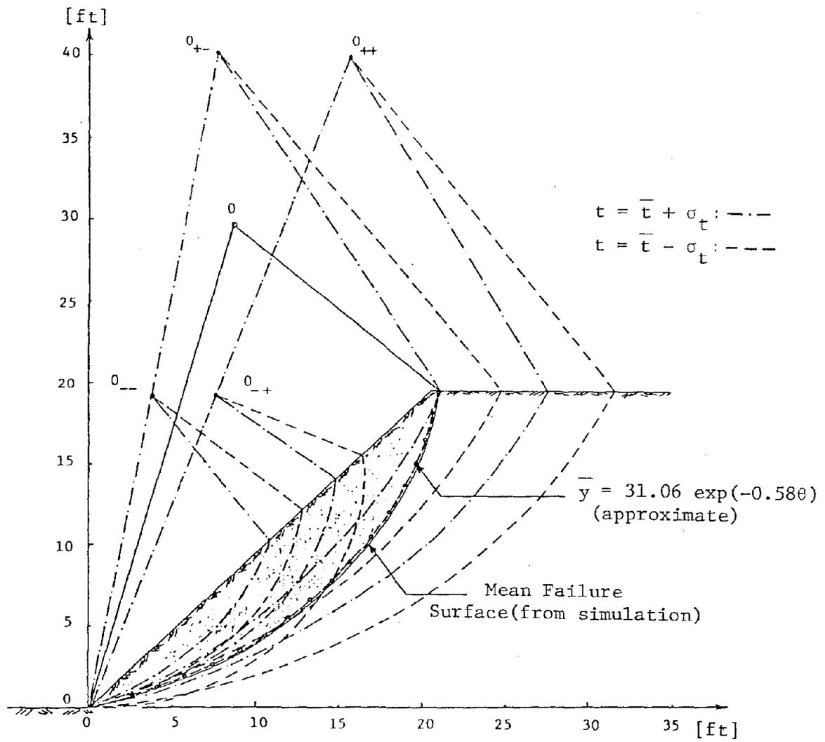
FIGURE 2-3. MEAN FAILURE SURFACE: AN EXAMPLE
