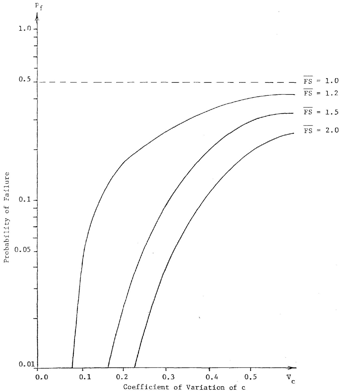
FIGURE 4-3. EFFECT OF  $V_c$  ON  $p_f$ , UNDRAINED ANALYSIS ( $\beta = 30^\circ$ )
