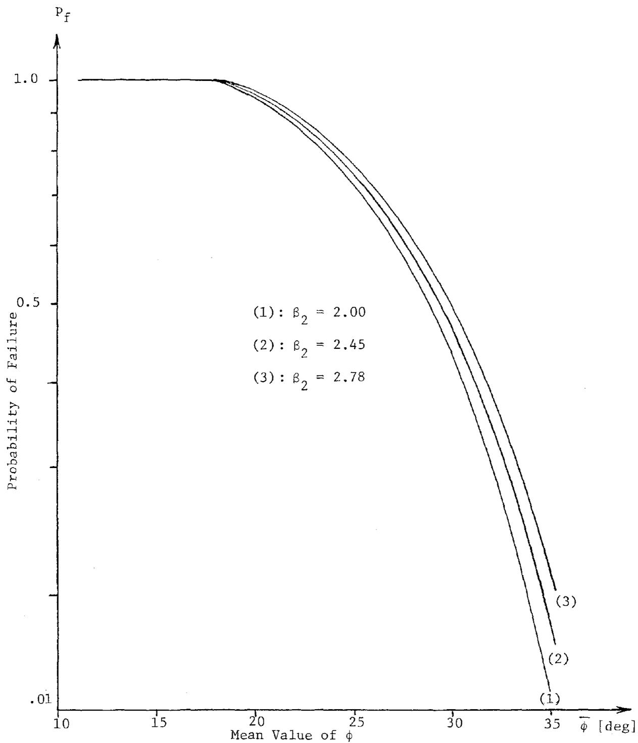
FIGURE 4-8. EFFECT ON PROBABILITY OF FAILURE OF COEFFICIENT OF KURTOSIS OF  $\phi$ -PARAMETER
