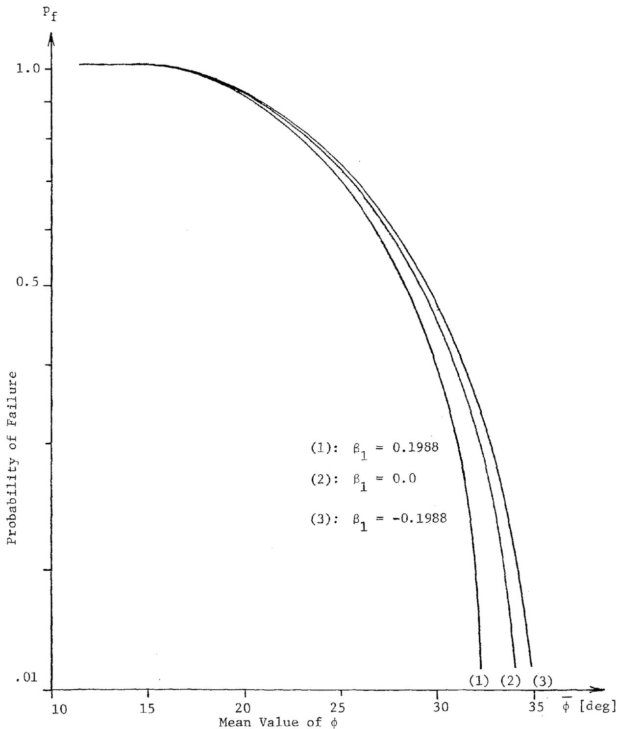
FIGURE 4-6. EFFECT ON PROBABILITY OF FAILURE OF COEFFICIENT OF SKEWNESS OF  $\phi$ -PARAMETER
