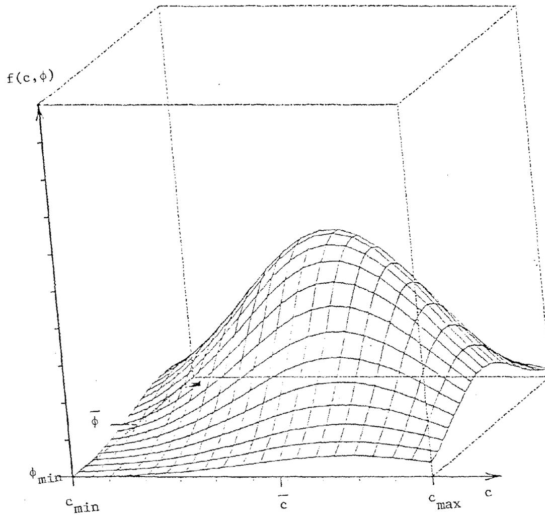
FIGURE 3-4. TRUNCATED BIVARIATE NORMAL DISTRIBUTION FOR STRENGTH PARAMETERS OF ILLUSTRATIVE EXAMPLE ( $\rho = -0.325$ )
