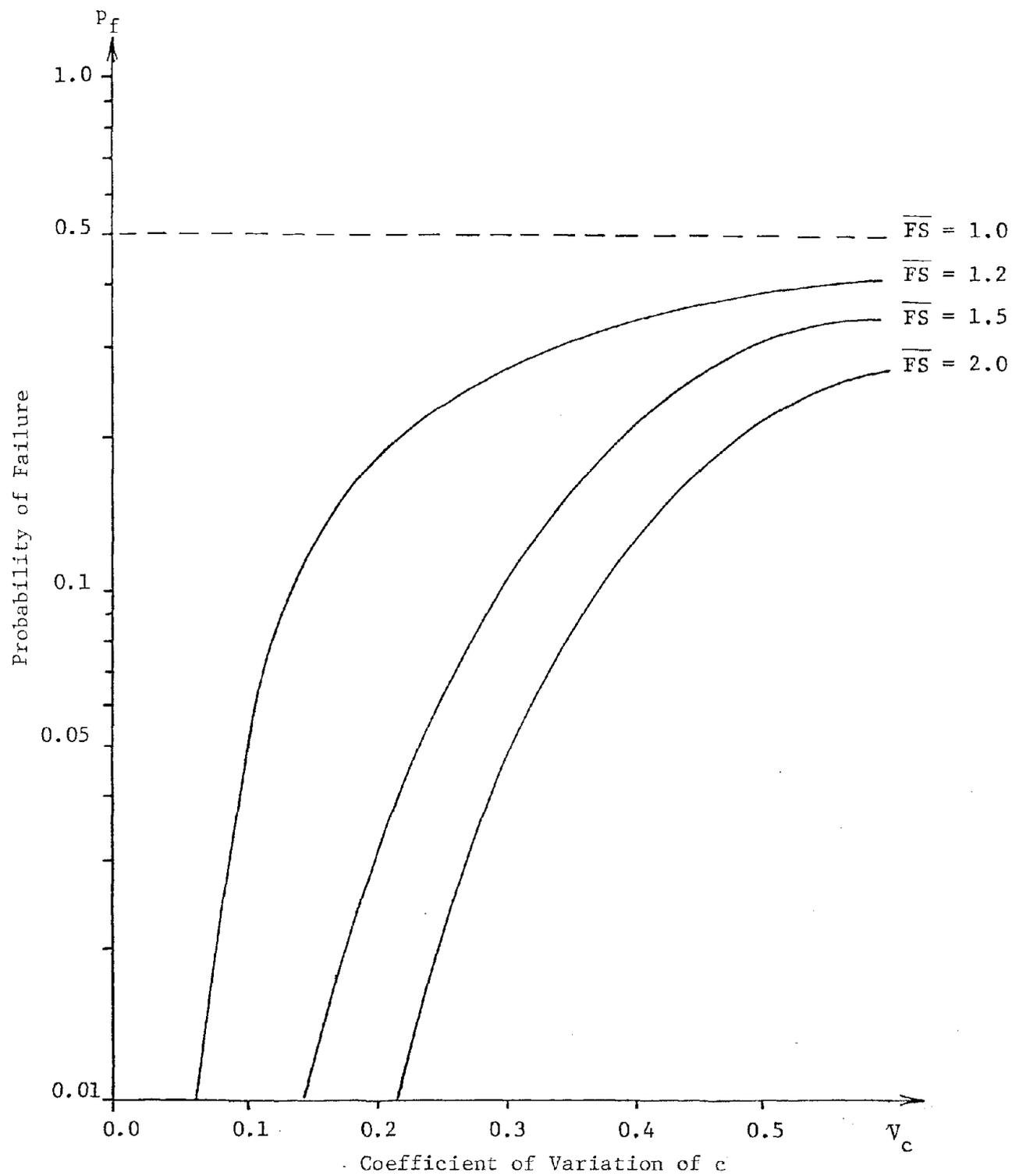
FIGURE 4-4. EFFECT OF  $V_c$  ON  $P_f$ , UNDRAINED ANALYSIS ( $\beta = 60^\circ$ )
