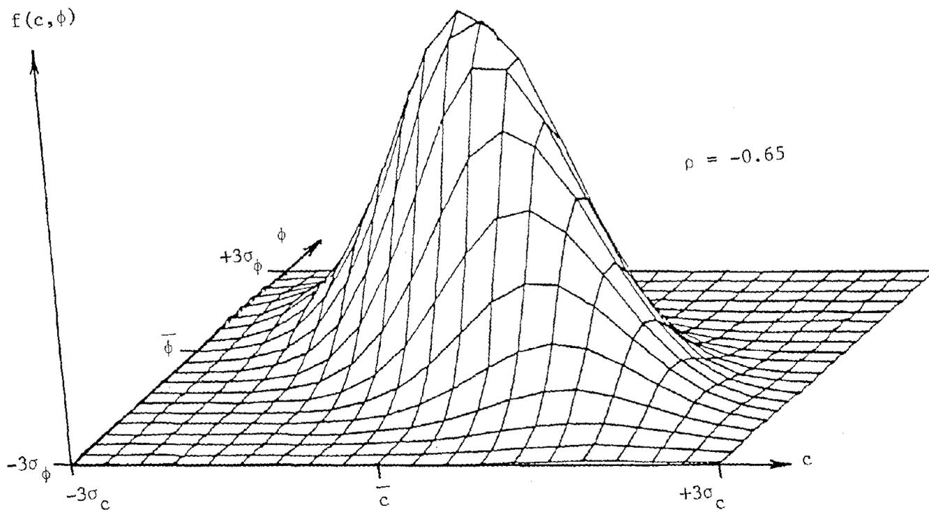
FIGURE 3-6. BIVARIATE NORMAL DISTRIBUTION FOR STRENGTH PARAMETERS OF ILLUSTRATIVE EXAMPLE
