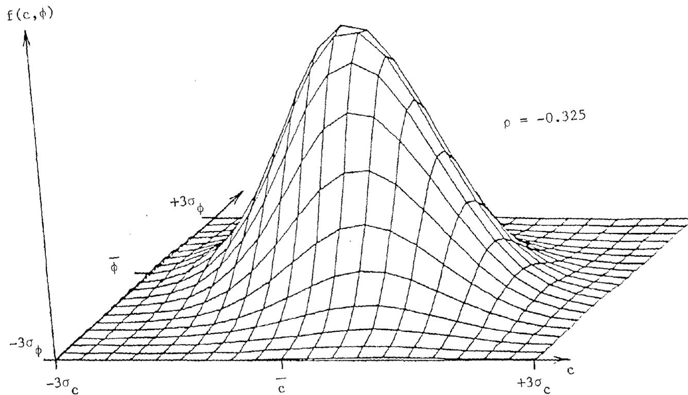
FIGURE 3-3. BIVARIATE NORMAL DISTRIBUTION FOR STRENGTH PARAMETERS OF ILLUSTRATIVE EXAMPLE
