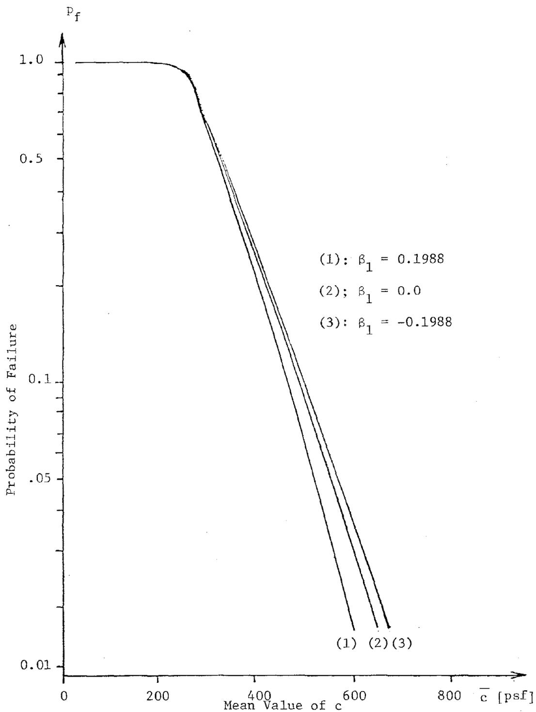
FIGURE 4-5. EFFECT ON THE PROBABILITY OF FAILURE OF COEFFICIENT OF SKEWNESS OF  $c$ -PARAMETER
