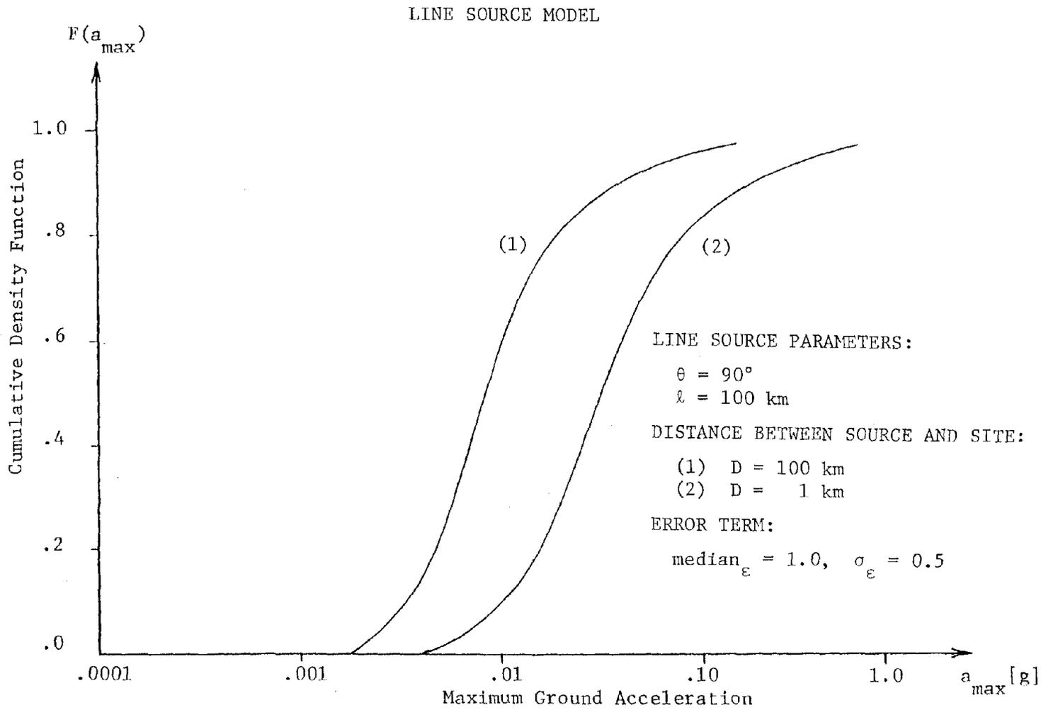
FIGURE 5-12. CUMULATIVE FUNCTION OF GROUND ACCELERATION
