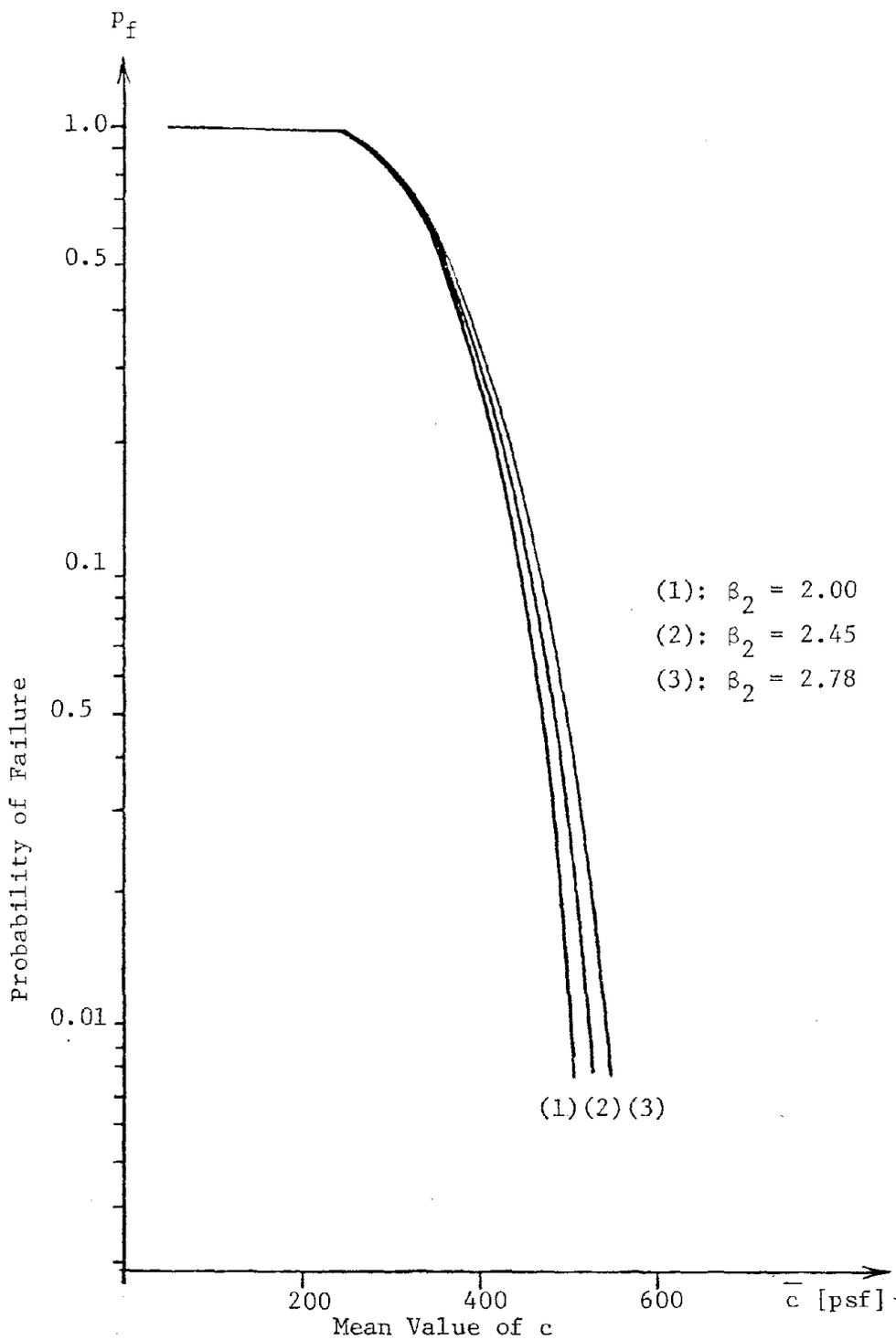
FIGURE 4-7. EFFECT ON PROBABILITY OF FAILURE OF COEFFICIENT OF KURTOSIS OF  $c$ -PARAMETER
