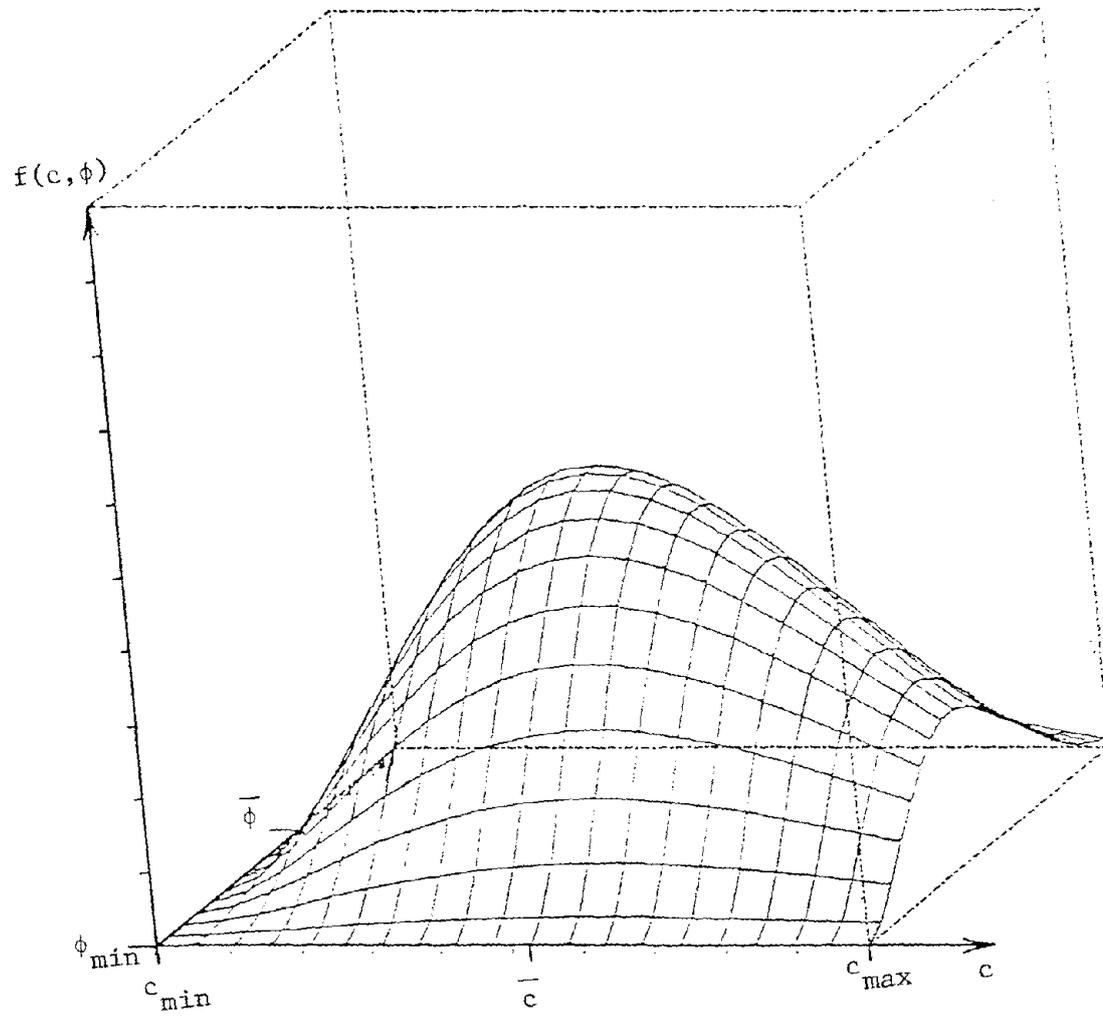
FIGURE 3-9. TRUNCATED BIVARIATE BETA DISTRIBUTION FOR STRENGTH PARAMETERS OF ILLUSTRATIVE EXAMPLE ( $\rho = -0.325$ )
