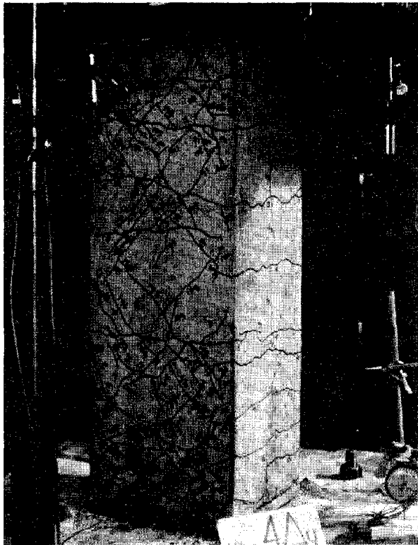
Appearance of specimen after testing
