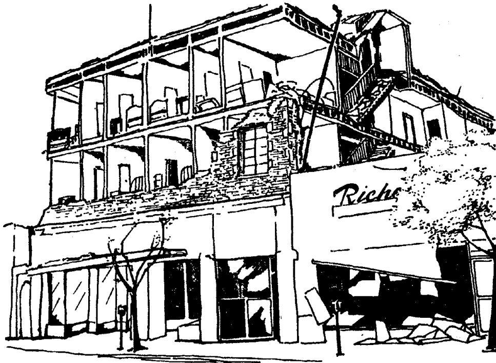
NONSTRUCTURAL WALLS FUNCTIONING AS SHEAR WALLS
