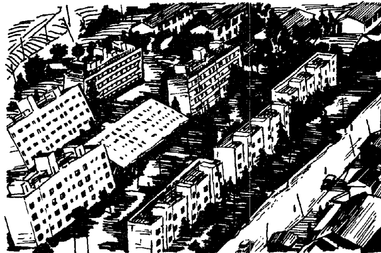
LIQUIFACTION - 1964 NIIGATA, JAPAN EARTHQUAKE Figure 3.14
