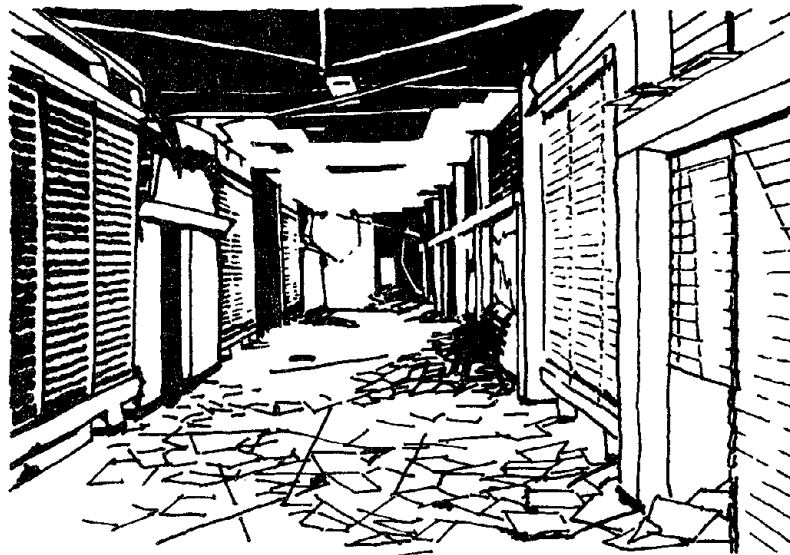
CEILING COLLAPSE SUPREME COURT - 1972 MANAGUA EARTHQUAKE Figure 14.14
