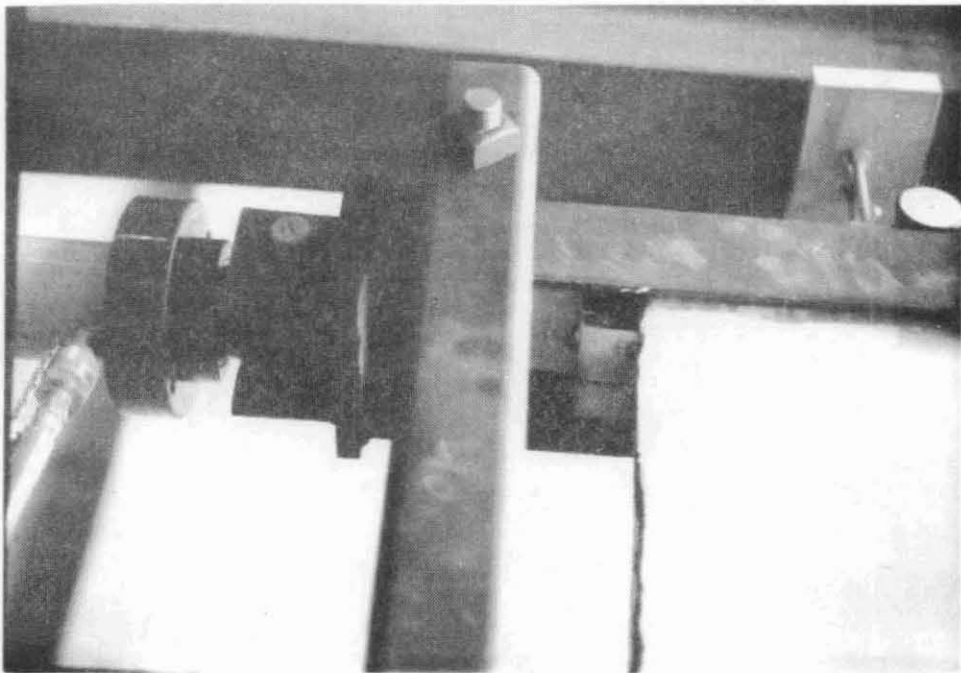
Fig. 45: Partition Test Specimen P2: Slippage @ Top Runner
