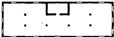
Figure IV-28. Wall length/floor area ratio quickly reveals different load/capacity factors of two buildings which both meet minimum code requirements.
