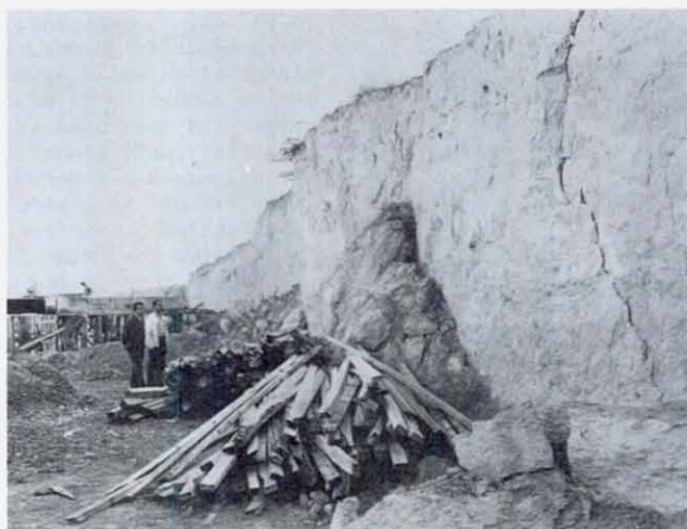
FIGURE 59 This 20-foot high bank of lacustrine clay with thin gravel lenses at a construction site on the west side of Burdur, undercut in some places, has stood for nine months with only small falls of earth. Soil everywhere observed in the Burdur region was firm, and no damage was attributed to soil failure.
