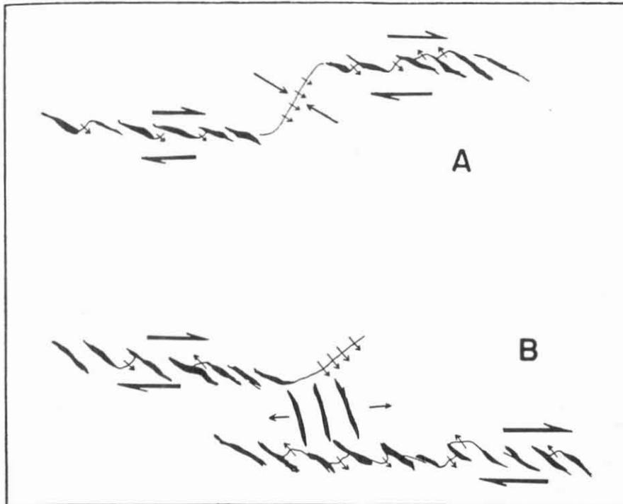
19. Schematic Description of Local Ground Deformation
