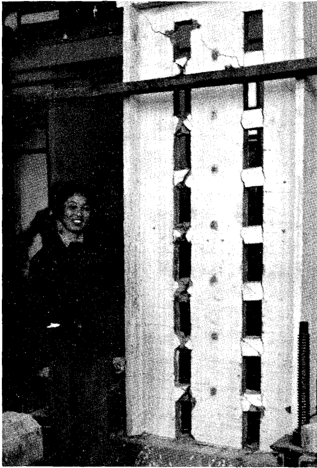
Figure 4.3 Model of coupled shear wall at the Academy of Building Research, Beijing.
