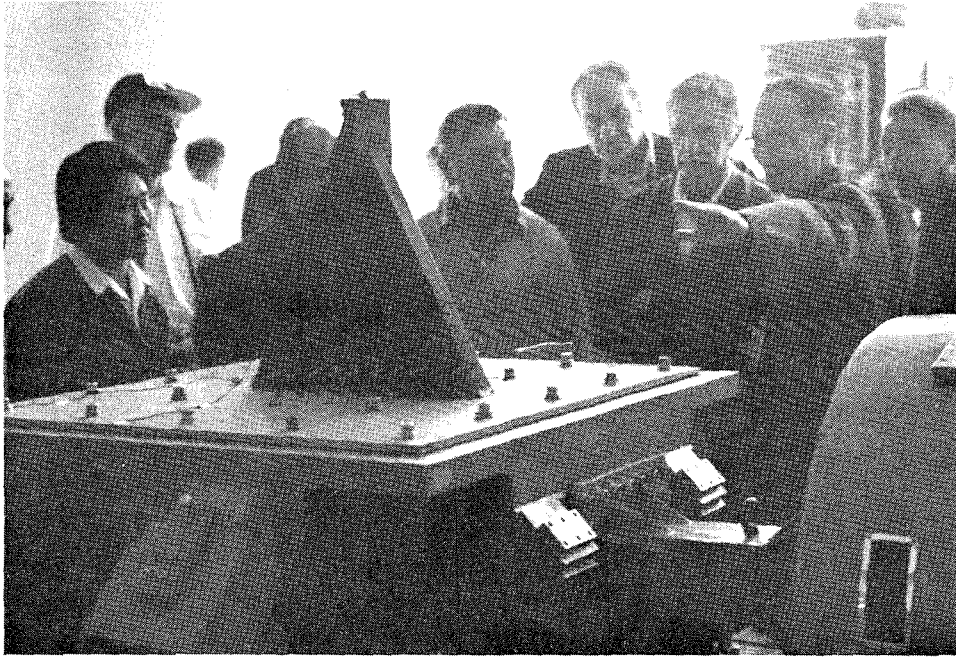
Figure 4.7 Section of concrete gravity dam on shake table.
