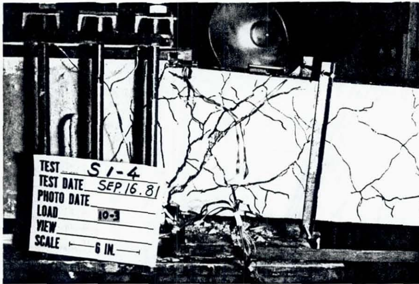
Fig. 3.14 Specimen S1-4 at the Maximum Positive Displacement of Tenth Load Cycle
